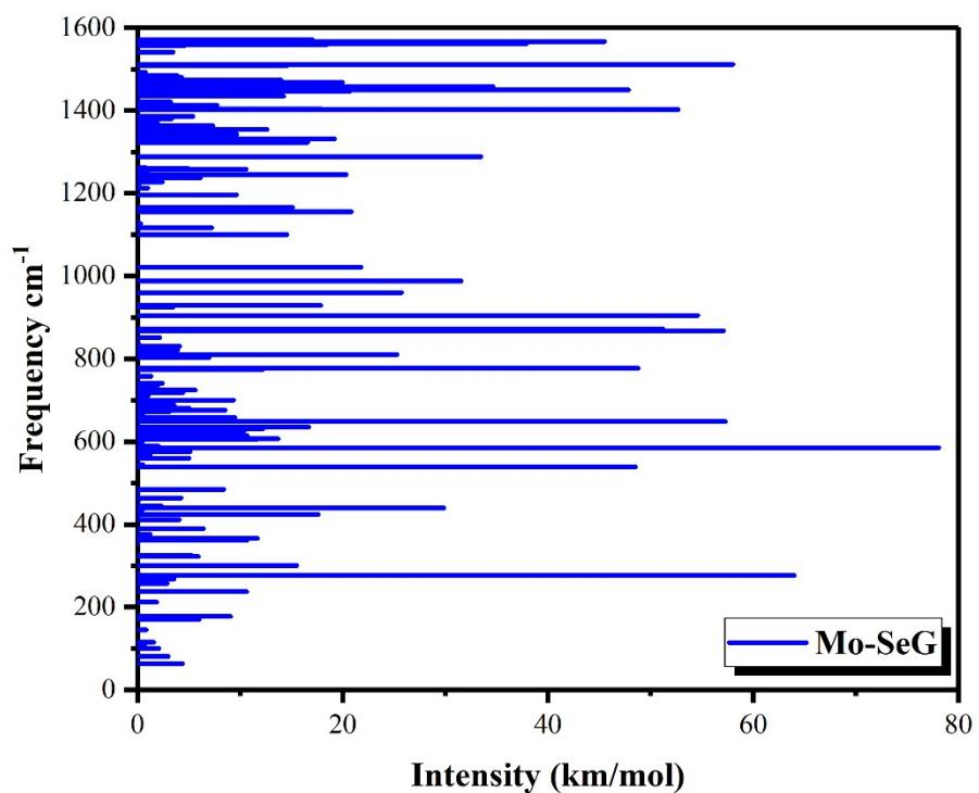
**Figure S1.** Frequency distribution of geometrically optimized Mo/SeG.
