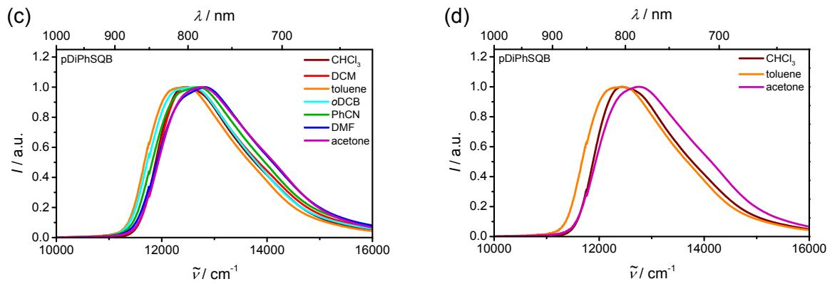
**Fig. S4.** (a)(b) Complete and (c) normalised absorption spectra of **[TP-SQB]<sub>n</sub>** in various solvents. (d) Normalised absorption spectra of **[TP-SQB]<sub>n</sub>** in CHCl<sub>3</sub>, toluene, and acetone.
