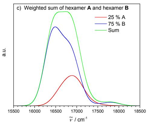
**Fig. S2.** Simulated absorption spectra of  $[\text{TP-SQB}]_6$  based on the CNDO S2 results from Table S1 convoluted with Gaussian function with an estimated half width of  $400 \text{ cm}^{-1}$  for hexamer **A** (a), hexamer **B** (b) and the weighted sum of both structure **A** and **B** (c).
