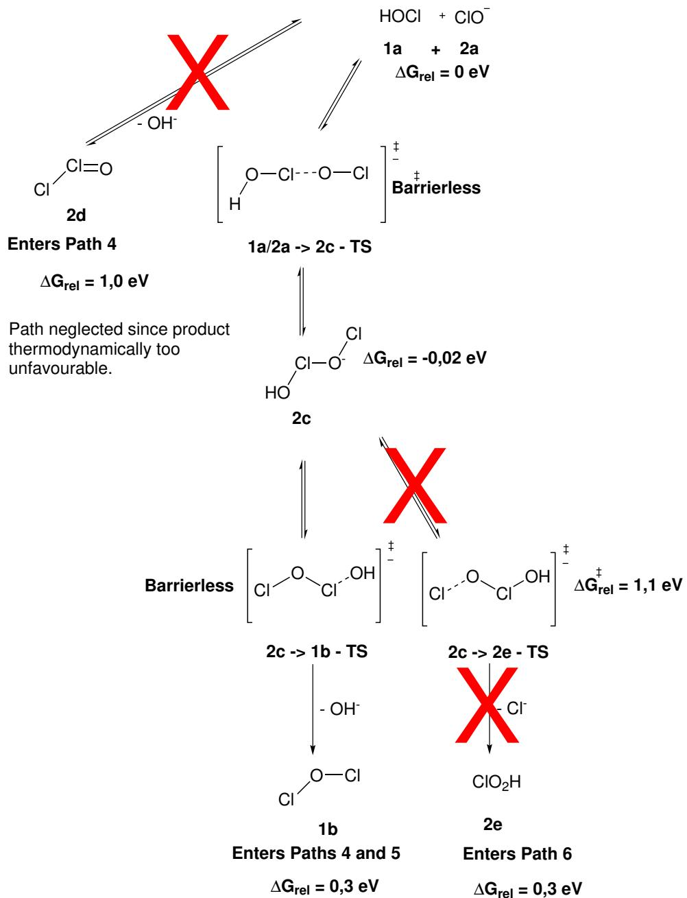
**Path3 - High pH (potentially direct formation of chlorite!)**
