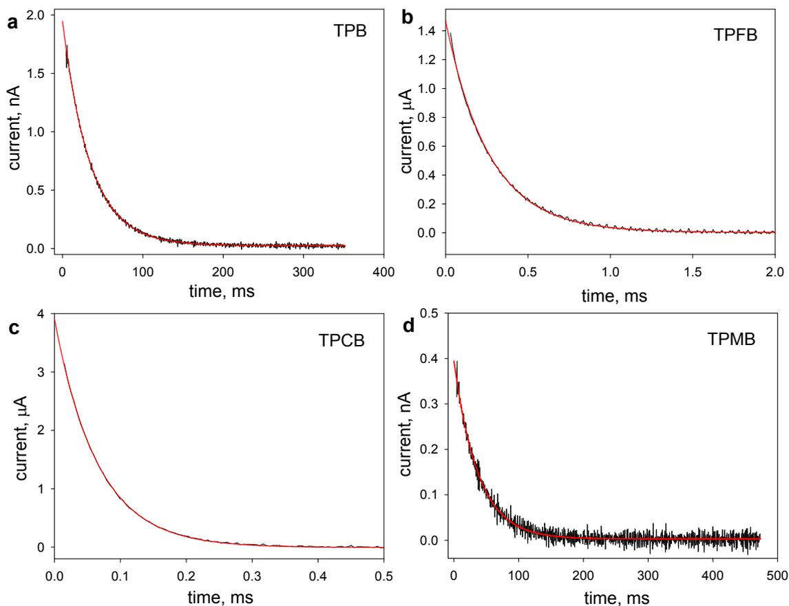
**Figure S2.** Time courses of electrical current through planar BLMs after application of a voltage jump from 0 mV to 25 mV (black curves) and their best fit by a monoexponential function (red curves) in the presence of 0.1  $\mu$ M TPB (a,  $\tau = 34.5$  ms), 0.1  $\mu$ M TPFB (b,  $\tau = 265$   $\mu$ s), 0.1  $\mu$ M TPCB (c,  $\tau = 65.5$   $\mu$ s) and 0.2  $\mu$ M TPMB (d,  $\tau = 37.5$  ms).
