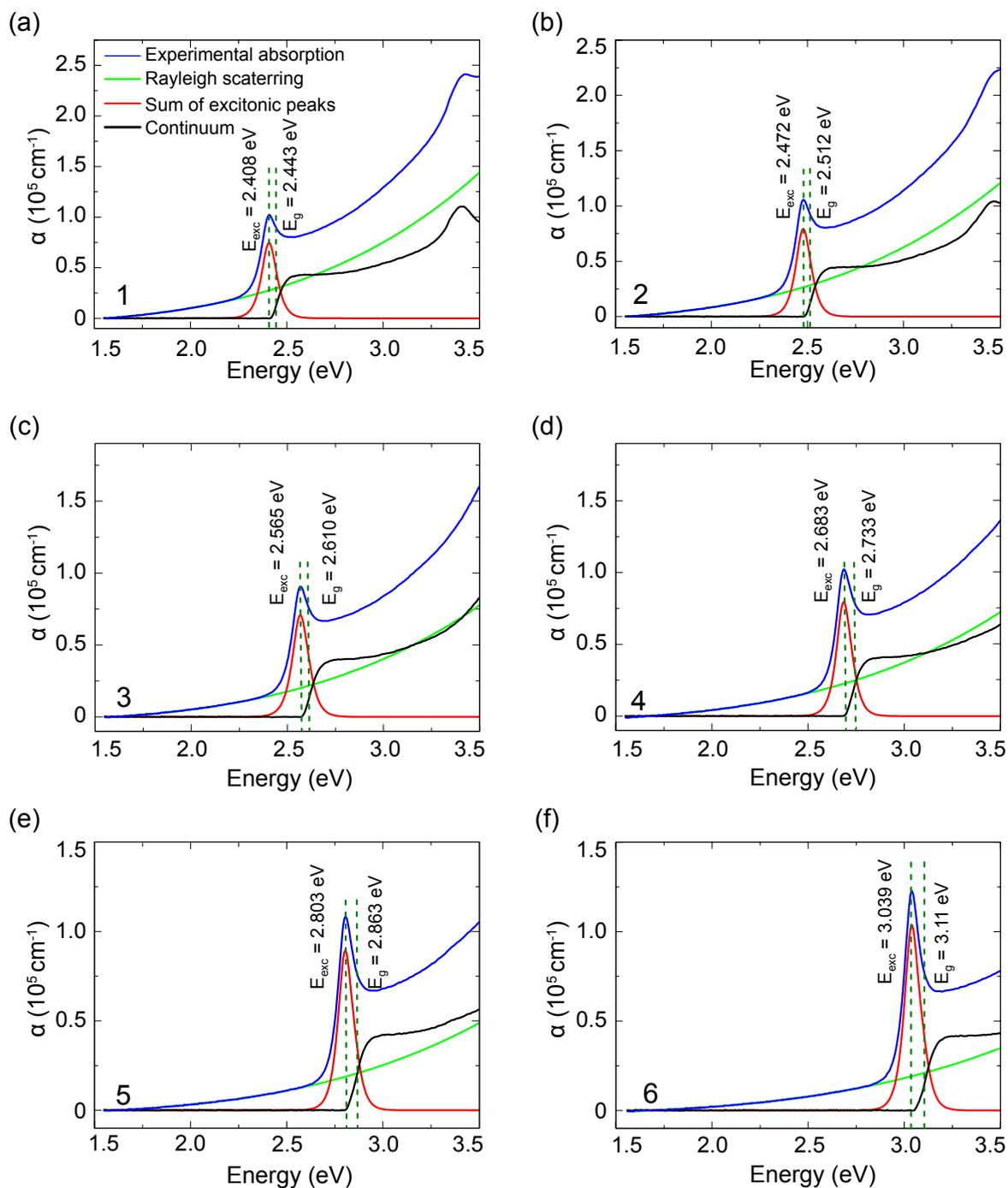
Figure S 3: Spectral deconvolution of the experimental extinction of 1-6. Continuum stands for band-to-band electronic absorption.
