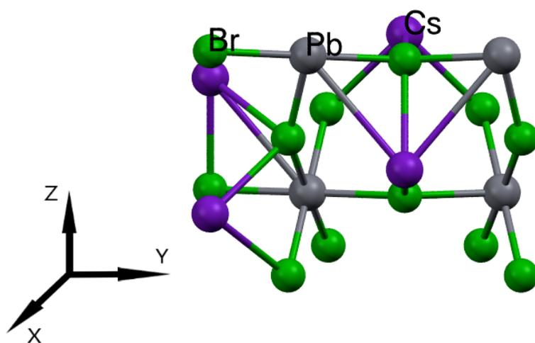
Figure S 4: The example of the orthorhombic unit cell (Pnma) used in the ab-initio calculations. The atomic coordinates are presented in the Table S2
