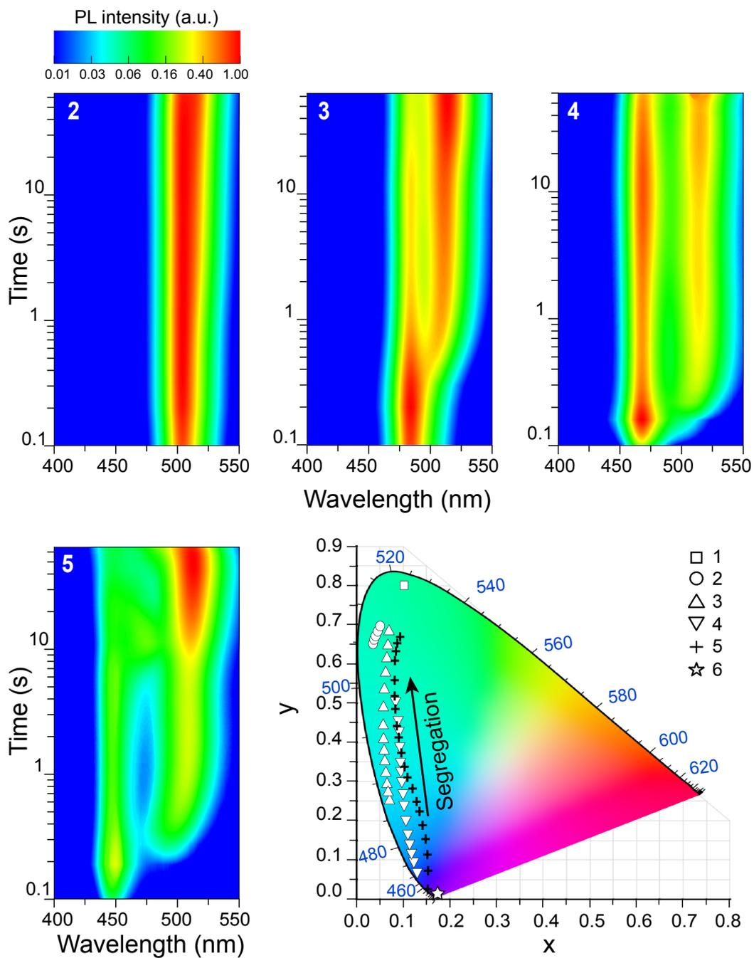
Figure S 1: PL dynamics caused by light-induced halide ion segregation in mixed-halide perovskite thin films and its representation in CIE 1931 color space.
