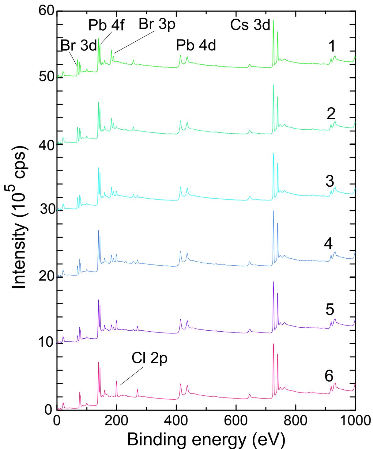
Figure S 2: Survey scan XPS spectra for 1-6
