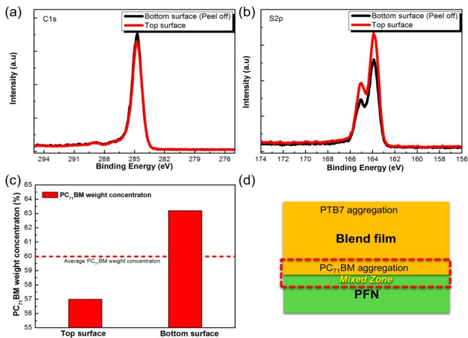
Figure S4. XPS spectra of (a) C1s and (b) S2p of PTB7:PC<sub>71</sub>BM blend film at top and bottom surfaces. (c) The PC<sub>71</sub>BM weight concentration in the blend film at top and bottom surfaces. (d) Schematic illustration for distribution of PTB7 and PC<sub>71</sub>BM in the blend film.
