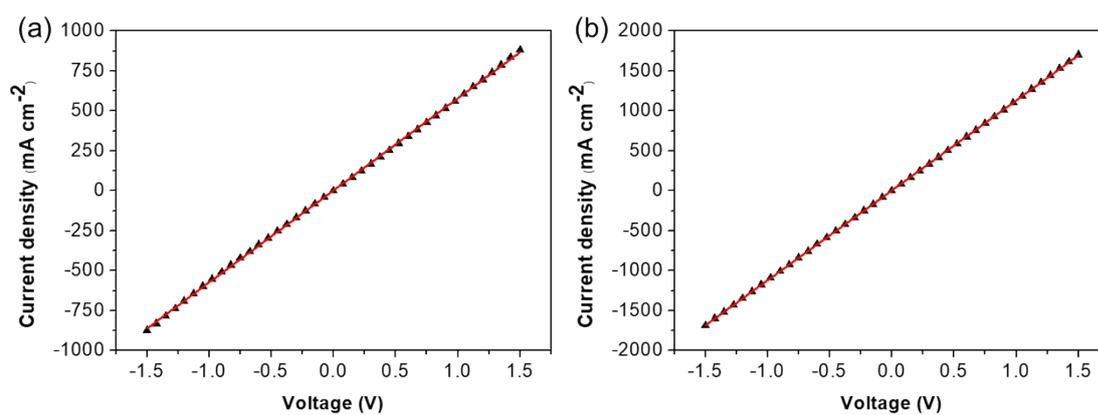
Figure S3. Conductivity measurements of PC<sub>71</sub>BM in (a) ITO/PC<sub>71</sub>BM(20nm)/PFN(2nm)/Al and (b) ITO/PFN(2nm)/PC<sub>71</sub>BM(20nm)/Al.
