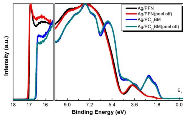
Figure S2. UPS spectra of PFN and PC<sub>71</sub>BM films prepared by spin-coating method and “Peel-off” method on Ag.
