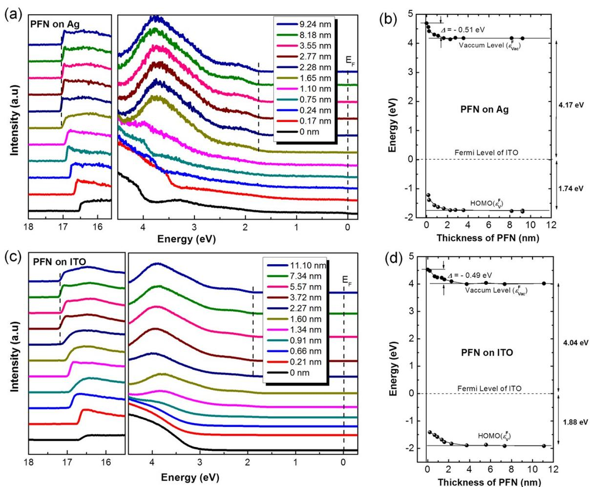
Figure S1. UPS spectra of various thickness PFN layer spin-coated on Ag (a) and ITO (c). Evolution of the WF and HOMO with the variation in thickness of PFN on Ag (b) and ITO (d).
