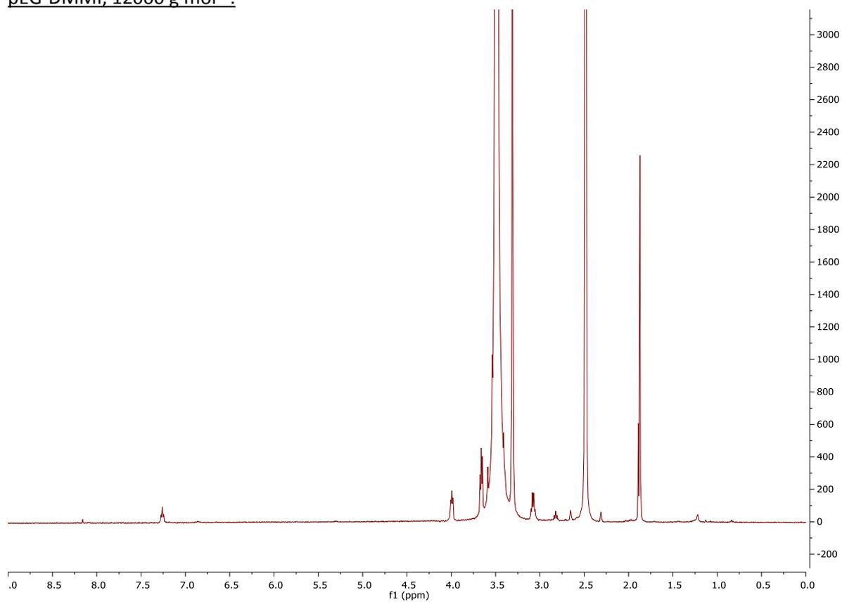
**Figure 30.** Full <sup>1</sup>H-NMR spectrum of pEG-DMMI, 12000 g·mol<sup>-1</sup>. The solvent is DMSO-d<sub>6</sub>.
