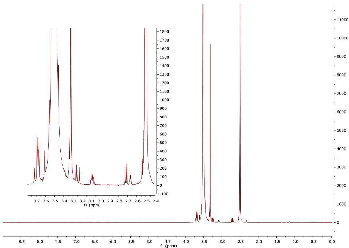
**Figure 6.** Full  $^1\text{H-NMR}$  spectrum of pEG-epoxide,  $12000\text{ g}\cdot\text{mol}^{-1}$ . The solvent is  $\text{DMSO-d}_6$ .
