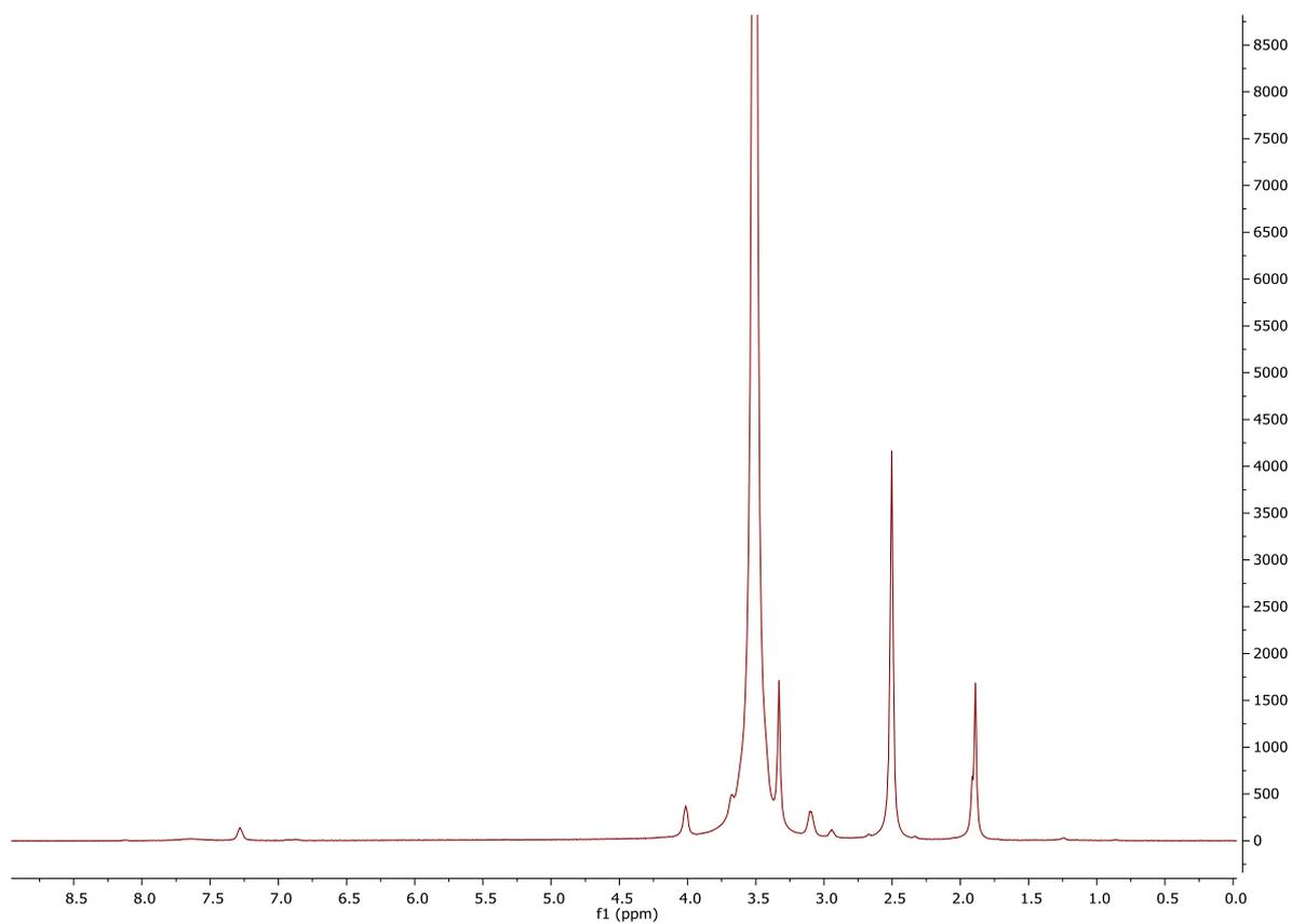
**Figure 26.** Full  $^1\text{H}$ -NMR spectrum of pEG-DMMI,  $4000\text{ g}\cdot\text{mol}^{-1}$ . The solvent is  $\text{DMSO-d}_6$ .
