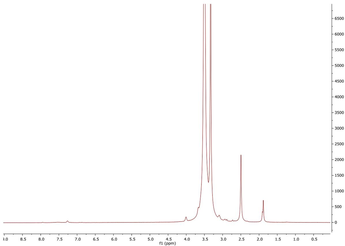
**Figure 28.** Full <sup>1</sup>H-NMR spectrum of pEG-DMMI, 8000 g·mol<sup>-1</sup>. The solvent is DMSO-d<sub>6</sub>.
