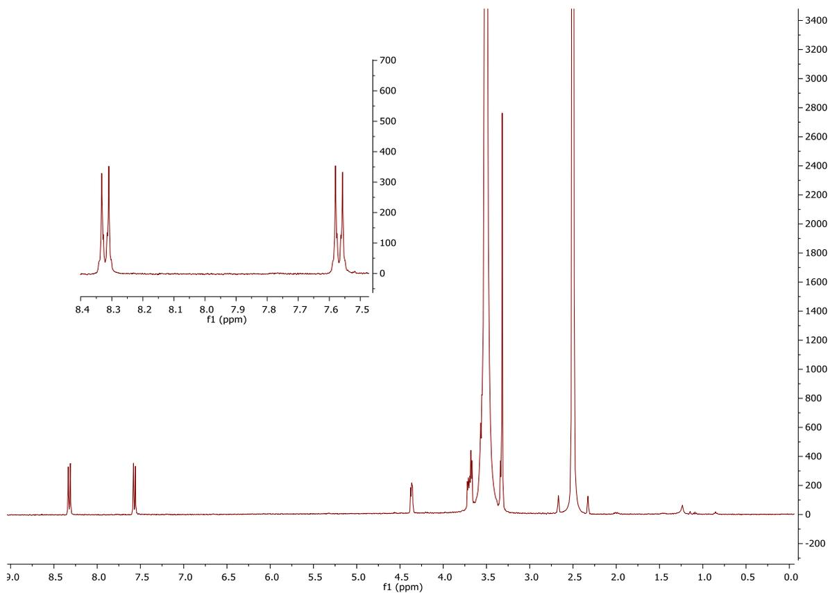
**Figure 25.** Full <sup>1</sup>H-NMR spectrum of pEG-p-nitrophenylcarbonate, 12000 g·mol<sup>-1</sup>. The solvent is DMSO-d<sub>6</sub>.
