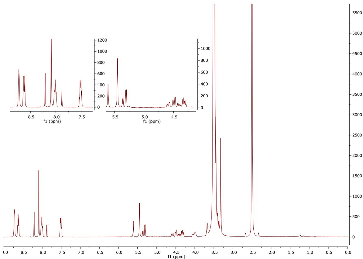
**Figure 13.** Full  $^1\text{H-NMR}$  spectrum of pEG-hydroxy-terpyridine,  $4000 \text{ g}\cdot\text{mol}^{-1}$ . The solvent is  $\text{DMSO-d}_6$ .
