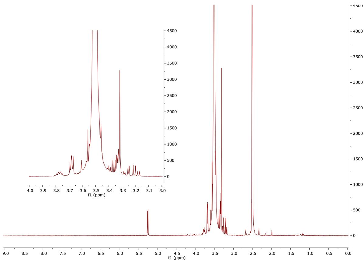
**Figure 10.** Full  $^1\text{H}$ -NMR spectrum of pEG-hydroxy-azide,  $10000 \text{ g}\cdot\text{mol}^{-1}$ . The solvent is  $\text{DMSO-d}_6$ .
