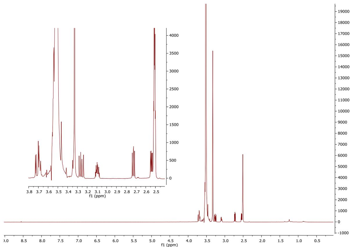
**Figure 2.** Full <sup>1</sup>H-NMR spectrum of pEG-epoxide, 4000 g·mol<sup>-1</sup>. The solvent is DMSO-d<sub>6</sub>.
