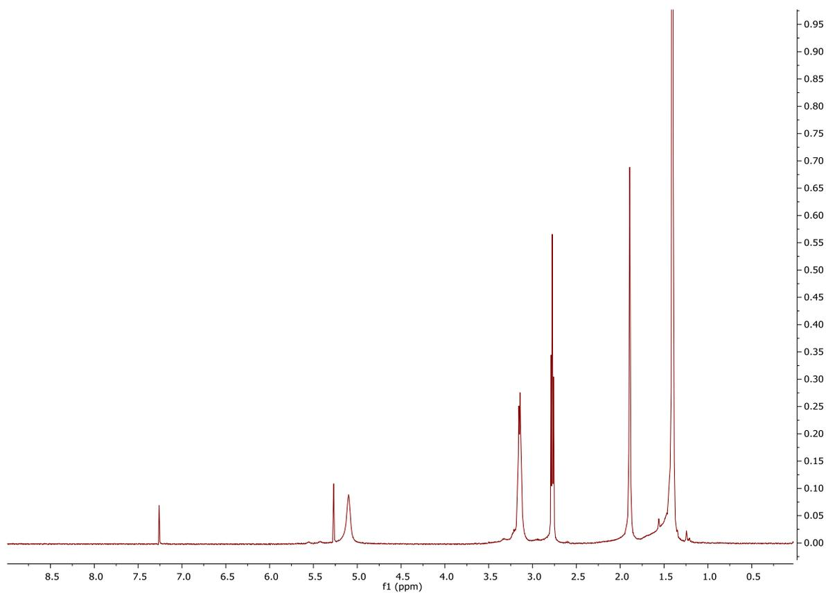
**Figure 18.** Full  $^1\text{H}$ -NMR spectrum of *Tert*-butyl (2-aminoethyl)carbamate. The solvent is  $\text{CDCl}_3$ .
