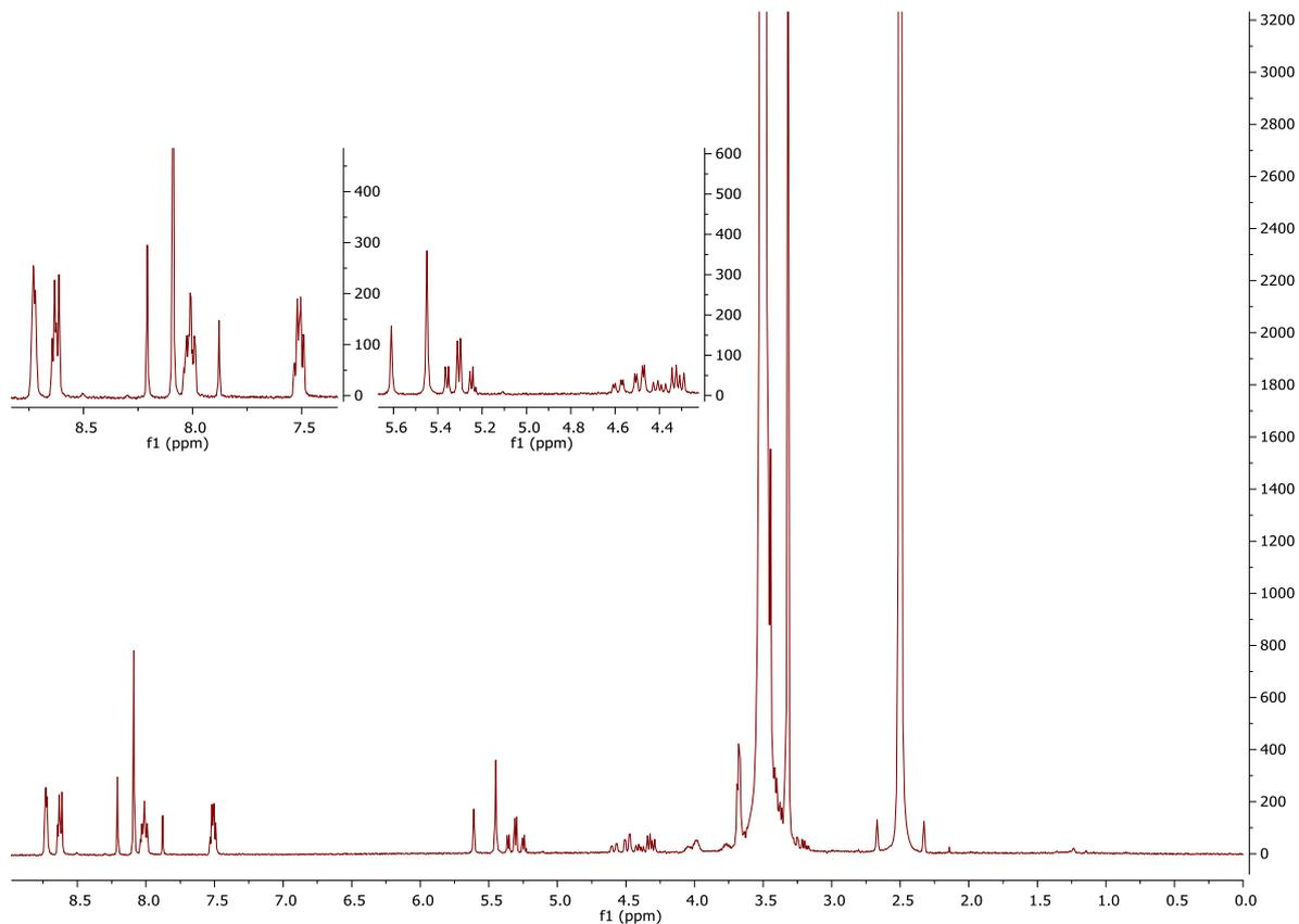
**Figure 16.** Full  $^1\text{H}$ -NMR spectrum of pEG-hydroxy-terpyridine,  $10000 \text{ g}\cdot\text{mol}^{-1}$ . The solvent is  $\text{DMSO-d}_6$ .
