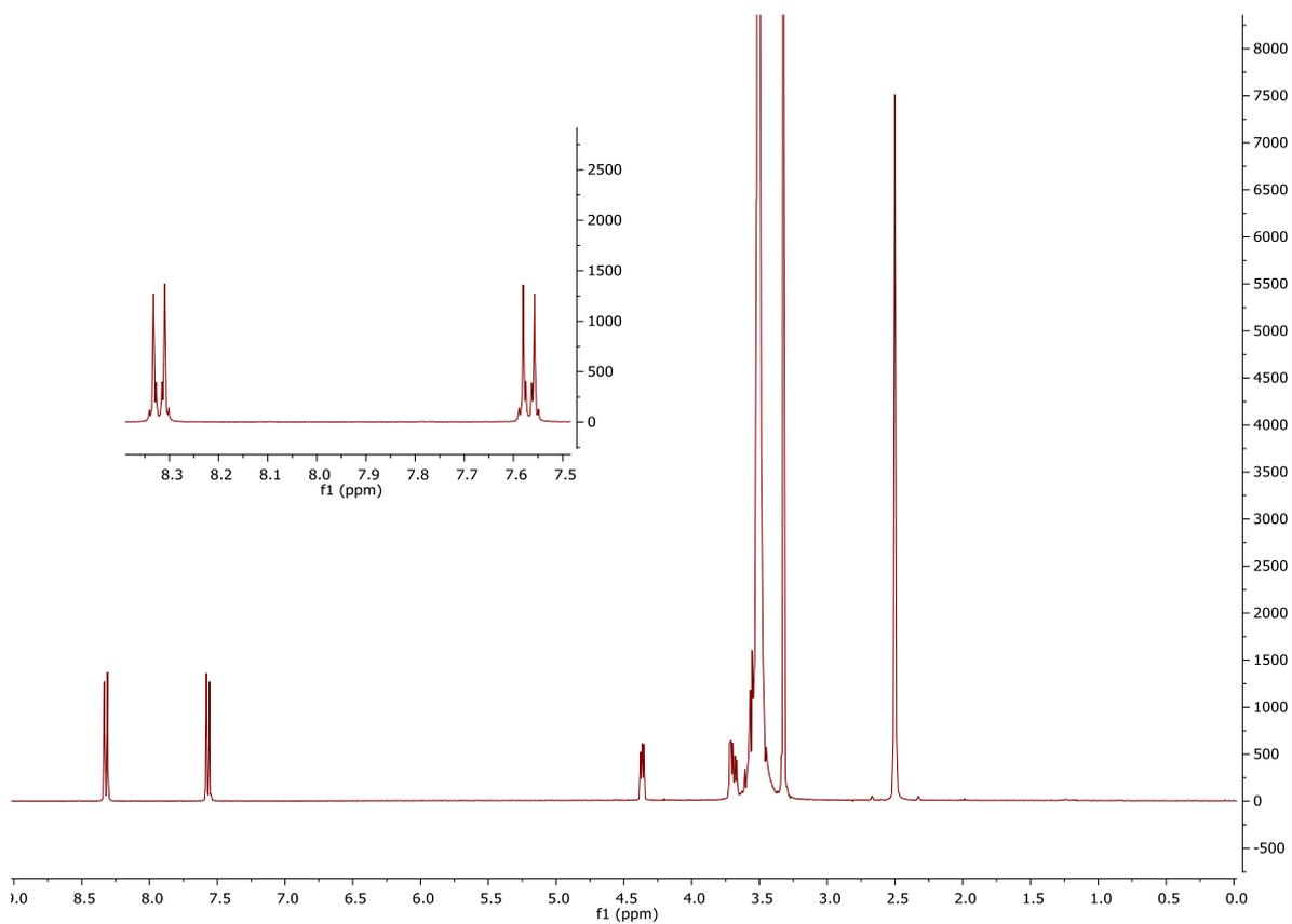
**Figure 22.** Full  $^1\text{H-NMR}$  spectrum of pEG-*p*-nitrophenylcarbonate,  $6000\text{ g}\cdot\text{mol}^{-1}$ . The solvent is  $\text{DMSO-d}_6$ .
