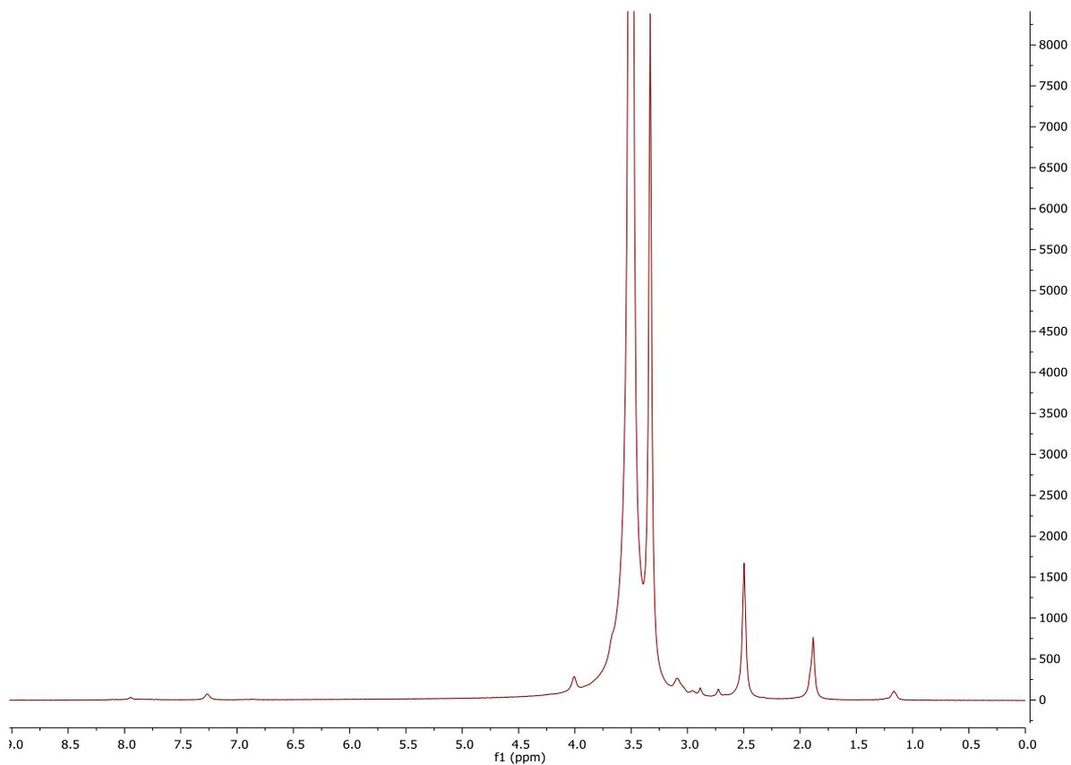
**Figure 27.** Full  $^1\text{H}$ -NMR spectrum of pEG-DMMI,  $6000\text{ g}\cdot\text{mol}^{-1}$ . The solvent is  $\text{DMSO-d}_6$ .
