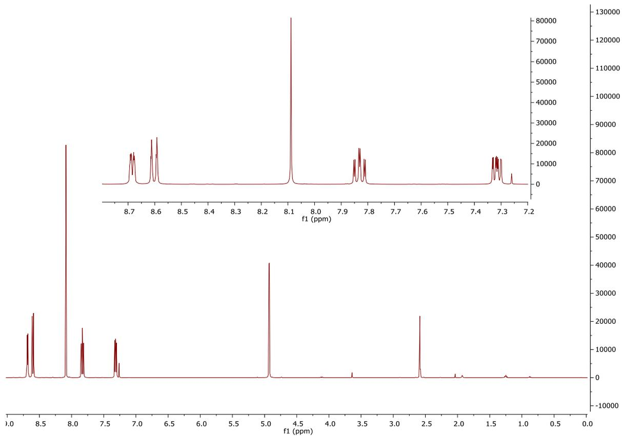
**Figure 12.** Full  $^1\text{H-NMR}$  spectrum of propargyl-terpyridine. The solvent is  $\text{CDCl}_3$ .
