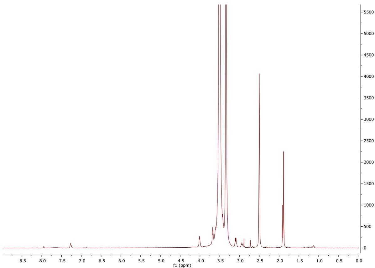
**Figure 29.** Full <sup>1</sup>H-NMR spectrum of pEG-DMMI, 10000 g·mol<sup>-1</sup>. The solvent is DMSO-d<sub>6</sub>.
