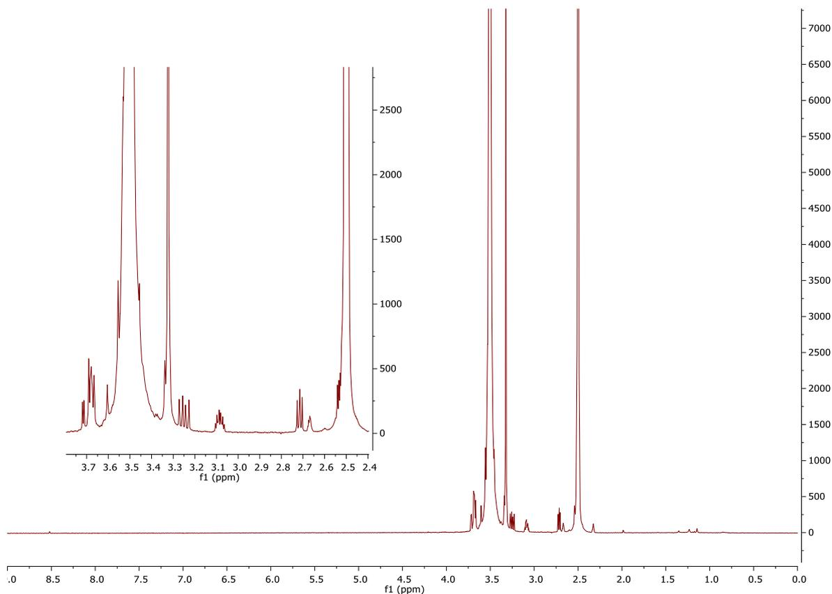
**Figure 5.** Full  $^1\text{H-NMR}$  spectrum of pEG-epoxide,  $10000\text{ g}\cdot\text{mol}^{-1}$ . The solvent is  $\text{DMSO-d}_6$ .
