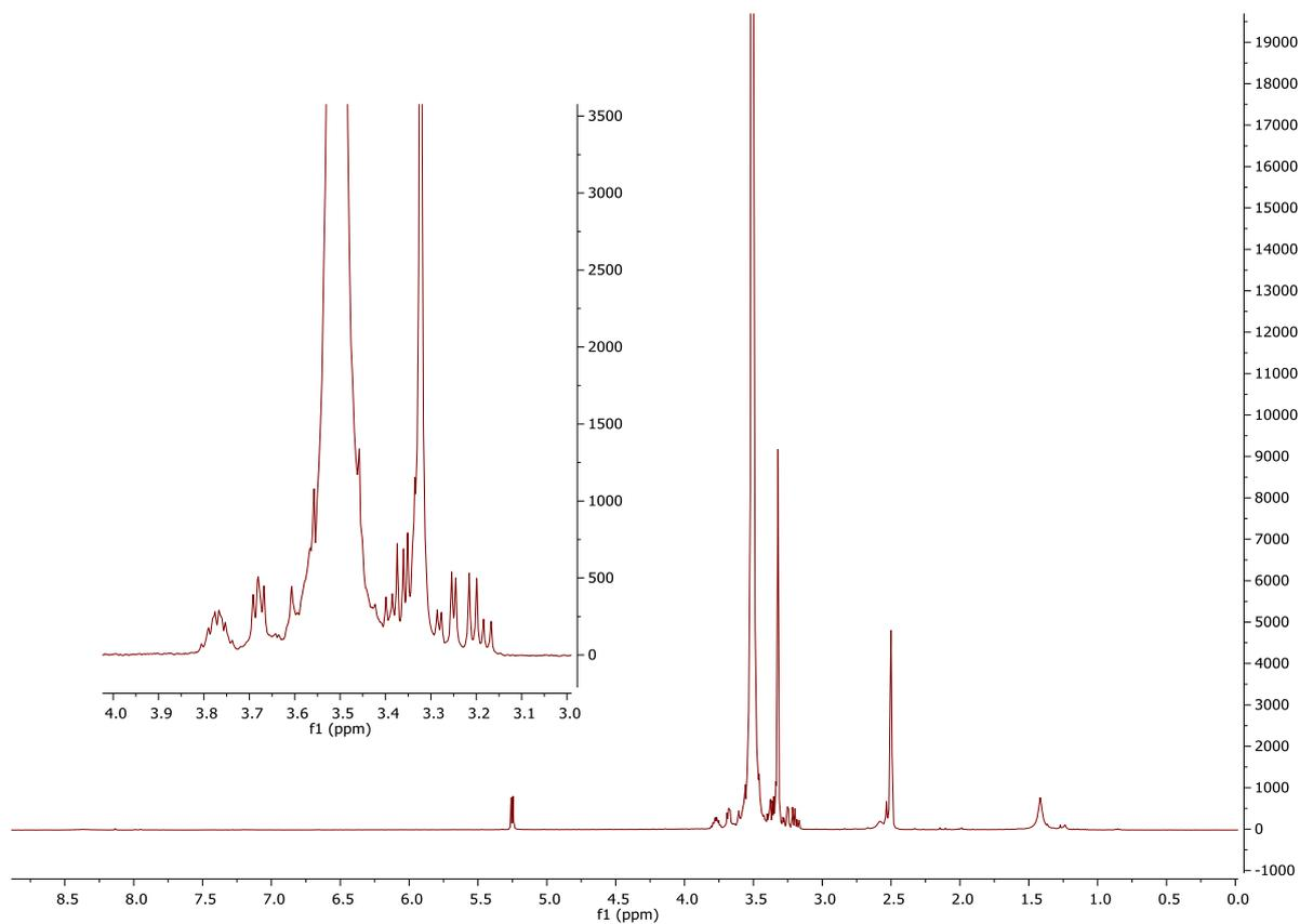
**Figure 7.** Full  $^1\text{H-NMR}$  spectrum of pEG-hydroxy-azide,  $4000\text{ g}\cdot\text{mol}^{-1}$ . The solvent is  $\text{DMSO-d}_6$ .
