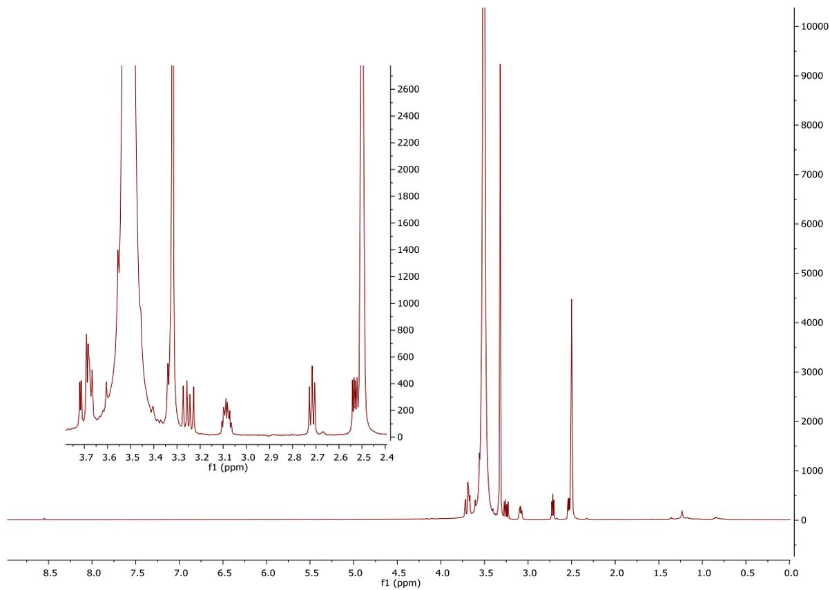
**Figure 3.** Full <sup>1</sup>H-NMR spectrum of pEG-epoxide, 6000 g·mol<sup>-1</sup>. The solvent is DMSO-d<sub>6</sub>.
