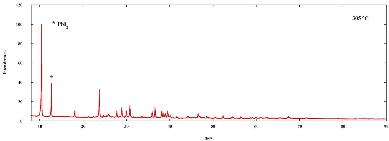
Fig. S5. X-ray powder diffraction pattern of  $\text{N}(\text{CH}_3)_4\text{PbI}_3$  after isothermal treatment at 305 °C for 10 hours.
