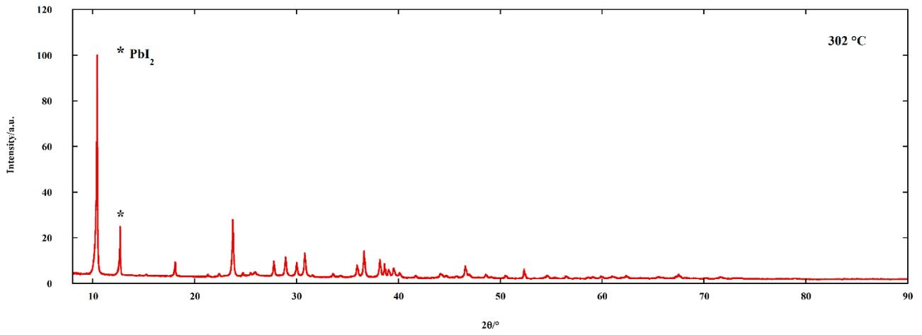
Fig. S4. X-ray powder diffraction pattern of  $\text{N}(\text{CH}_3)_4\text{PbI}_3$  after isothermal treatment at 302 °C for 10 hours.
