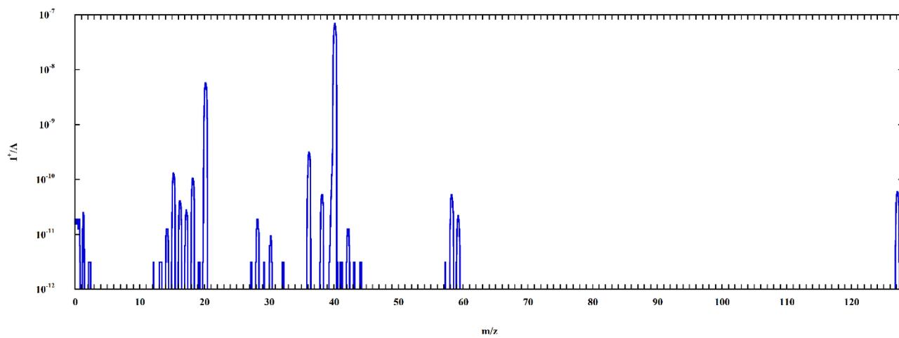
Fig. S9. Mass spectrum acquired in correspondence of the maximum ion currents due to evolved gases in the TG-DTA/QMS-EGA experiment.
