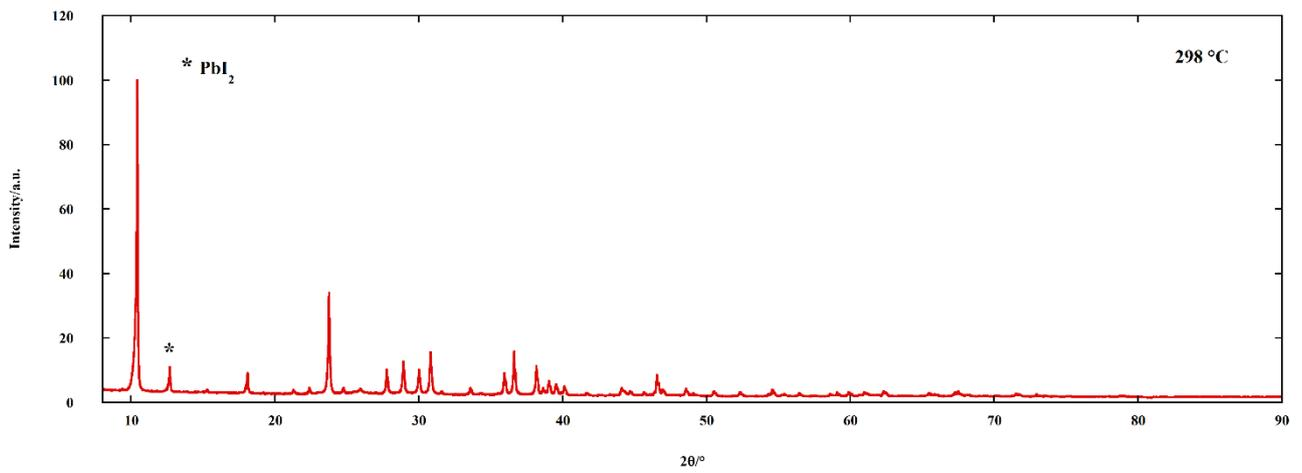
Fig. S2. X-ray powder diffraction pattern of  $N(\text{CH}_3)_4\text{PbI}_3$  after isothermal treatment at 298 °C for 10 hours.
