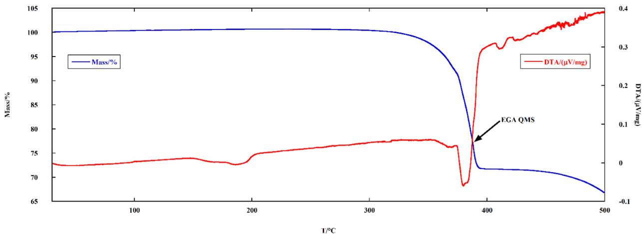
Fig. S7. TG-DTA curves of  $N(CH_3)_4PbI_3$  acquired in combination with QMS-EGA. The point of maximum ion currents intensities due to the gases evolved by the sample is indicated by an arrow.
