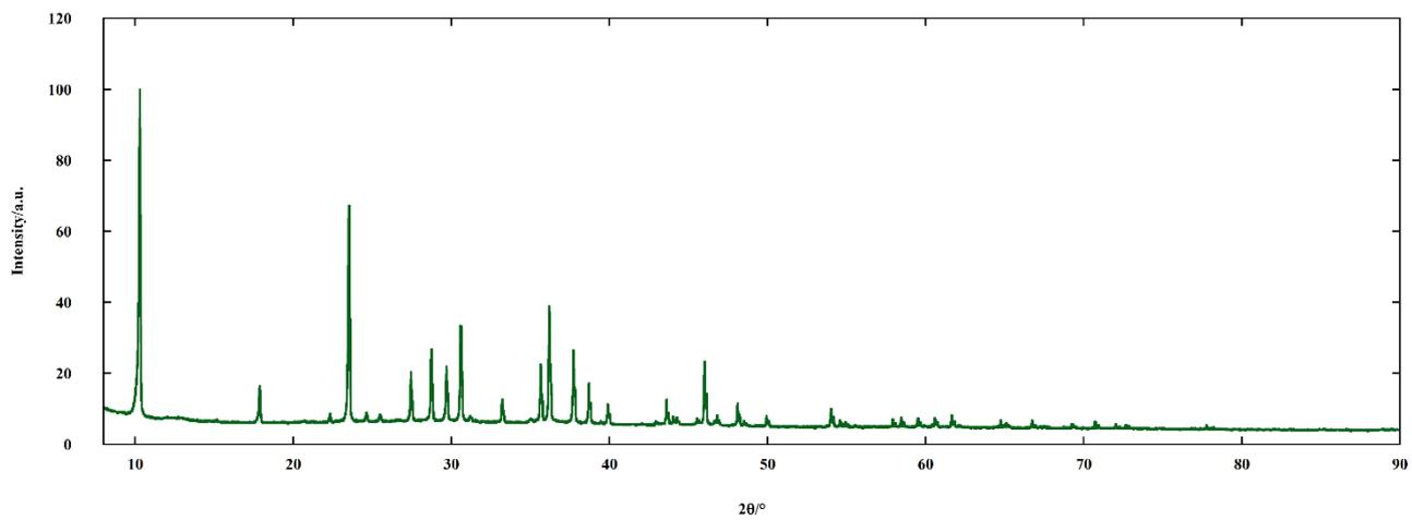
Fig. S6. X-ray powder diffraction pattern of  $\text{N}(\text{CH}_3)_4\text{PbI}_3$  acquired with environmental chamber at  $127\text{ }^\circ\text{C}$ .
