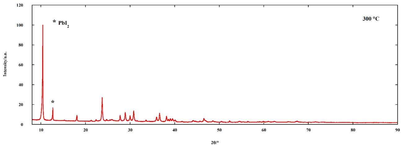
Fig. S3. X-ray powder diffraction pattern of  $\text{N}(\text{CH}_3)_4\text{PbI}_3$  after isothermal treatment at 300 °C for 10 hours.
