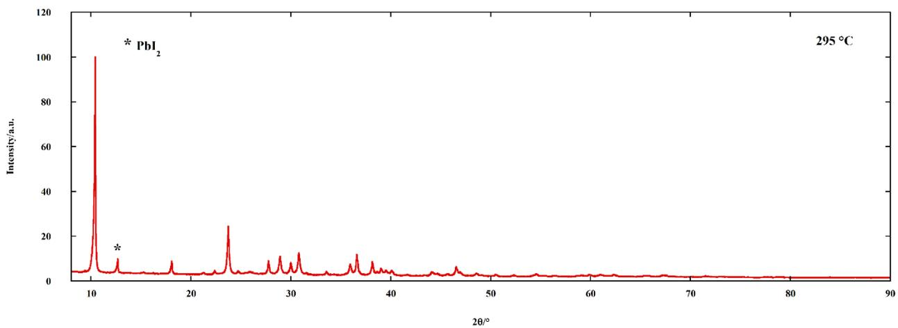
Fig. S1. X-ray powder diffraction pattern of  $\text{N}(\text{CH}_3)_4\text{PbI}_3$  after isothermal treatment at 295 °C for 10 hours.
