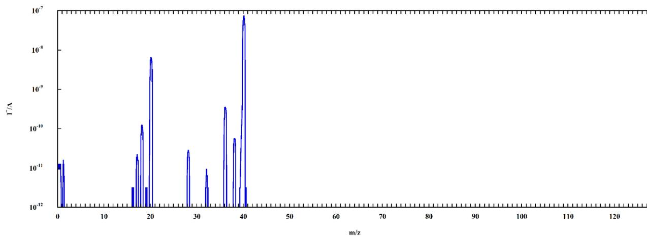
Fig. S8. Quadrupole mass spectrum of the carrier gas (Ar) used in the TG-DTA/QMS-EGA experiment.
