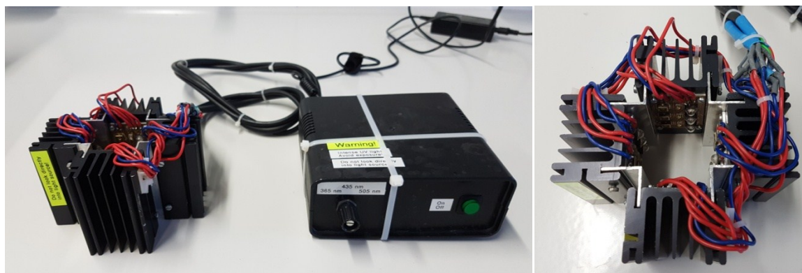
Fig. S12: Image of the photo reactor by Sahlmann Photochemical Solutions consisting of four single LED units (each comprising 3 LEDs of one wavelength) aligned in a 90° angle. Three different wavelengths can be selected (365 nm, 435 nm and 505 nm). The total light intensity in the center of the photo reactor (area: 5 × 5 cm 2 ) amounts to 85 mW/cm 2 .
