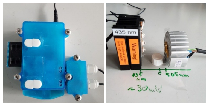
Fig. S3: In-house built automatic switching unit (left) connected to two light sources (435 nm and 505 nm, right).
