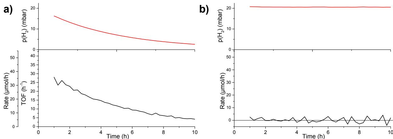
**Fig. S14** Backwards reaction rates measured on: a) impregnated 0.5% $\text{Pt}_{\text{NP}}:\text{TiO}_2$  and b) support blank ({001}-anatase) showing no noticeable activity.
