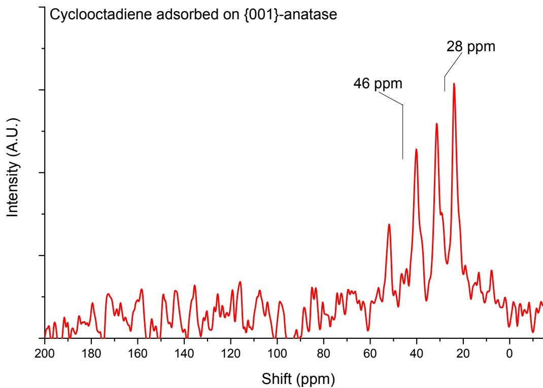
**Fig. S4** <sup>13</sup>C MAS SSNMR spectrum of cyclooctadiene adsorbed on {001}-anatase
