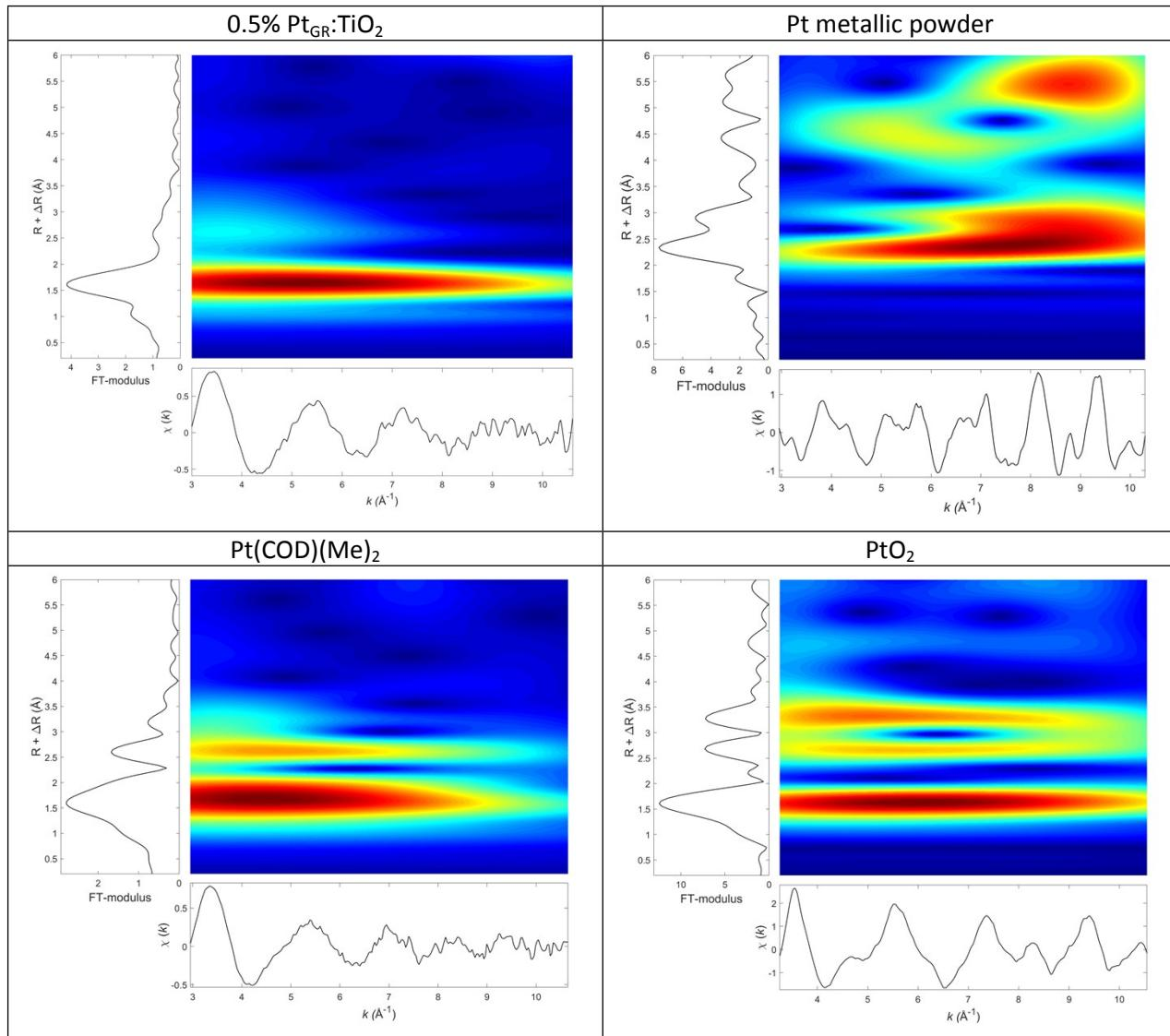
**Fig. S6** Contour plots of the wavelet transform magnitude showing the  $(k, R)$  localization of each FT-EXAFS contribution measured at the Pt L<sub>3</sub>-edge for 0.5% $\text{Pt}_{\text{GR}}\text{:TiO}_2$ , Pt metallic powder, Pt(COD)(Me)<sub>2</sub>, and  $\text{PtO}_2$
