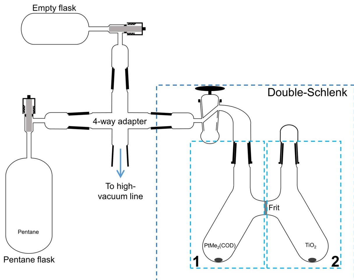
**Fig. S1** Setup used for grafting reactions
