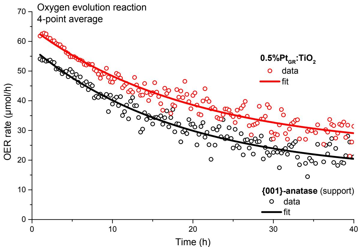
**Fig. S12** OER activity and exponential decay fits of  $\{\text{001}\}\text{-anatase}$  and  $0.5\%\text{Pt}_{\text{GR}}\text{:TiO}_2$ . First 30 minutes excluded due to gas mixing kinetics in the reactor
