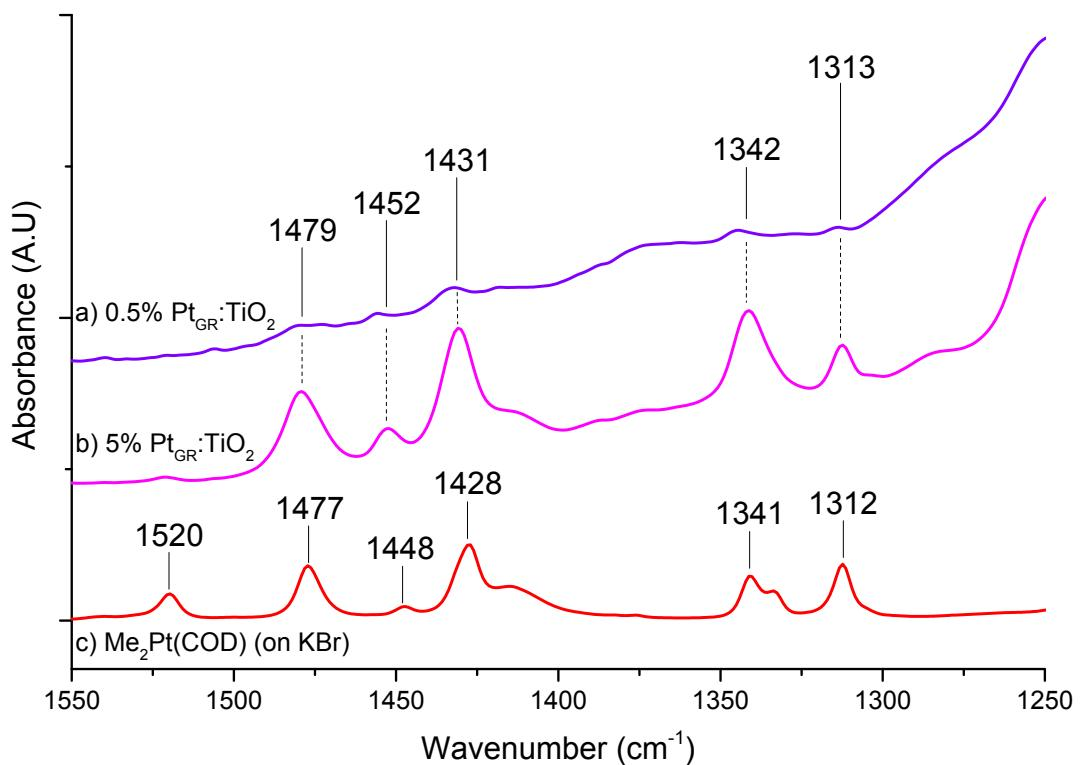
**Fig. S3** Infrared spectroscopy (DRIFTS) of a) 0.5%Pt<sub>GR</sub>:TiO<sub>2</sub>; b) 5% Pt<sub>GR</sub>:TiO<sub>2</sub>; c) Me<sub>2</sub>Pt(COD) on KBr.
