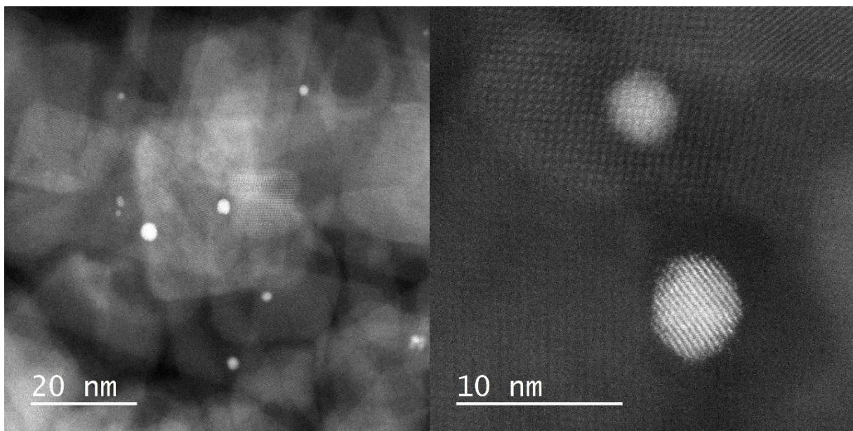
**Fig. S13** TEM micrographs of 0.5% $\text{Pt}_{\text{GR}}:\text{TiO}_2$  after photocatalysis with sacrificial methanol. Only nanoparticles are visible
