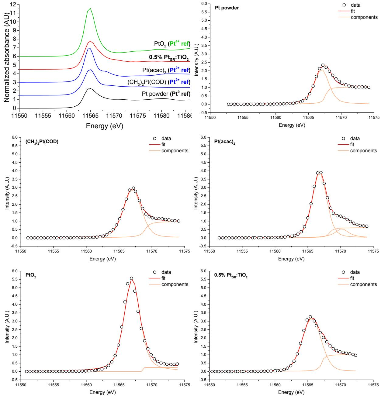
**Fig. S5** HERFD-XANES absorption spectra and fits using a pseudo-voigt function for the whiteline and arctangent function for the step. An additional lorentzian peak had to be included in the fitting model of the  $\text{Pt}(\text{acac})_2$  sample.
