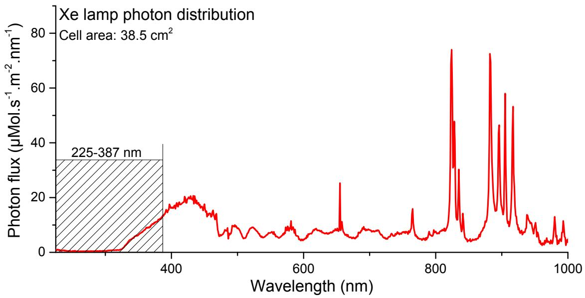
**Figure S11** Xenon lamp photon distribution.
