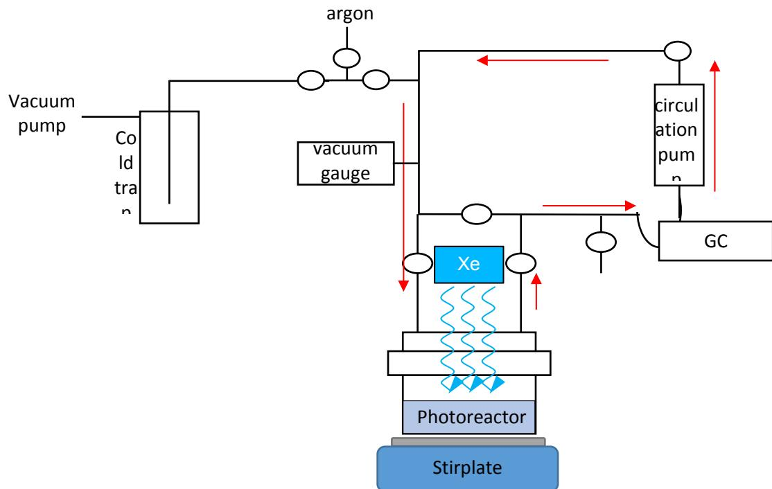
**Fig. S2** Photocatalysis setup
