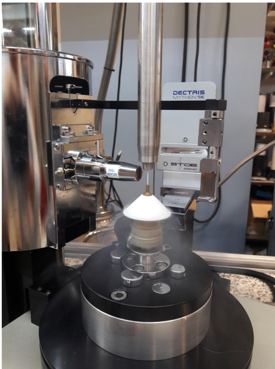
Fig. S59. View of the low-temperature set-up on the Stoe Stadi-P diffractometer equipped with a single Mythen 1K detector. The instrument has been modified so that the incident beam height is higher than normal to allow for the mounting of different sample environment stages. In addition, the set-up employs screw-in brass stubs with internal diameters from 0.2 to 1.2 mm (in 0.1 mm steps) as developed for use on the high-resolution PXRD beamlines BM16/ID31 at ESRF, and also used on, for example, the high-resolution PXRD beamline I11 at the Diamond synchrotron. The vertical axis of the Stadi-P is perfect for the use of the Oxford Instruments CryojetHT device that enables samples to be measured from about -173\text{ }^{\circ}\text{C} to 227\text{ }^{\circ}\text{C} . However, the rotating goniometer head disrupts the laminar shield flow of the CryojetHT. As a preventative measure against ice formation during data collection at the lowest temperatures, a conical polytetrafluoroethylene (PTFE/Teflon TM ) cone is fitted as shown, on which ice may form as a skirt at its outer edge only.
