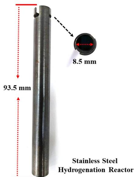
**Fig. S1.** The stainless steel hydrogenation reactor with a height of 93.5 mm and a diameter of 8.5 mm
