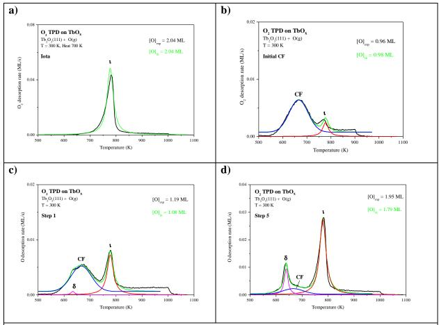
**Figure S2:** a) Measured and Lorentz fit of an  $O_2$  TPD spectrum for the reference  $\iota$ -phase, b) Measured and total fit of an  $O_2$  TPD spectrum obtained after oxidizing the initial CF-Tb<sub>2</sub>O<sub>3</sub> film. The measured spectrum was fit using the Lorentz peak determined in a) and a Voigt function to fit the broad CF peak. Measured and fitting peaks for c) Redox Step 1 and d) Redox Step 5.
