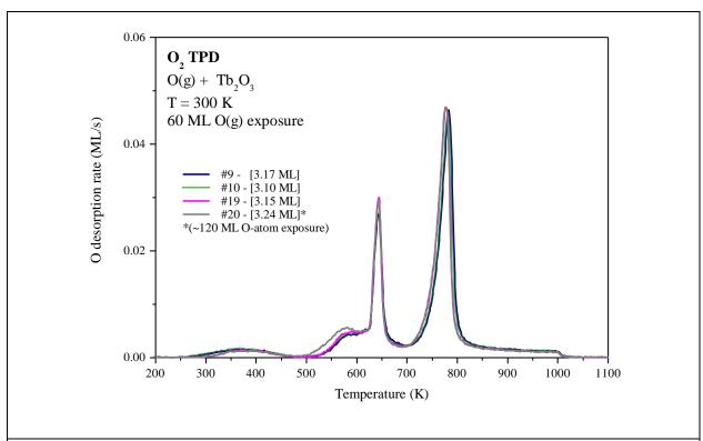
**Figure S1:** O<sub>2</sub> TPD spectra obtained after 9, 10 and 19 oxidation and reduction steps, with the O-atom exposure equal ~60 ML during the oxidation step. An O-atom exposure of ~120 ML was used in the 20<sup>th</sup> oxidation step.
