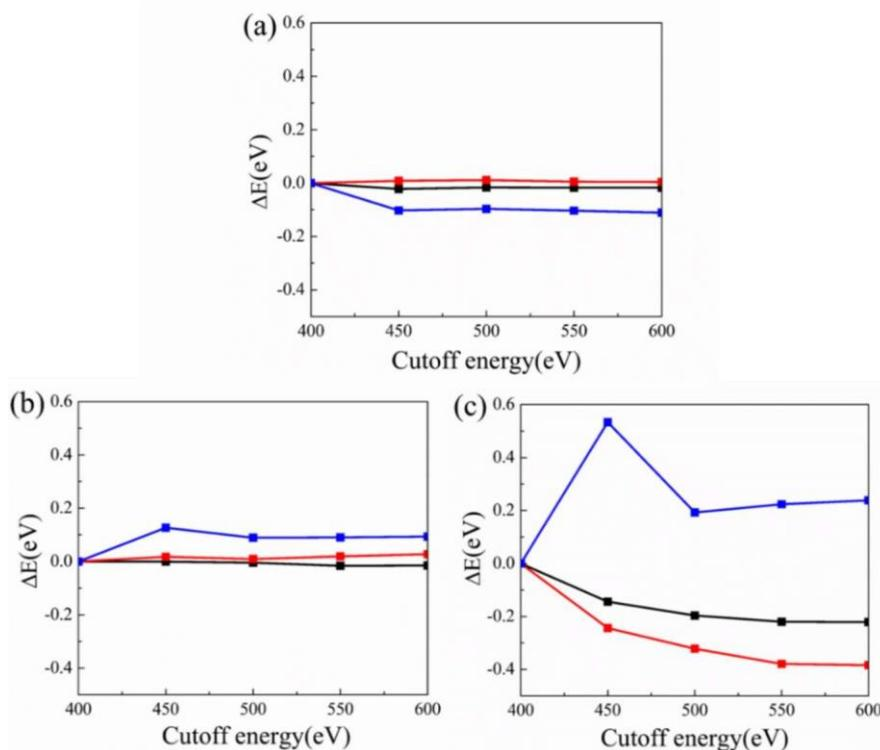
Figure 1S. Lattice energy convergence as a function of plane wave cutoff. (a) PBE. (b) DFT-D3. (c) optB88-vdW. Black for CHZ, red for CHZCP, and blue for CdCP.  $\Delta E$  is the difference of lattice energy taking the value of 400 eV as reference.
