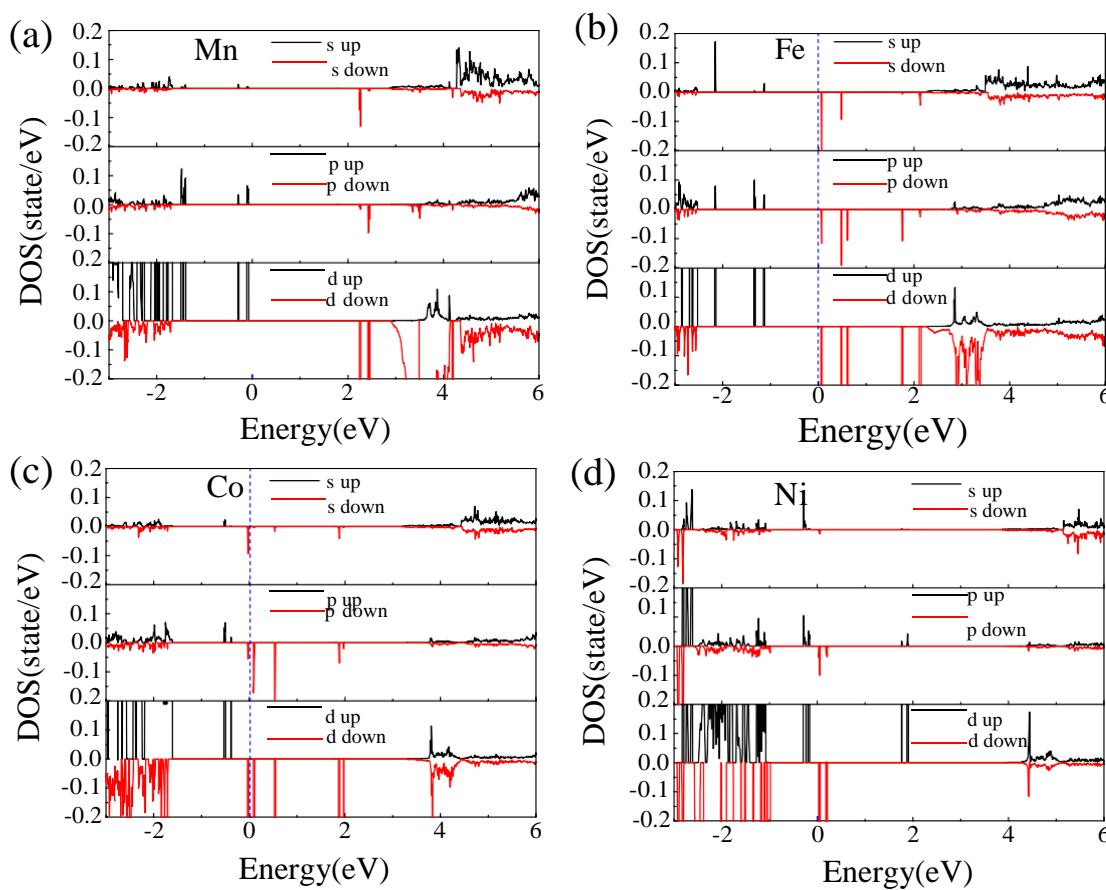
Figure 3S. Partial density of states of metal atoms in the molecular crystals. (a) MnCP. (b) FeCP. (c) CoCP. (d) NiCP.
