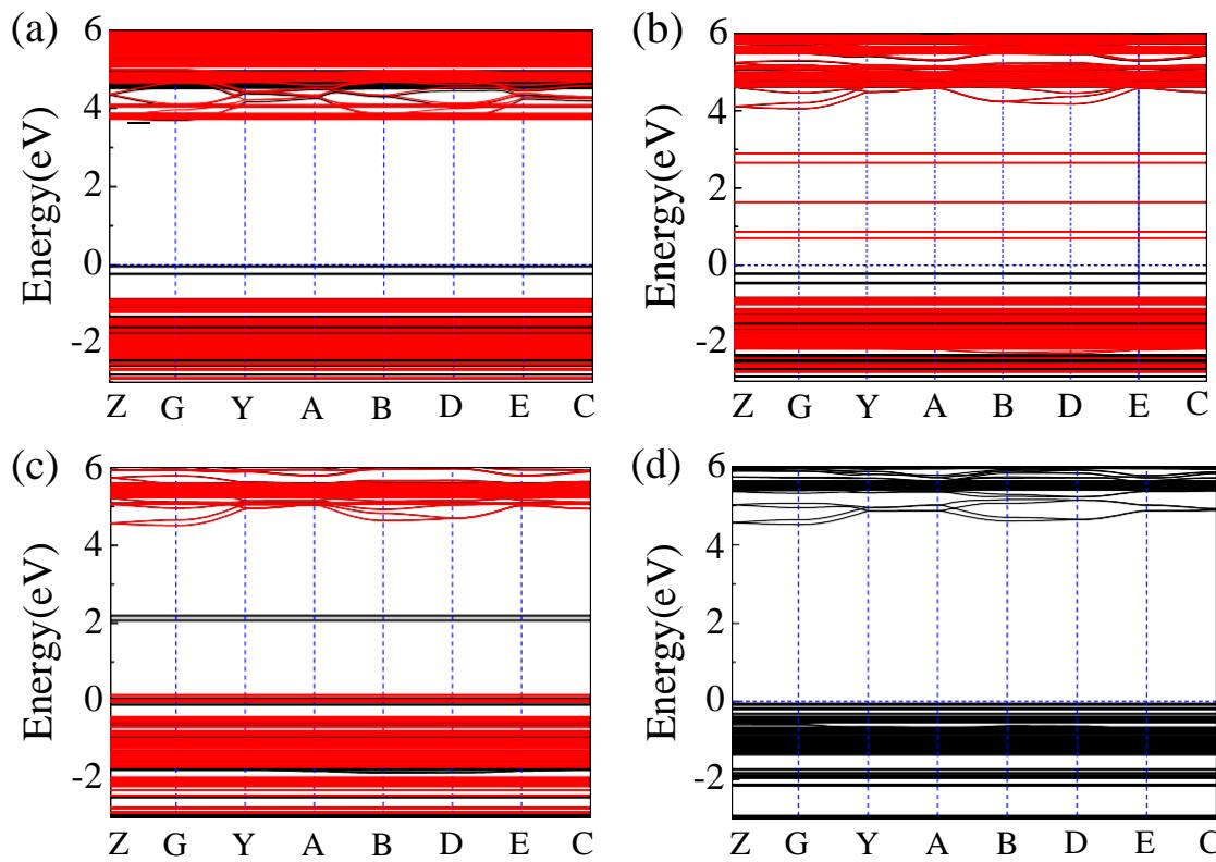
Figure 4S. The band structures of molecular crystals using the PBE+U. (a) MnCP. (b) CoCP. (c) NiCP. (d) CdCP. When the system is magnetic, black solid line represents spin up, red solid line represents spin down.
