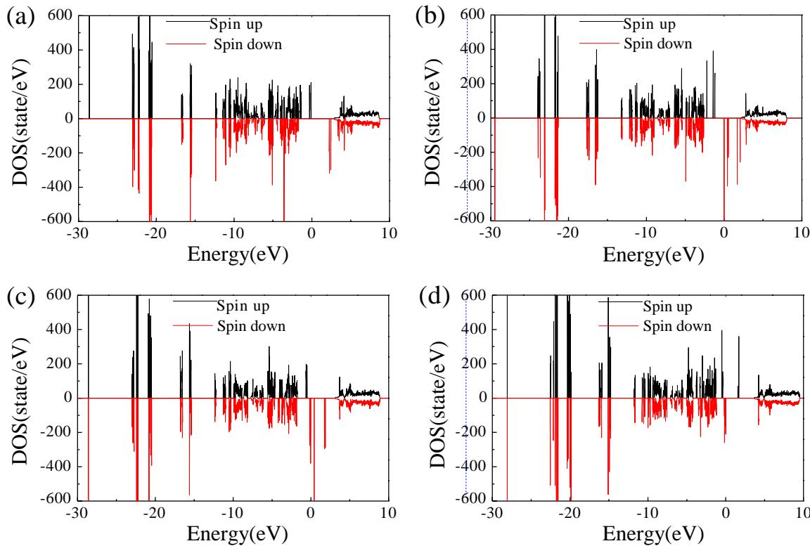
Figure 2S. The total density of states of four complexes. (a) MnCP. (b) FeCP. (c) CoCP. (d) NiCP.
