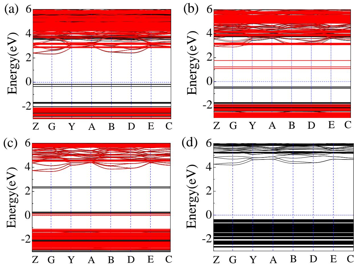
Figure 5S. The band structures of molecular crystals using the SCANrVV10. (a) MnCP. (b) CoCP. (c) NiCP. (d) CdCP. When the system is magnetic, black solid line represents spin up, red solid line represents spin down.
