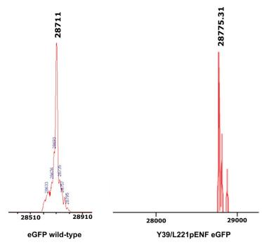
**Figure S1** Full-length ESI-MS spectra of eGFP wild-type and Y39/L221pENF eGFP after expression and purification. The mass shift of 64.31 Da between both proteins corresponds to the successful exchange of Y and L with 2 pENF.
