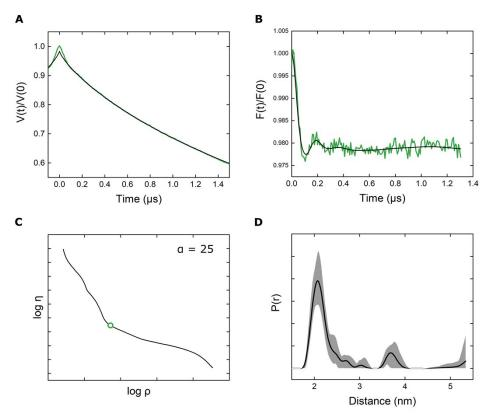
Figure S12 In vivo DEER distance determination of Y39/L221pENF-L eGFP. (A) Normalized DEER trace with homogeneous background fit (d = 2.36) (B) Background corrected form factor with fit by Tikhonov regularization. In triplicate measurements, we obtained varying modulation depths of 1-2% and comparable noise levels. (C) L-curve with the chosen alpha parameter (D) Validated distance distribution.
