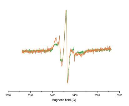
**Figure S8** Comparison of Y39/L221pENF-L eGFP *in vitro* (orange) and *in vivo* (green). Cw EPR spectra were recorded in X-band at room temperature and accumulated over 10 minutes (*in vitro*) or 50 minutes (*in vivo*). The narrow component corresponds to a small fraction of unbound spin label.
