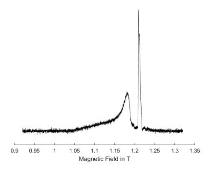
Figure S9 Q-band echo-detected field sweep of in-cell L221pENF-L eGFP at 50 K. The spectrum consists of contributions from remaining Cu(II) species after labeling (maximum at  $B = 1.18 \, T$ ) and nitroxide species (maximum at  $B = 1.21 \, G$ ). The Cu(II) contribution can be further decreased by additional washing of the cells, but at the cost of nitroxide signal intensity due to the rapid reduction in the cellular environment.
