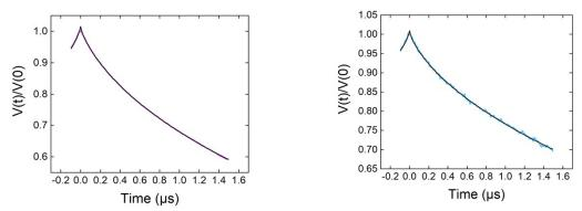
**Figure S11** Normalized DEER traces with homogeneous background fit for in vivo DEER measurements of with singly-labeled eGFP mutants Y39pENF-L (purple) and L221pENF-L (blue) (background start set to 0  $\mu$ s, background dimension is 2.2 or 2.3, respectively.)
