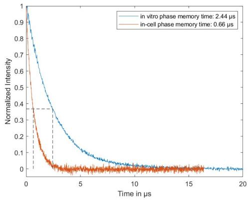
**Figure S10** Echo relaxation measurement with Y39/L221 pENF-L eGFP *in vitro* and *in vivo*. Phase memory times were determined as the time point at which the signal intensity decayed to 1/e of the initial intensity (t = 0  $\mu$ s). *In vivo* samples were prepared without deuterated solvents.
