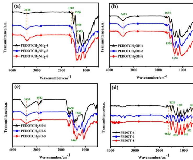
Fig. S4. FT-IR spectra of PEDOTCH<sub>2</sub>NH<sub>2</sub> (a), PEDOTCH<sub>2</sub>OH (b), PEDOTCH<sub>2</sub>SH (c) and PEDOT (d); the molar ratios of monomer to FeCl<sub>3</sub> are 1:4, 1:6 and 1:8
