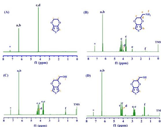
Fig. S2. <sup>1</sup>H-NMR of EDOT (A), EDOT-CH<sub>2</sub>NH<sub>2</sub> (B) EDOT-CH<sub>2</sub>OH (C) and EDOT-CH<sub>2</sub>SH (D); Starred peak comes from CDCl<sub>3</sub>
