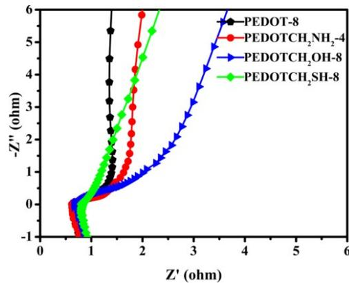
Fig. S7. The Nyquist Plots of PEDOTCH<sub>2</sub>NH<sub>2</sub>-4, PEDOTCH<sub>2</sub>OH-8, PEDOTCH<sub>2</sub>SH-8 and PEDOT-8: the molar ratios of monomer to FeCl<sub>3</sub> are 1:4 and 1:8; the applied potential: 0.61 V, amplitude: 5 mV and frequency range: 0.01-100 KHz.
