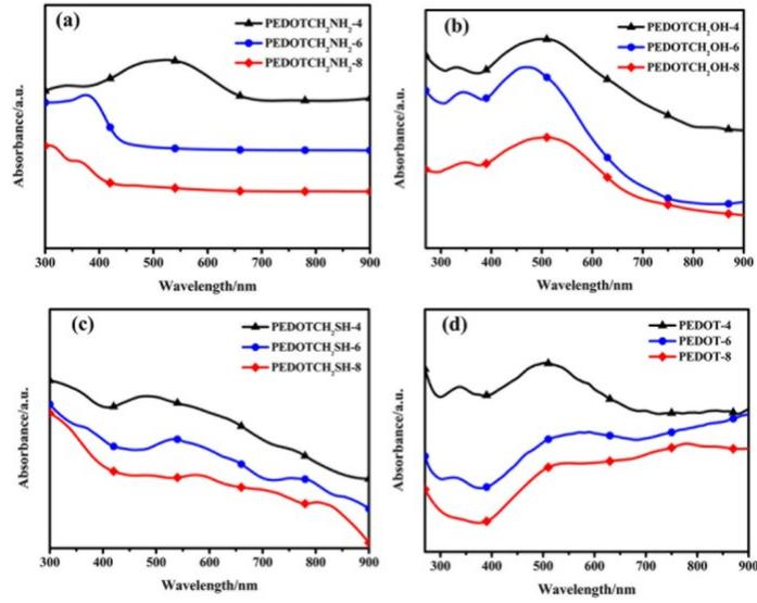
Fig. S5. UV-vis absorption spectra of PEDOTCH<sub>2</sub>NH<sub>2</sub> (a), PEDOTCH<sub>2</sub>OH (b), PEDOTCH<sub>2</sub>SH (c) and PEDOT (d); the molar ratios of monomer to FeCl<sub>3</sub> are 1:4, 1:6 and 1:8
