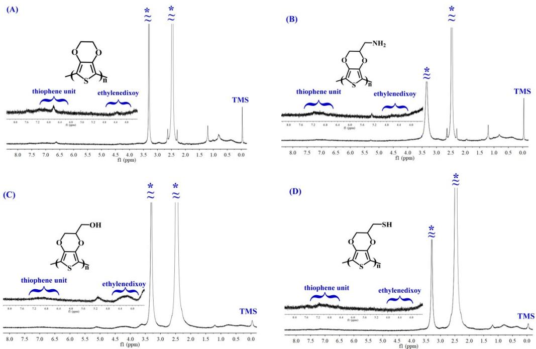
Fig. S3.  $^1\text{H-NMR}$  spectra of dedope-polymers in  $\text{DMSO-d}_6$  (treated with  $0.2\text{ M NaBH}_4(\text{aq})$ ); PEDOT (A), PEDOTCH<sub>2</sub>NH<sub>2</sub> (B), EDOTCH<sub>2</sub>OH (C) and EDOTCH<sub>2</sub>SH (D); Starred peak comes from H<sub>2</sub>O and DMSO-d<sub>6</sub>
