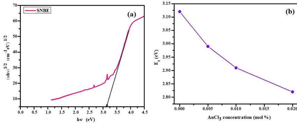
Figure S2: (a) Typical plot of  $(\alpha h\nu)^{1/2}$  versus  $(h\nu)$  in SNBE (gold free) glass, (b) variation of  $E_g$  as a function of  $\text{AuCl}_3$  concentration.
