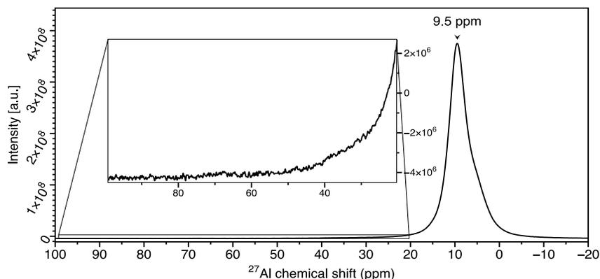
**Figure S1.** <sup>27</sup>Al MAS-NMR spectrum of  $\alpha$ -Al(OH)<sub>3</sub> stock used in the current study. Inset to the left of the peak at ca. 9.5 ppm shows magnified spectral region from 30 to 90 ppm where penta- (40 ppm) and tetra-coordinated (80 ppm) Al species are expected to be observed. Spin rate = 20 kHz.
