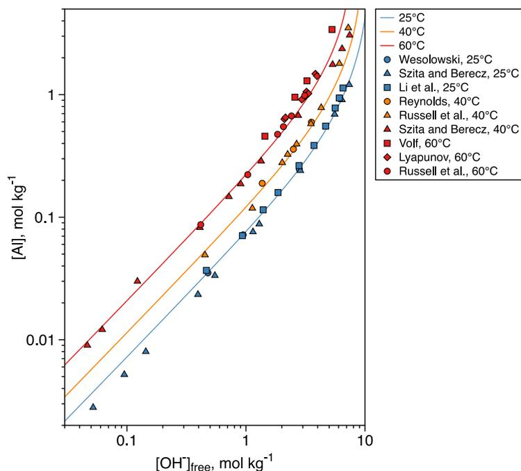
**Figure S4.** Comparison of the current  $\alpha\text{-Al(OH)}_3$  solubility model in  $\alpha\text{-Al(OH)}_3\text{-NaOH-H}_2\text{O}$  system at 25°C (blue trace), 45°C (orange trace), and 60°C (red trace) with literature values.
