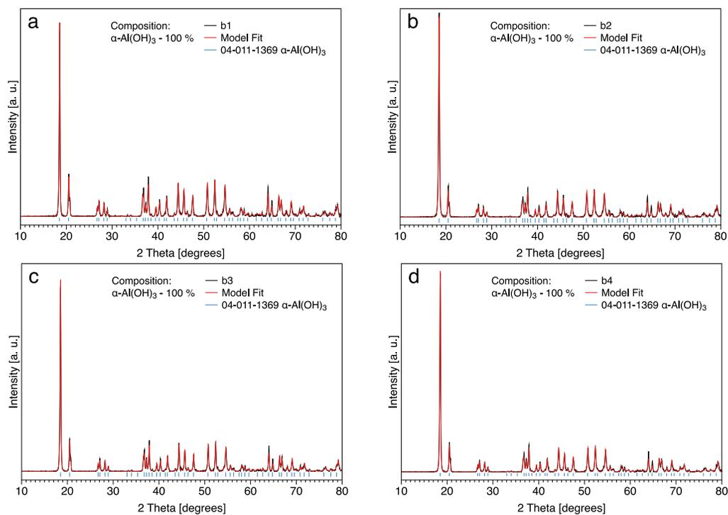
**Figure S3.** PXRD of solid phases extracted at the end of the experiments conducted at 45°C from oversaturation.
