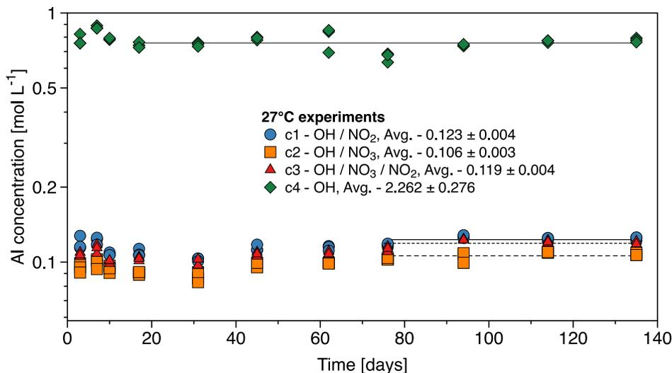
**Figure S5.**  $\alpha\text{-Al(OH)}_3$  solubility at 27°C as a function of varying NaNO<sub>2</sub>, NaNO<sub>3</sub>, and NaOH concentration. Horizontal lines indicate data regions used to obtain the displayed average plateau Al concentration.
