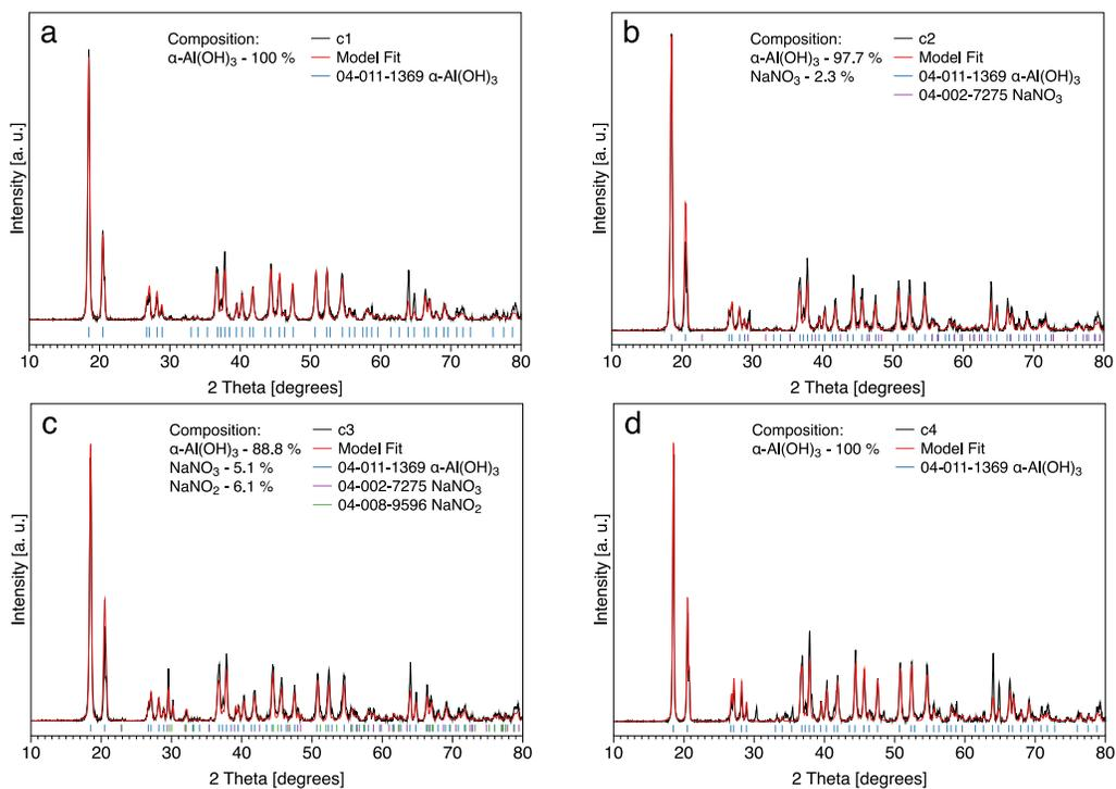
**Figure S7.** PXRD of solid phases extracted at the end of the experiments conducted at 27°C from undersaturation.
