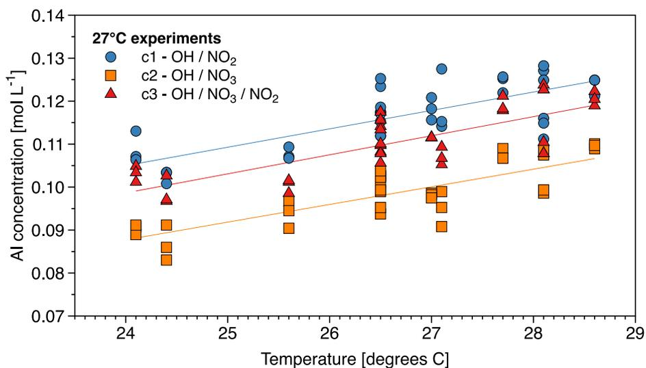
**Figure S6.** Dependence of  $\alpha\text{-Al(OH)}_3$  solubility on temperature in experiments c1-3.
