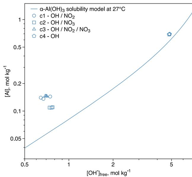
**Figure S8.** Measured  $\alpha\text{-Al(OH)}_3$  solubility in current experiments at versus solubility predicted from Pitzer model in the system of  $\alpha\text{-Al(OH)}_3\text{-NaOH-H}_2\text{O}$ .
