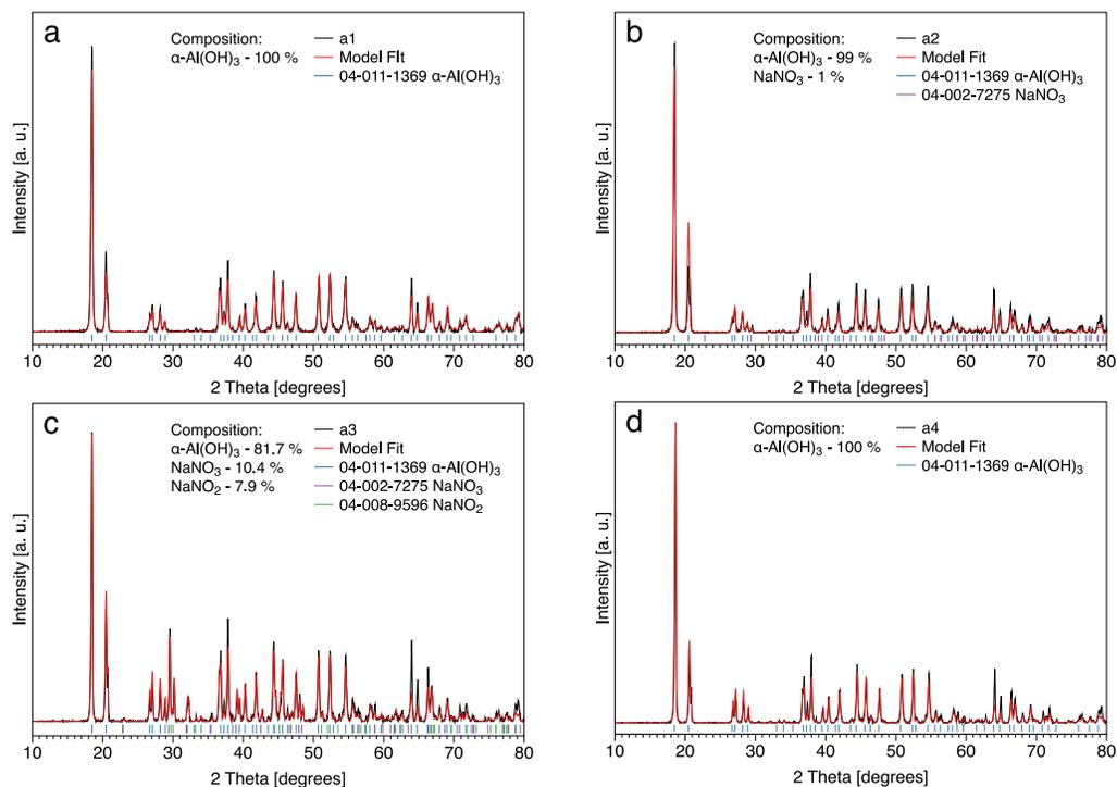
**Figure S2.** PXRD of solid phases extracted at the end of the experiments conducted at 45°C from undersaturation.
