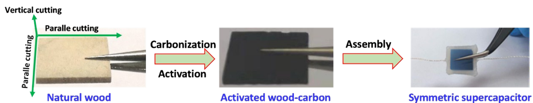
Figure S1. Construction of a quasi-solid-state symmetric supercapacitor (SSC) based on activated wood carbon (AWC) monoliths as freestanding thick electrodes.
