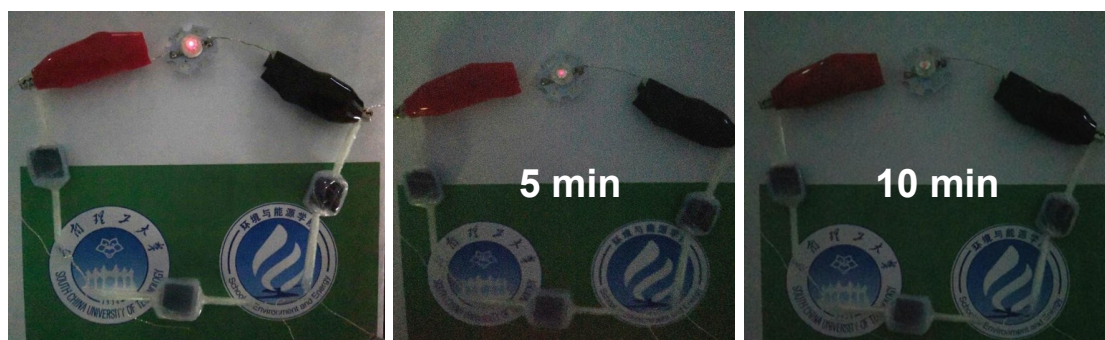
Figure S11. The quasi-solid-state SSC assembled by the two identical AWC powered an LED (1 W) for 10 mins by three in series.
