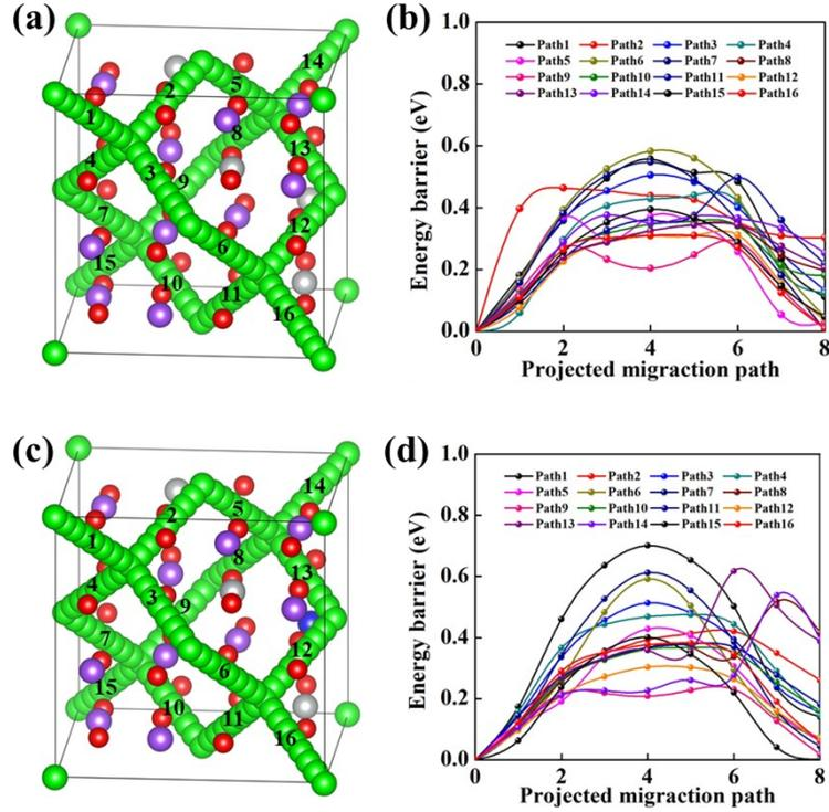
**Fig S3.** Illustration of 16 Li ion diffuse paths (a) and their corresponding (b) energy barriers in  $F\text{-LiNi}_{0.5}\text{Mn}_{1.5}\text{O}_4$ . Illustration of all 16 Li ion diffuse paths (c) and their corresponding (d) energy barriers in  $\text{Cr}_{\text{Ni}}\text{-}F\text{-LiNi}_{0.5}\text{Mn}_{1.5}\text{O}_4$ .
