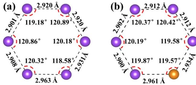
**Fig S4.** Bond lengths and bond angles of TM rings in (a)  $F\text{-LiNi}_{0.5}\text{Mn}_{1.5}\text{O}_4$  and (b)  $\text{Cr}_{\text{Ni}}\text{-}F\text{-LiNi}_{0.5}\text{Mn}_{1.5}\text{O}_4$ .
