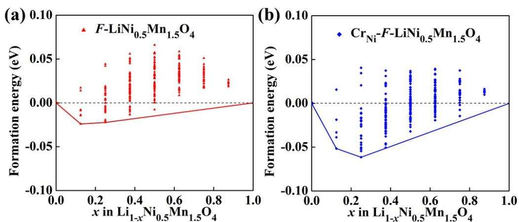
**Fig S2.** Formation energy and convex hulls of (a)  $\text{F-Li}_{1-x}\text{Ni}_{0.5}\text{Mn}_{1.5}\text{O}_4$  and (b)  $\text{Cr}_{\text{Ni}}\text{-F-Li}_{1-x}\text{Ni}_{0.5}\text{Mn}_{1.5}\text{O}_4$  as a function of delithiation content  $x$ .
