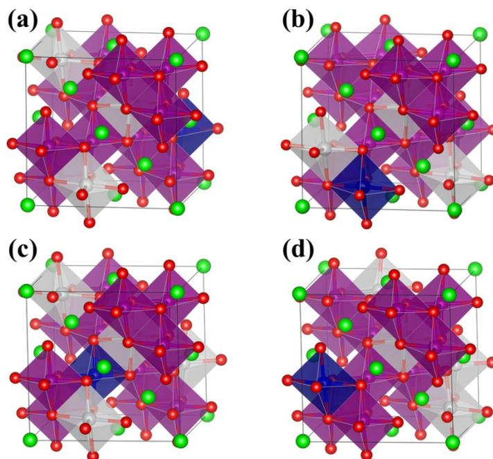
**Fig S1.** Most stable configurations of (a)  $\text{Cr}_{\text{Ni}}\text{-P-LiNi}_{0.5}\text{Mn}_{1.5}\text{O}_4$ , (b)  $\text{Cr}_{\text{Ni}}\text{-F-LiNi}_{0.5}\text{Mn}_{1.5}\text{O}_4$ , (c)  $\text{Cr}_{\text{Mn}}\text{-P-LiNi}_{0.5}\text{Mn}_{1.5}\text{O}_4$ , and  $\text{Cr}_{\text{Mn}}\text{-F-LiNi}_{0.5}\text{Mn}_{1.5}\text{O}_4$ .
