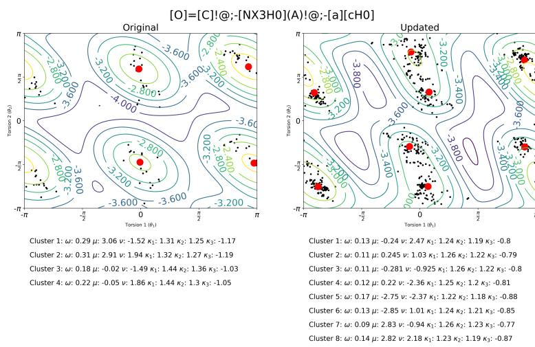
Figure S2: Mixture model for correlated torsions. The contour plot indicates the log density of a mixture model and the points (in red) mark the mean location for the components. **Left:** original correlated torsion that derived from filtered COD set. **Right:** updated correlated torsion by adding more observations from ChEMBL[12] database.
