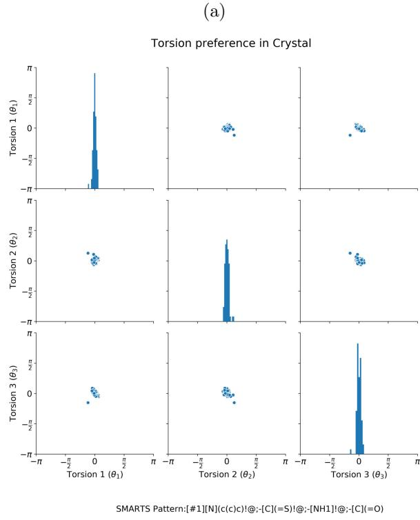
Figure S3: Higher order correlated torsions in (a) Crystal (b) MMFF94 and (c) GFN2. Torsion angles are measured in radian. We can see that all torsion angles are highly concentrated around  $0^\circ$  in crystal and GFN2. It suggests that the C=O and C=S are oriented in opposite directions and form a pseudo six-membered ring. This conformation promotes C=O – H-N intramolecular hydrogen bond. The torsion angles in MMFF94 form a bimodal distribution (around  $0^\circ$  and  $180^\circ$ ).
