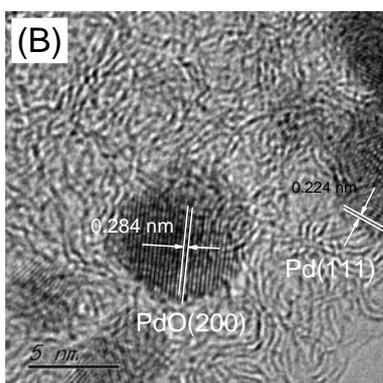
Figure S12. TEM images of the catalysts: (A) 2.5%Pd-PVP/C(1:2); (B) lattice fringe of Pd NPs on the catalyst 2.5%Pd-PVP/C(1:2).
