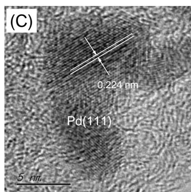
Figure S9. TEM images of the catalysts: (A) 1%Pd-PVP/C(1:2); (B) 1%Pd-PVP/C(1:2, 550°C); (C) lattice fringe of Pd NPs on the catalyst 1%Pd-PVP/C(1:2); (D) lattice fringe of Pd NPs on the catalyst 1%Pd-PVP/C(1:2, 550°C).
