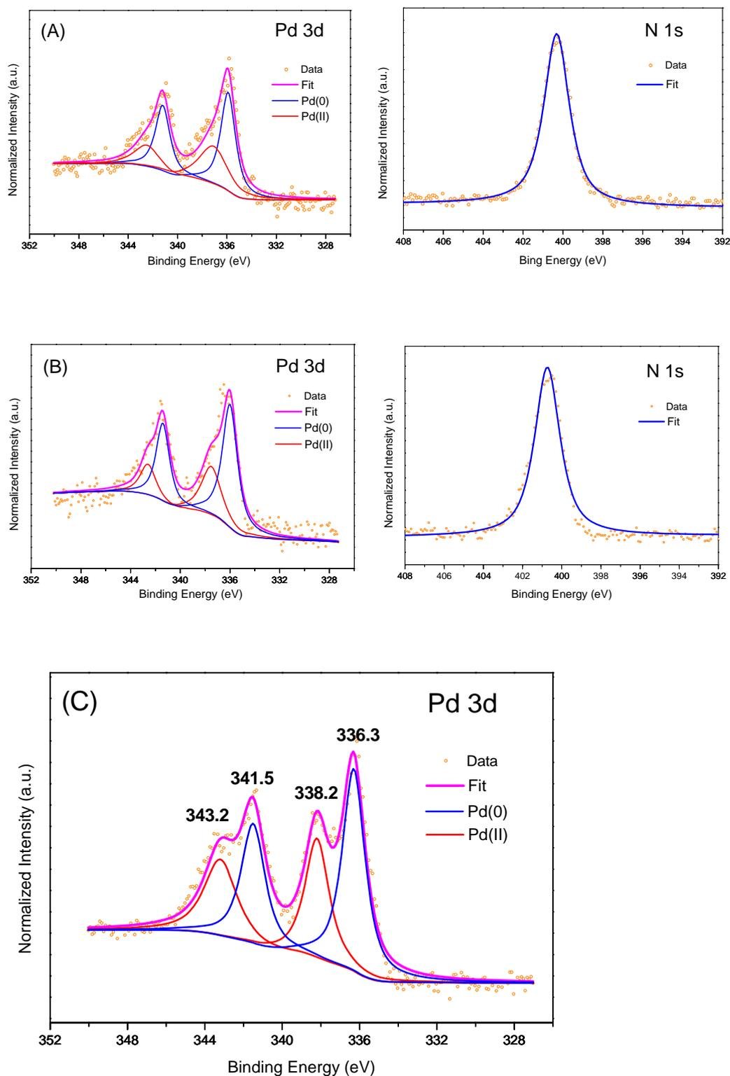
Figure S15. XPS spectra for Pd (3d) and N (1s) of the catalysts: (A) 2.5%Pd-PVP/C(1:2); (B) 5%Pd-PVP/C(1:2); (C) commercial Pd/C.
