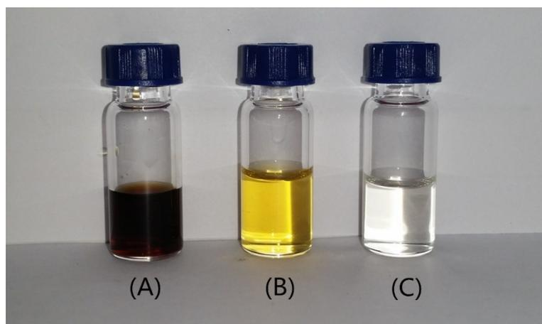
Figure S7 The photos of the products: (A) The reaction product without any catalyst; (B) The reaction product using catalyst 1%Pd-PVP(1-2); (C) The reaction product using catalyst commercial Pd
