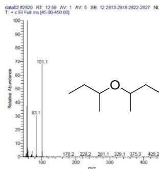
Figure S6. GC-Mass spectra of the overhydrogenation products obtained from using the commercial Pd/C as the catalyst..
