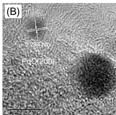
Figure S13. TEM images of the catalysts: (A) 5%Pd-PVP/C(1:2); (B) lattice fringe of Pd NPs on the catalyst 5%Pd-PVP/C(1:2).
