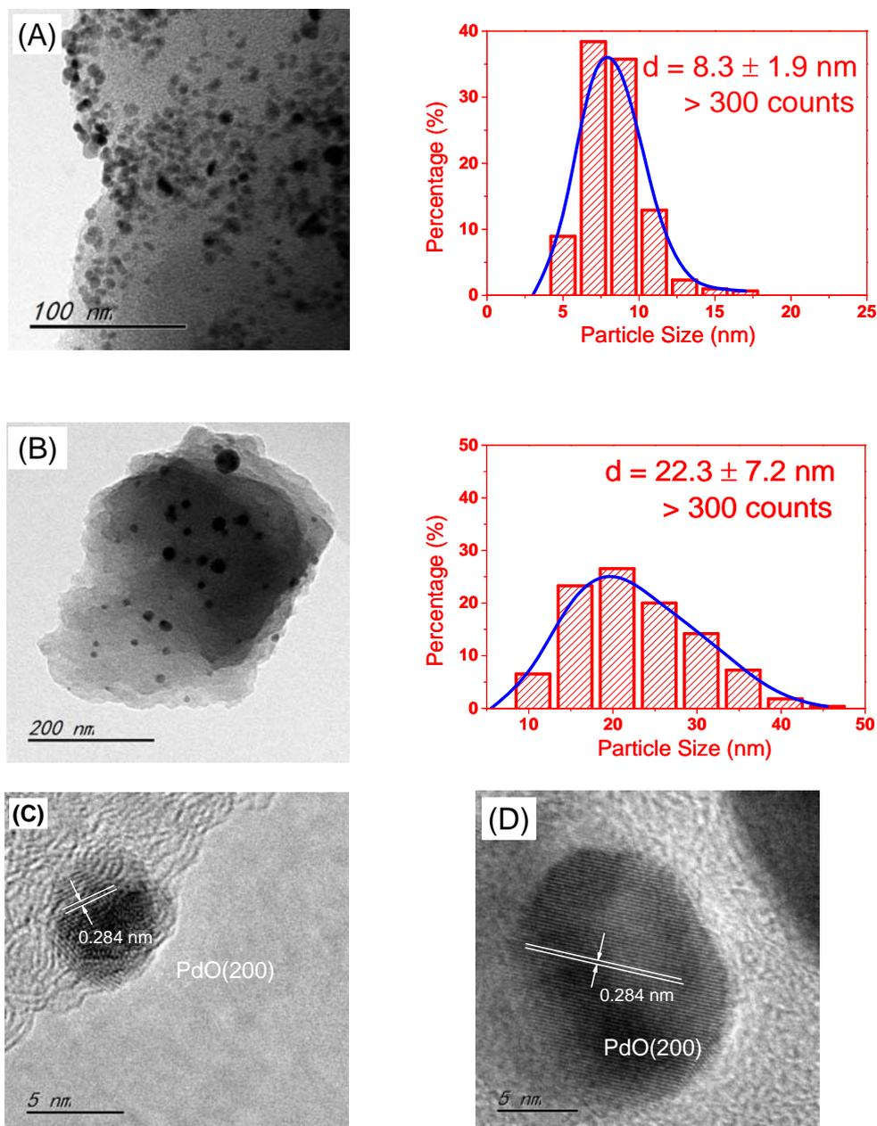
Figure S8. TEM images of the catalysts: (A) 1%Pd-PVP/C(1:1); (B) 1%Pd-PVP/C(1:1, 550°C); (C) lattice fringe of Pd NPs on the catalyst 1%Pd-PVP/C(1:1); (D) lattice fringe of Pd NPs on the catalyst 1%Pd-PVP/C(1:1, 550°C).
