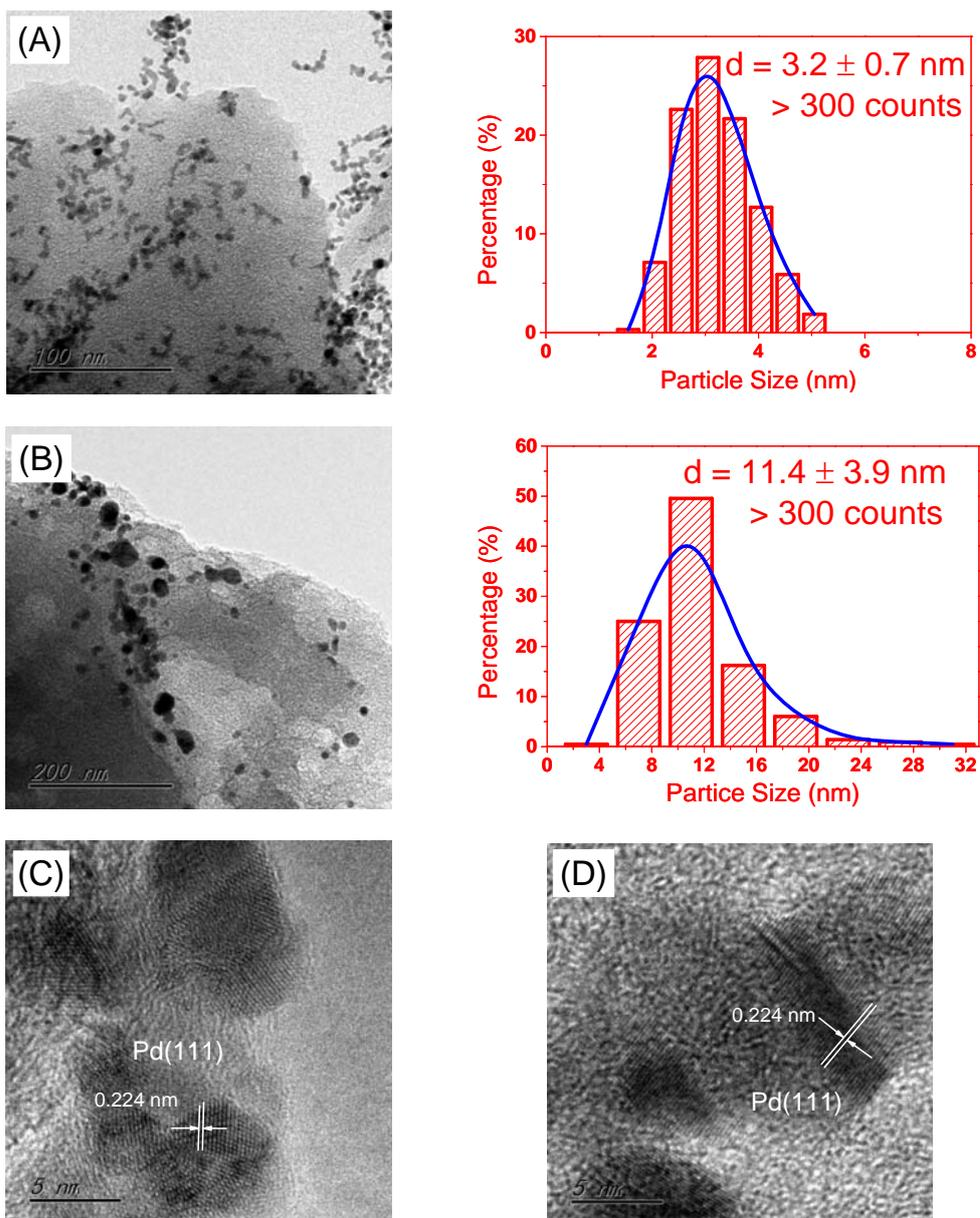
Figure S10. TEM images of the catalysts: (A) 1%Pd-PVP/C(1:4); (B) 1%Pd-PVP/C(1:4, 550°C); (C) lattice fringe of Pd NPs on the catalyst 1%Pd-PVP/C(1:4); (D) lattice fringe of Pd NPs on the catalyst 1%Pd-PVP/C(1:4, 550°C).
