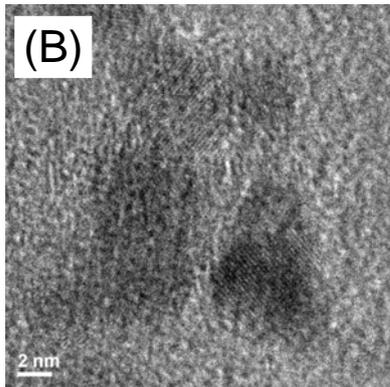
Figure S11. TEM images of the catalysts: (A) commercial Pd/C; (B) lattice fringe of Pd NPs on the commercial Pd/C
