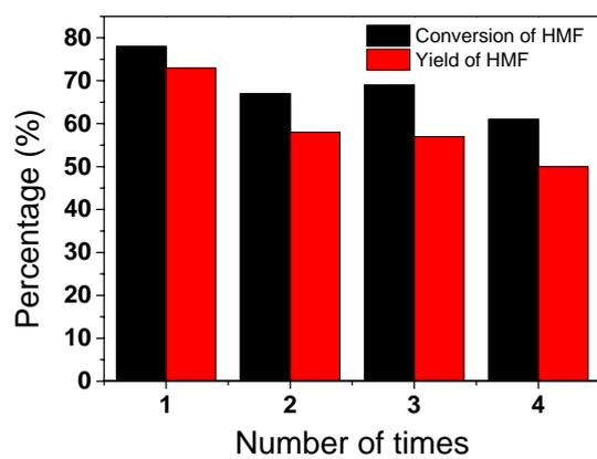
Figure S16 Recycle experiments for 1%Pd-PVP/C(1:2). Reaction conditions:
