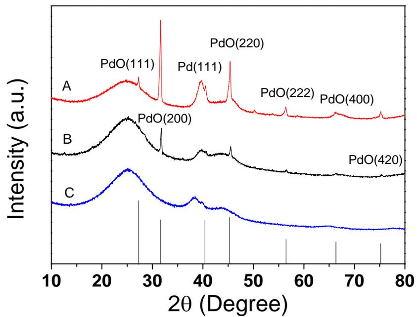
Figure S14. XRD patterns of the catalysts: (A) commercial Pd/C; (B) 5%Pd-PVP/C(1:2); (C) 2.5%Pd-PVP/C(1:2).
