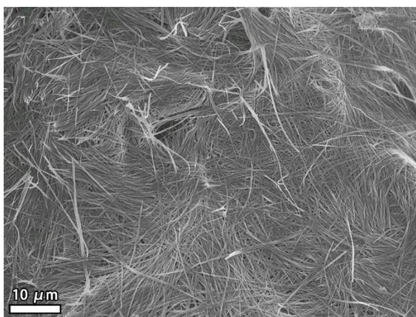
**Figure S1.** Morphology characterization: SEM image of MnO<sub>2</sub>-GOS-TiO<sub>2</sub>.
