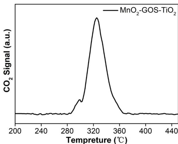
**Figure S3.** The temperature-programmed oxidation (TPO) of GO in reaction atmosphere.
