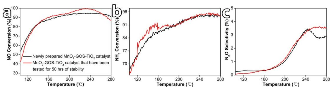
Figure S7. Catalyst performance: (a) NO conversion, (b) NH<sub>3</sub> conversion and (c) N<sub>2</sub>O selectivity of newly prepared and used MnO<sub>2</sub>-GOS-TiO<sub>2</sub> catalyst in the presence of steam.
