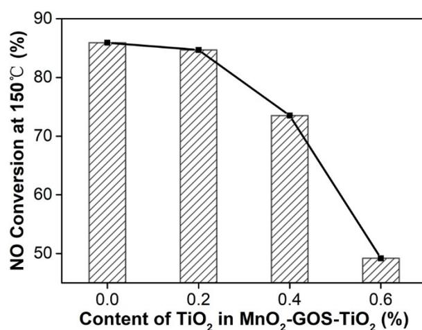
Figure S6. Relationship between catalyst performance and content of TiO<sub>2</sub> in MnO<sub>2</sub>-GOS-TiO<sub>2</sub>.
