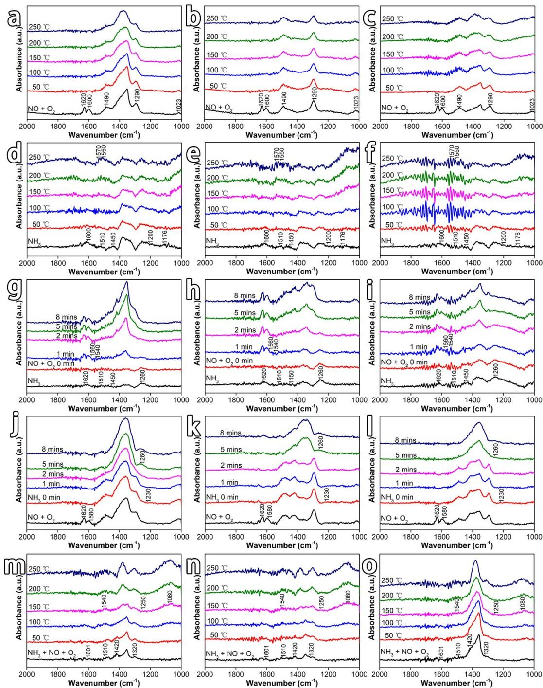
Figure S9. DRIFT study on  $\text{NH}_3$ -SCR mechanism of  $\text{MnO}_2$ ,  $\text{MnO}_2\text{-TiO}_2$  and  $\text{MnO}_2\text{-GOS-TiO}_2$ .
