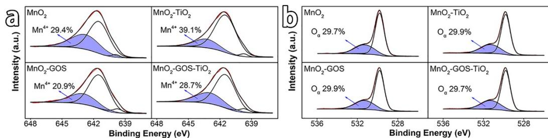
**Figure S8.** XPS spectra for (a) Mn 2p<sub>3/2</sub> and (b) O 2p<sub>3/2</sub> for MnO<sub>2</sub>, MnO<sub>2</sub>-TiO<sub>2</sub>, MnO<sub>2</sub>-GOS and MnO<sub>2</sub>-GOS-TiO<sub>2</sub>.
