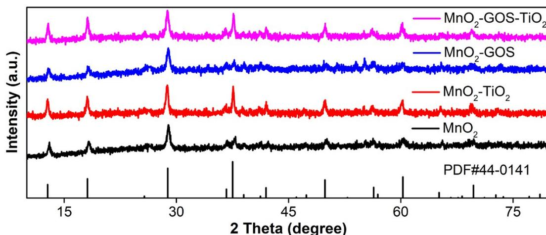
**Figure S2.** Structural characterization, XRD pattern of  $\text{MnO}_2$ ,  $\text{MnO}_2\text{-TiO}_2$ ,  $\text{MnO}_2\text{-GOS}$  and  $\text{MnO}_2\text{-GOS-TiO}_2$ .
