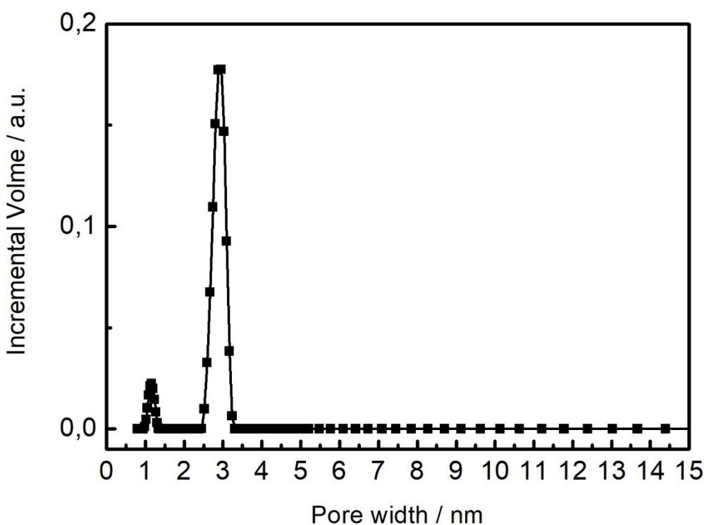
**Figure S8.** Pore size distribution of PCN-222(Rh).
