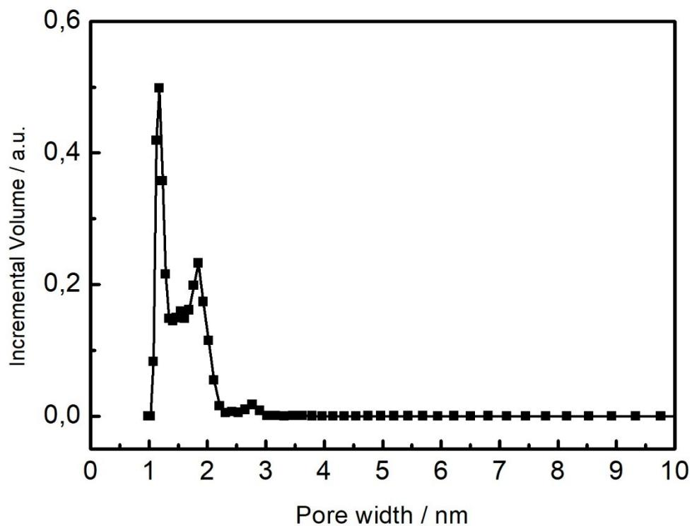
**Figure S6.** Pore size distribution of PCN-224(Rh).
