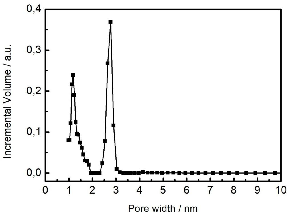
**Figure S9.** Pore size distribution of PCN-222.
