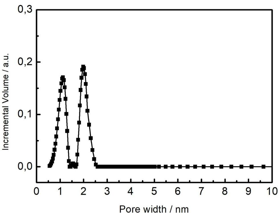
**Figure S7.** Pore size distribution of PCN-224.
