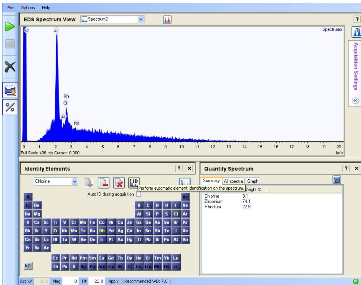
**Figure S3.** Energy dispersive spectra of PCN-222(Rh).
