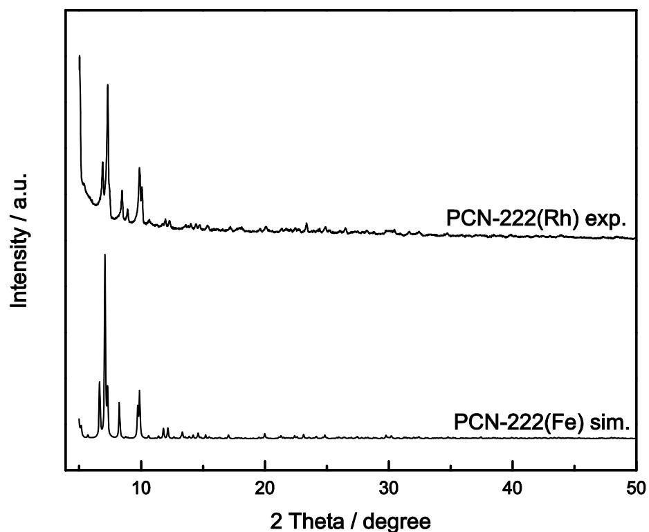
**Figure S4.** Experimental PXRD pattern of PCN-222(Rh) in comparison to the simulated pattern of PCN-222(Fe).
