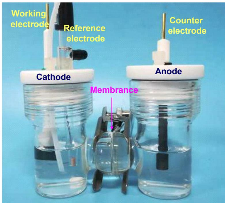
Fig. S3. Photograph of H-type electrochemical setup
