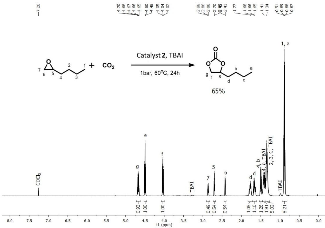
**Figure S29.** Crude <sup>1</sup>H-NMR spectra of cycloaddition of CO<sub>2</sub> to 1,2-Epoxyhexane by using catalyst **2** with TBAI (Table 3, Entry 9).
