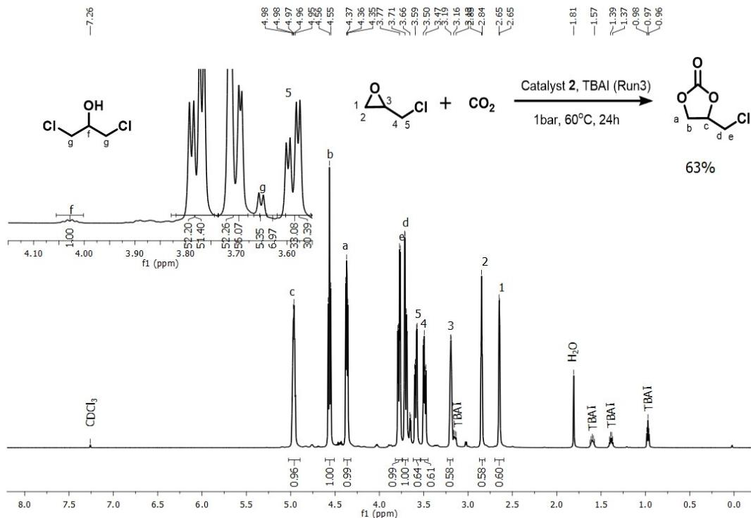
**Figure S28.** Crude <sup>1</sup>H-NMR spectra of cycloaddition of CO<sub>2</sub> to Epichlorohydrin by using catalyst **2** with TBAI (Run 3, Table 3, Entry 8).
