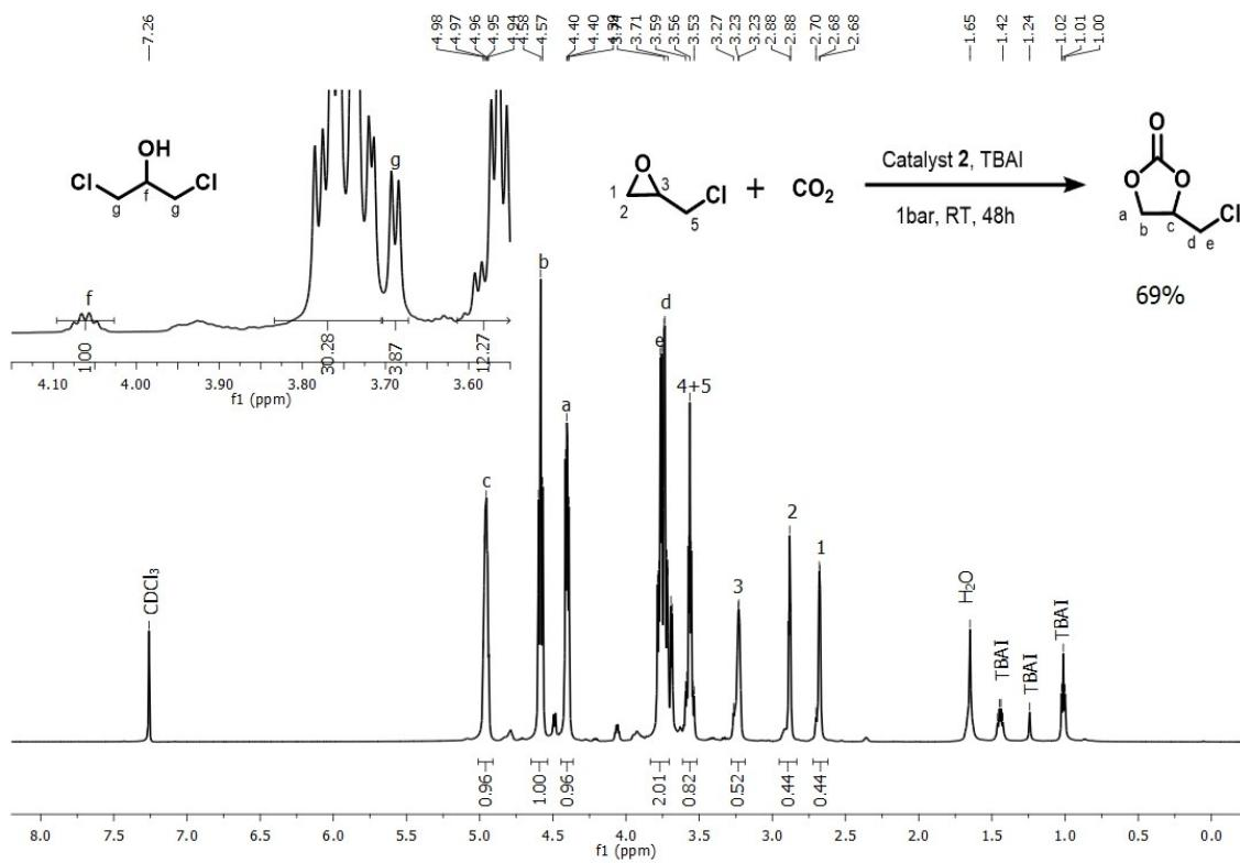
**Figure S37.** Crude <sup>1</sup>H-NMR spectra of cycloaddition of CO<sub>2</sub> to Epichlorohydrin by using catalyst **2** with TBAI at room temperature for 48 h (Table 3, Entry 18).
