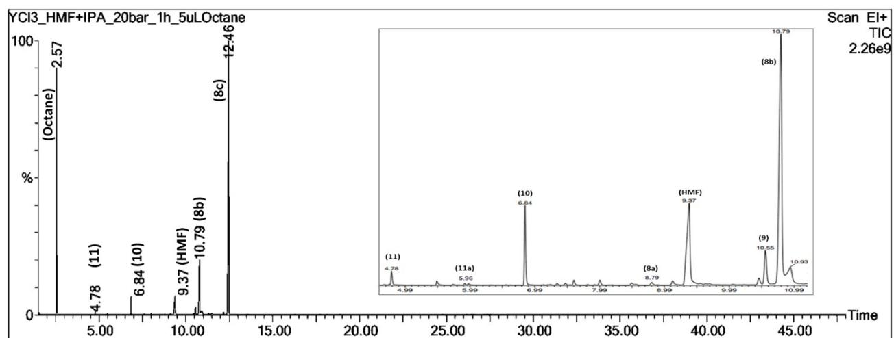
**Figure S42.** Chromatogram of reductive etherification of HMF catalyzed by YCl<sub>3</sub> at 150 °C, 20 bar N<sub>2</sub> for 1 h (Table S5, Entry 3).
