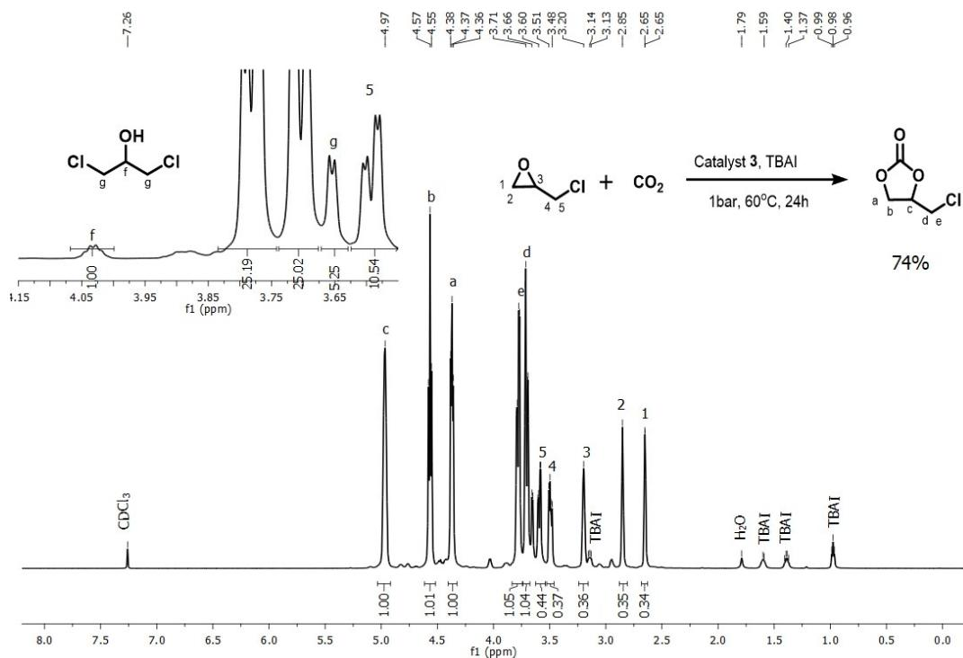
**Figure S30.** Crude <sup>1</sup>H-NMR spectra of cycloaddition of CO<sub>2</sub> to Epichlorohydrin by using catalyst **3** with TBAI (Table 3, Entry 10).
