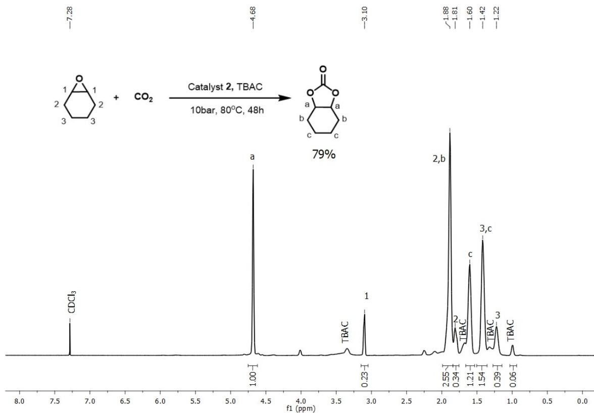
**Figure S36.** Crude <sup>1</sup>H-NMR spectrum of cycloaddition of CO<sub>2</sub> to cyclohexene oxide (**5i**) by using catalyst **2** with TBAC at 80°C, 10 bar CO<sub>2</sub> for 48 h (Table 3, Entry 16).
