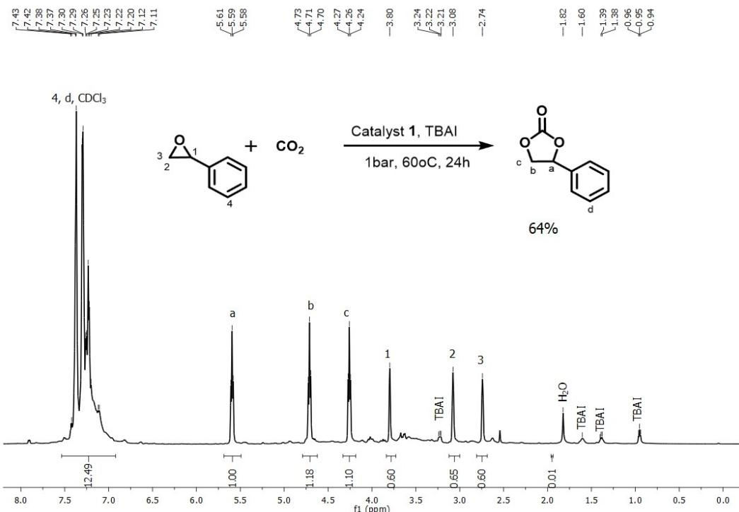
**Figure S25.** Crude <sup>1</sup>H-NMR spectra of cycloaddition of CO<sub>2</sub> to Styrene oxide by using catalyst **1** with TBAI (Table 3, Entry 7).
