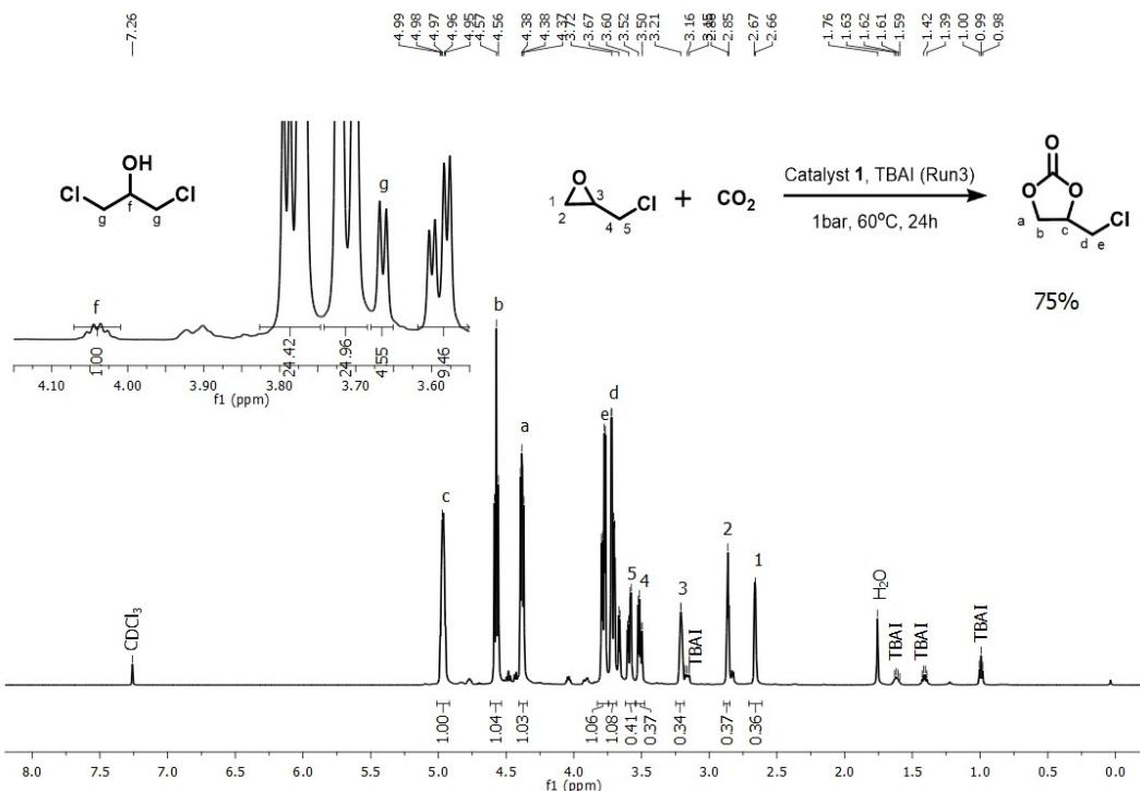
**Figure S21.** Crude <sup>1</sup>H-NMR spectra of cycloaddition of CO<sub>2</sub> to Epichlorohydrin by using catalyst **1** with TBAI (Run 3, Table 3, Entry 5).
