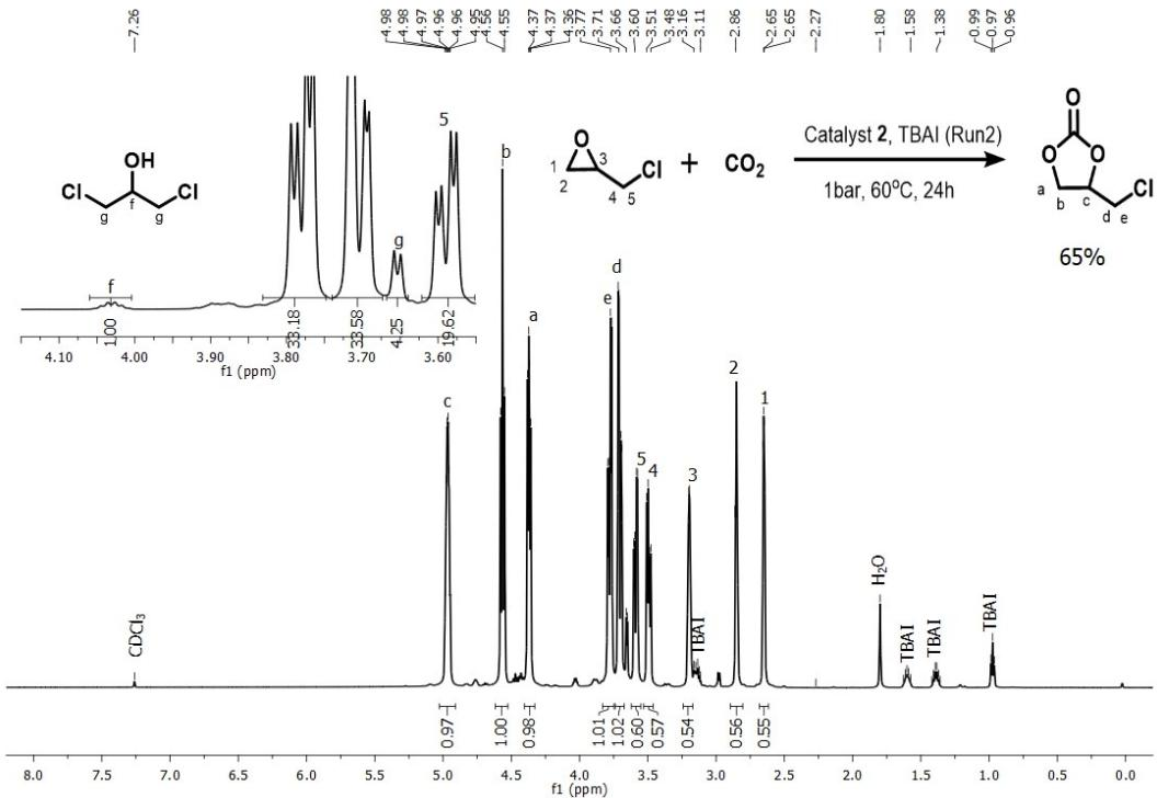
**Figure S27.** Crude <sup>1</sup>H-NMR spectra of cycloaddition of CO<sub>2</sub> to Epichlorohydrin by using catalyst **2** with TBAI (Run 2, Table 3, Entry 8).
