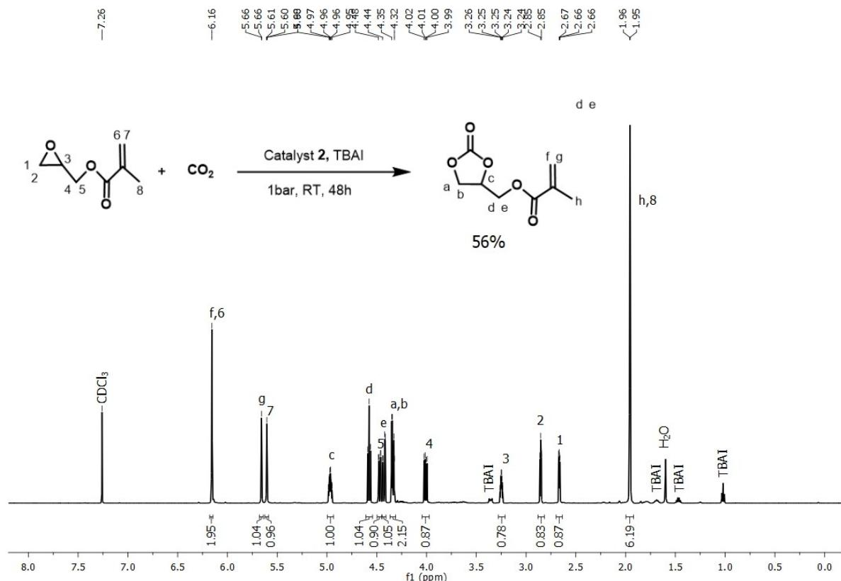
**Figure S38.** Crude <sup>1</sup>H-NMR spectrum of cycloaddition of CO<sub>2</sub> to glycidyl methacrylate (**5h**) by using catalyst **2** with TBAI at room temperature for 48 h (Table 3, Entry 19).
