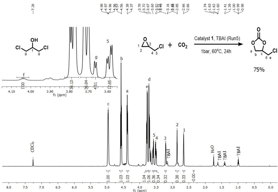
**Figure S23.** Crude  $^1\text{H}$ -NMR spectra of cycloaddition of  $\text{CO}_2$  to Epichlorohydrin by using catalyst **1** with TBAI (Run 5, Table 3, Entry 5).
