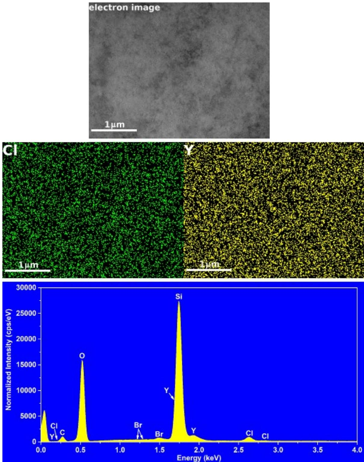
Figure S12. (top) electron image, (center) Y and Cl EDS mappings and (bottom) EDS spectrum of 2.
