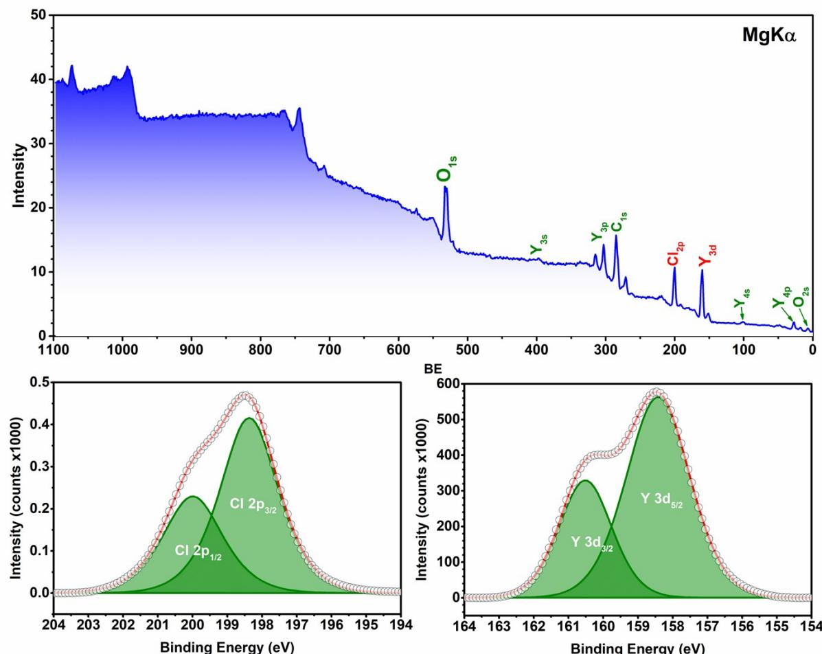
**Figure S8.** Survey (top) and excerpts of high-resolution XPS spectrum (bottom) of anhydrous  $\text{YCl}_3$ .
