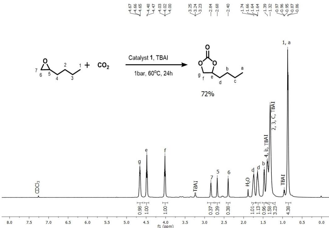
**Figure S15.** Crude  $^1\text{H}$ -NMR spectra of cycloaddition of  $\text{CO}_2$  to 1,2-Epoxyhexane by using catalyst **1** with TBAI (Table 3, Entry 1).
