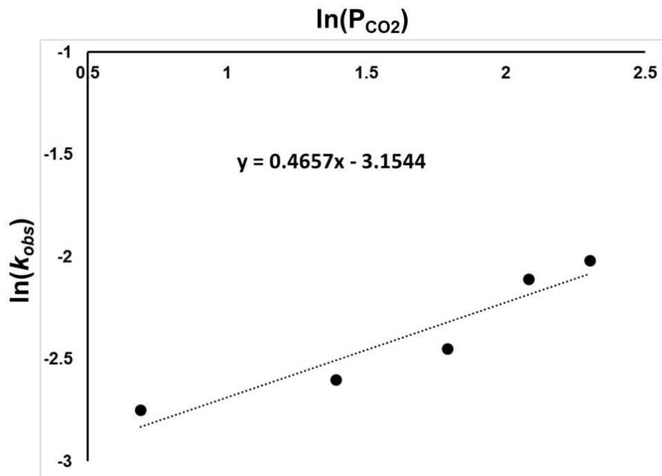
**Figure S40.** Logarithmic plot of apparent reaction rates ( $k_{obs}$ ) at different CO<sub>2</sub> pressures for the cycloaddition of CO<sub>2</sub> to epichlorohydrin catalyzed by homogeneous YCl<sub>3</sub>/TBAI.
