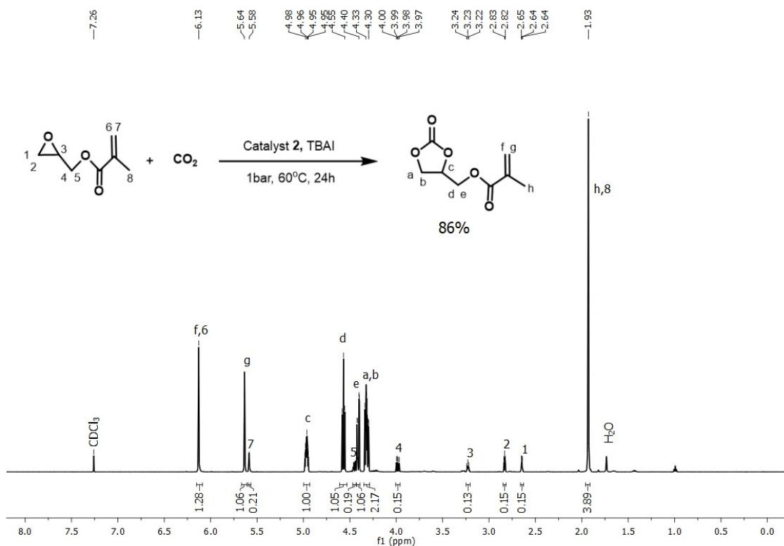
**Figure S32.** Crude <sup>1</sup>H-NMR spectra of cycloaddition of CO<sub>2</sub> to Glycidyl methacrylate (**5f**) by using catalyst **2** with TBAI at 60°C for 24 h (Table 3, Entry 12).
