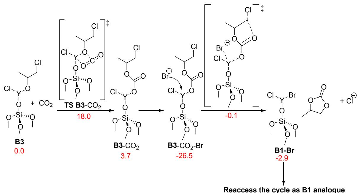
**Scheme S1.** Alternative mechanism for the formation of cyclic carbonate from **B3** with formation of **B1-Br** as surface complex. The values in red refer to calculated Gibbs free energies (kcal/mol) of intermediates and transition states (in square brackets) relative to **B3**.
