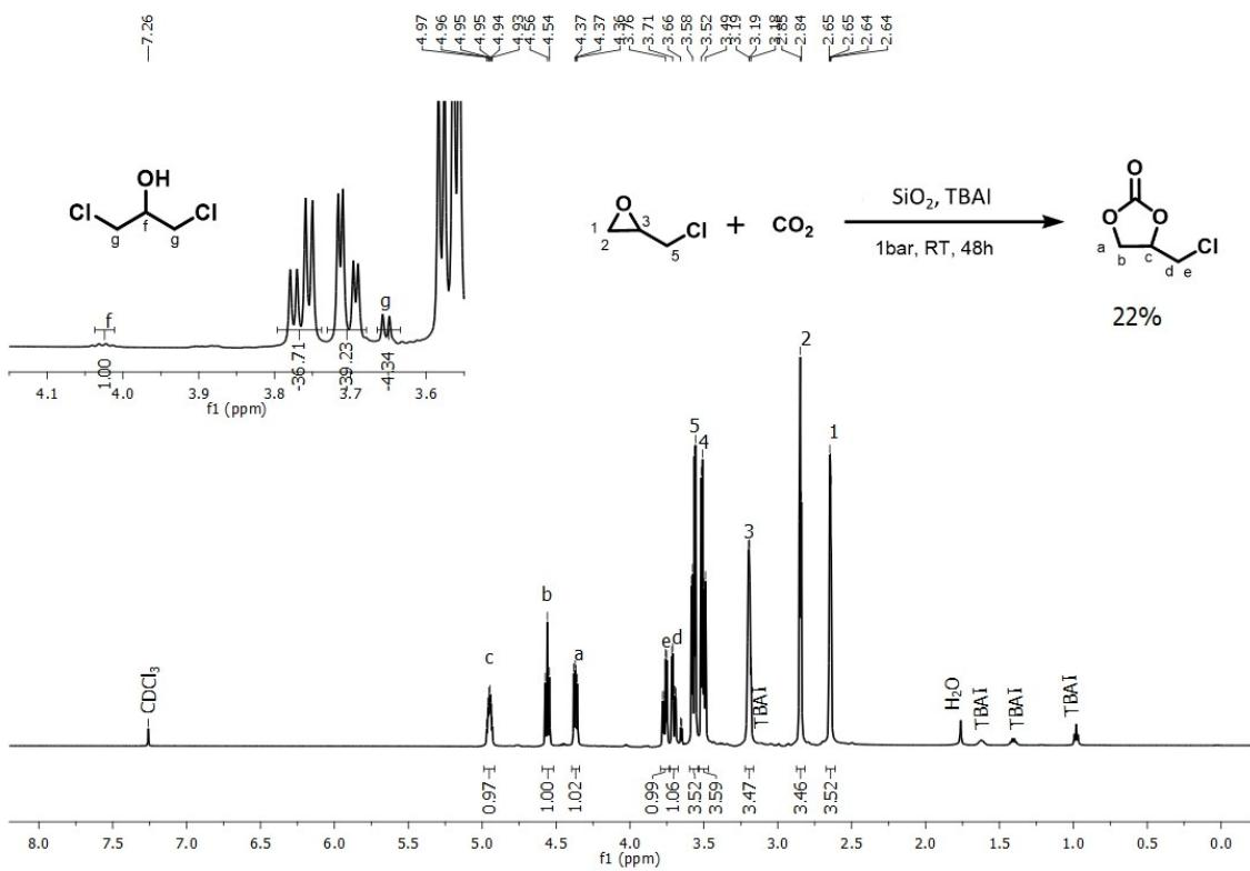
**Figure S39.** Crude  $^1\text{H}$ -NMR spectra of cycloaddition of  $\text{CO}_2$  to Epichlorohydrin by using tt- $\text{SiO}_2$  with TBAI at room temperature for 48 h (Table 3, Entry 20).
