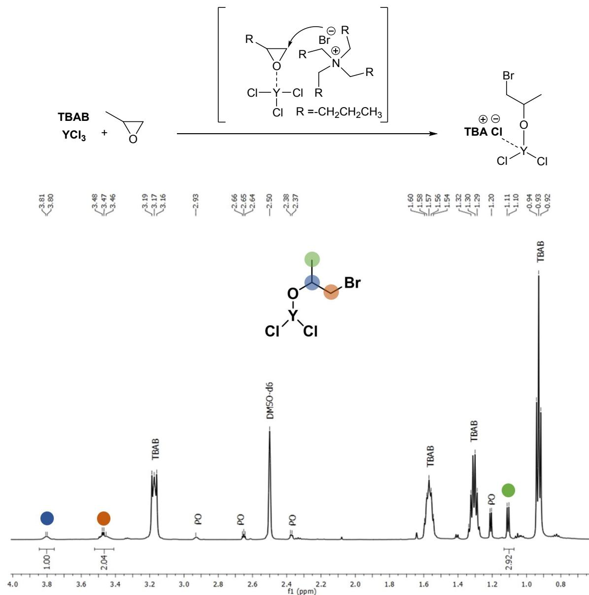
**Figure S1.**  $^1\text{H}$  NMR spectrum of I in  $\text{DMSO-d}_6$ . The protons of the opened epoxide ring are color-coded as shown in the structure in the inset.
