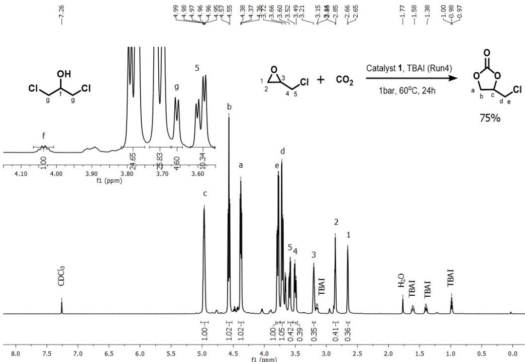
**Figure S22.** Crude <sup>1</sup>H-NMR spectra of cycloaddition of CO<sub>2</sub> to Epichlorohydrin by using catalyst **1** with TBAI (Run 4, Table 3, Entry 5).
