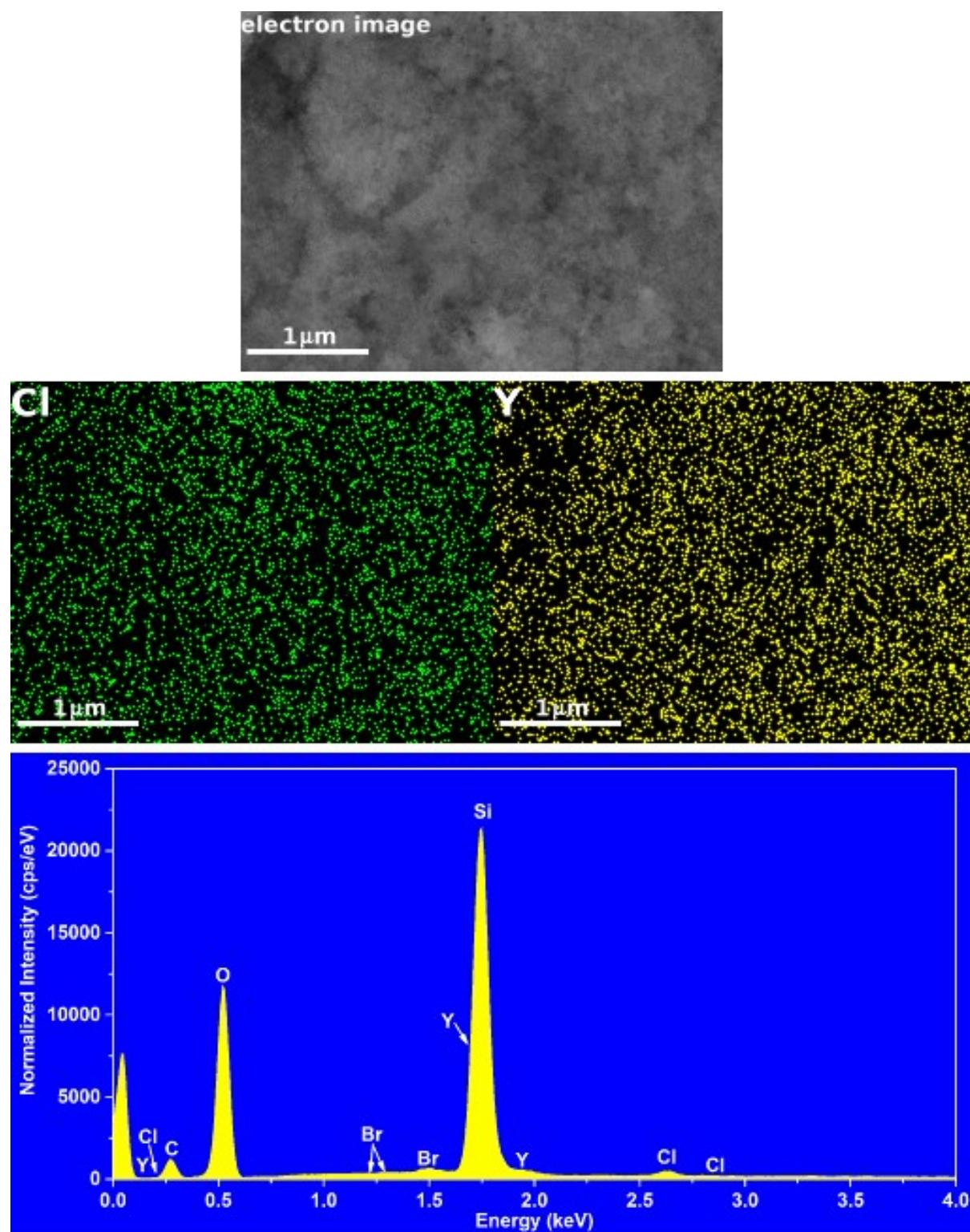
**Figure S11.** (top) electron image, (center) Y and Cl EDS mappings and (bottom) EDS Spectrum of **1**.
