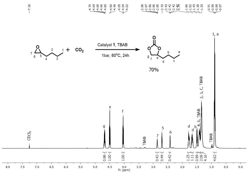
**Figure S17.** Crude  $^1\text{H}$ -NMR spectra of cycloaddition of  $\text{CO}_2$  to 1,2-Epoxyhexane by using catalyst **1** with TBAB (Table 3, Entry 3).
