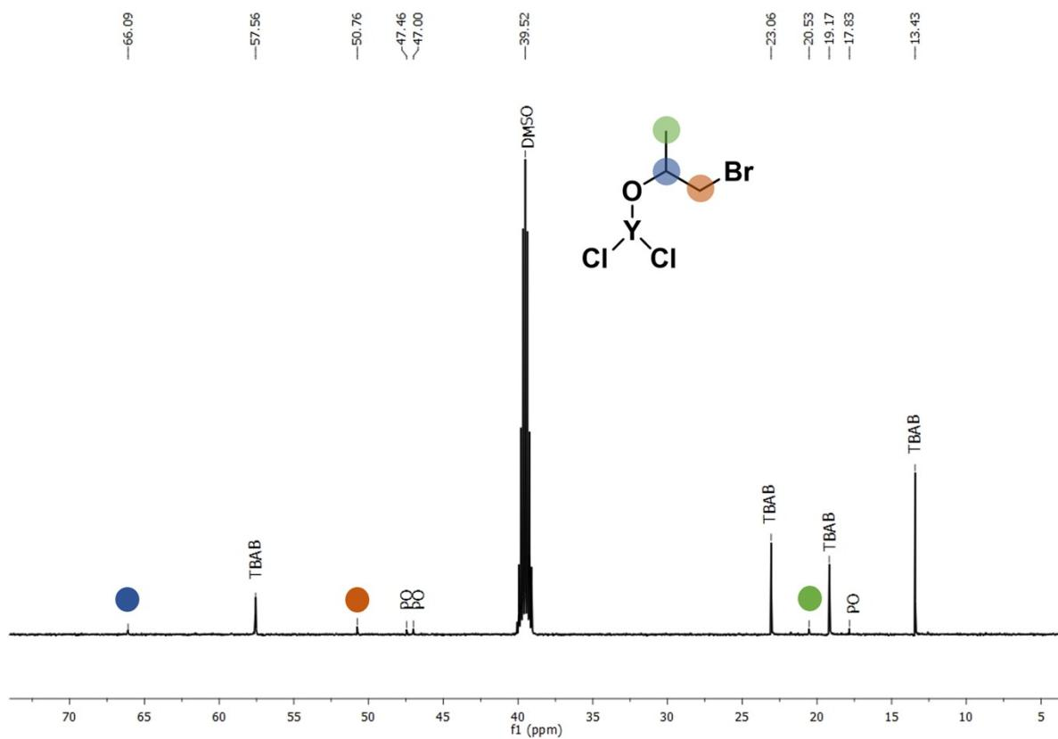
**Figure S2.**  $^{13}\text{C}$  NMR spectrum of **I** in  $\text{DMSO-d}_6$ . The carbon atoms of the opened epoxide ring are color-coded as shown in the structure in the inset.
