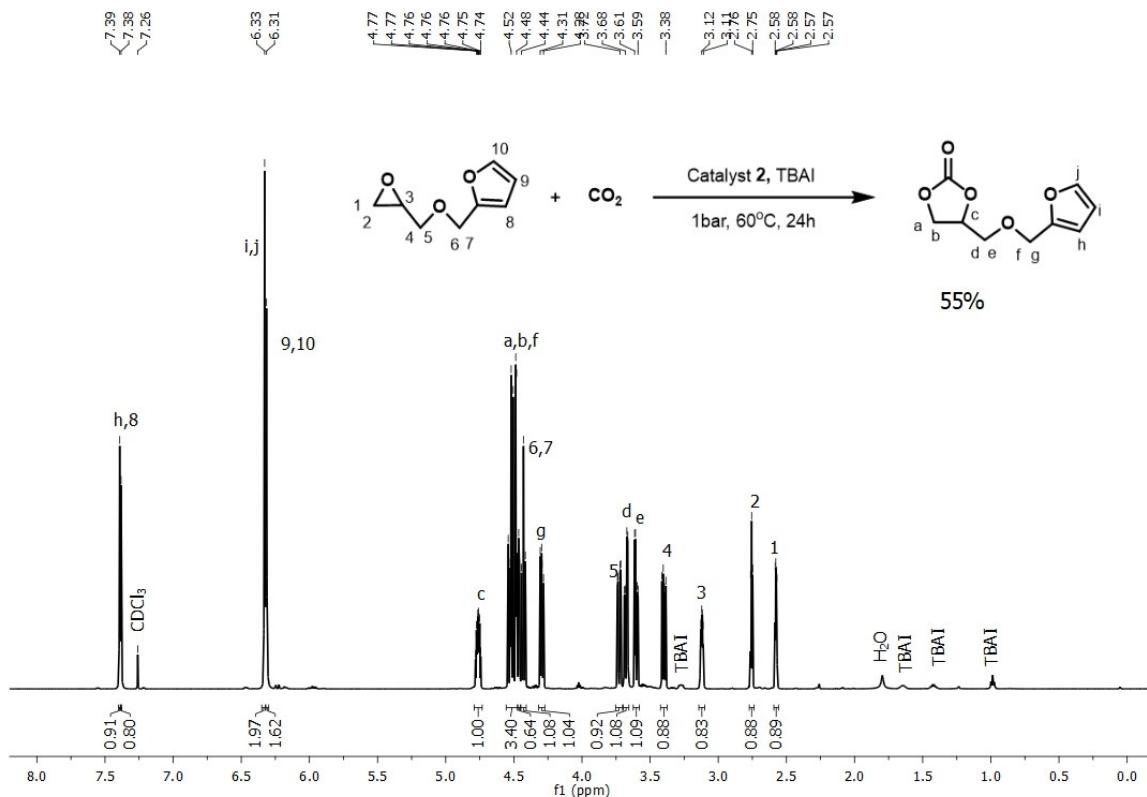
**Figure S34.** Crude <sup>1</sup>H-NMR spectra of cycloaddition of CO<sub>2</sub> to furfuryl glycidyl ether (**5h**) by using catalyst **2** with TBAI at 60°C for 24 h (Table 3, Entry 14).
