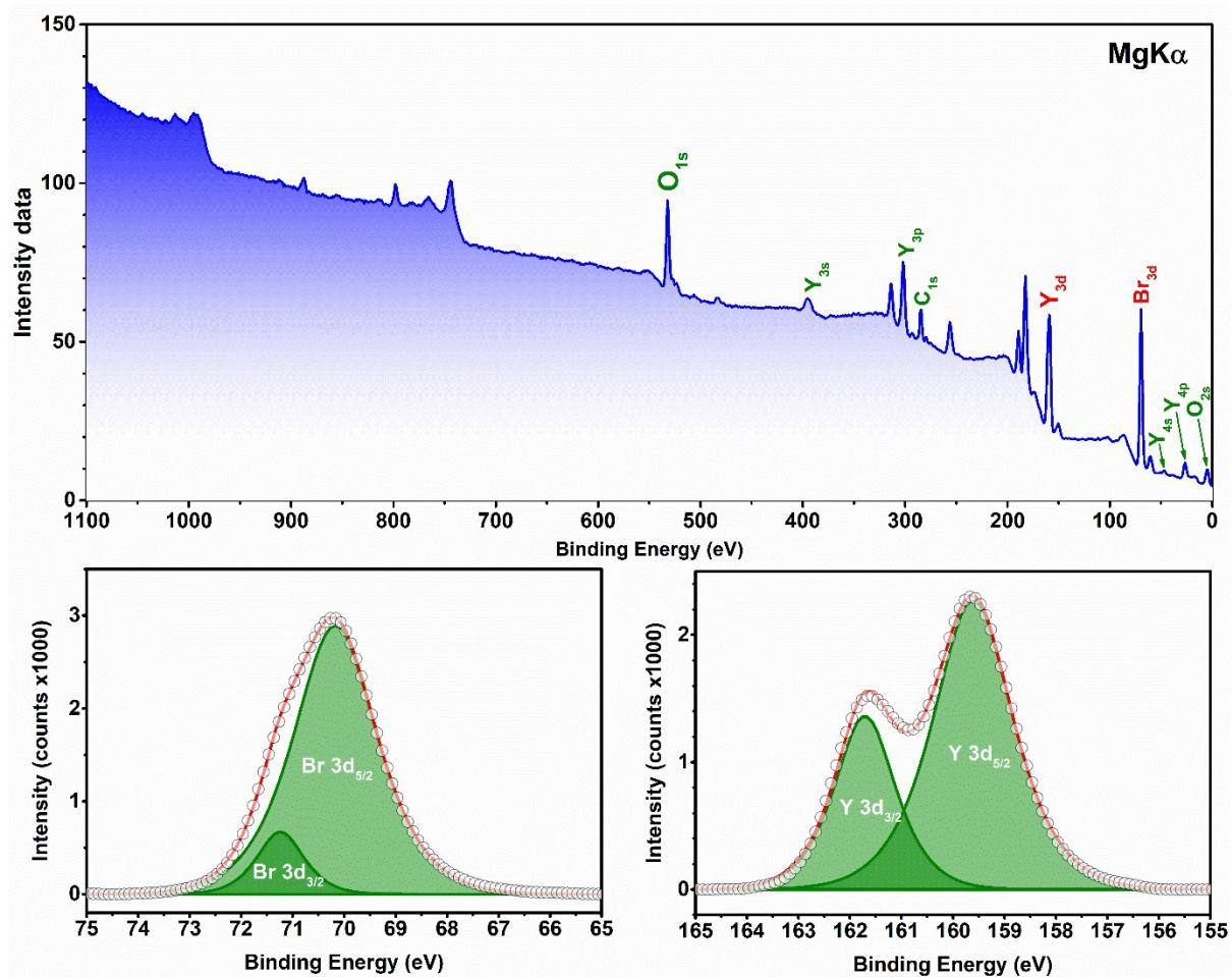
**Figure S9.** Survey (top) and excerpts of high-resolution XPS spectrum (bottom) of anhydrous YBr<sub>3</sub>.
