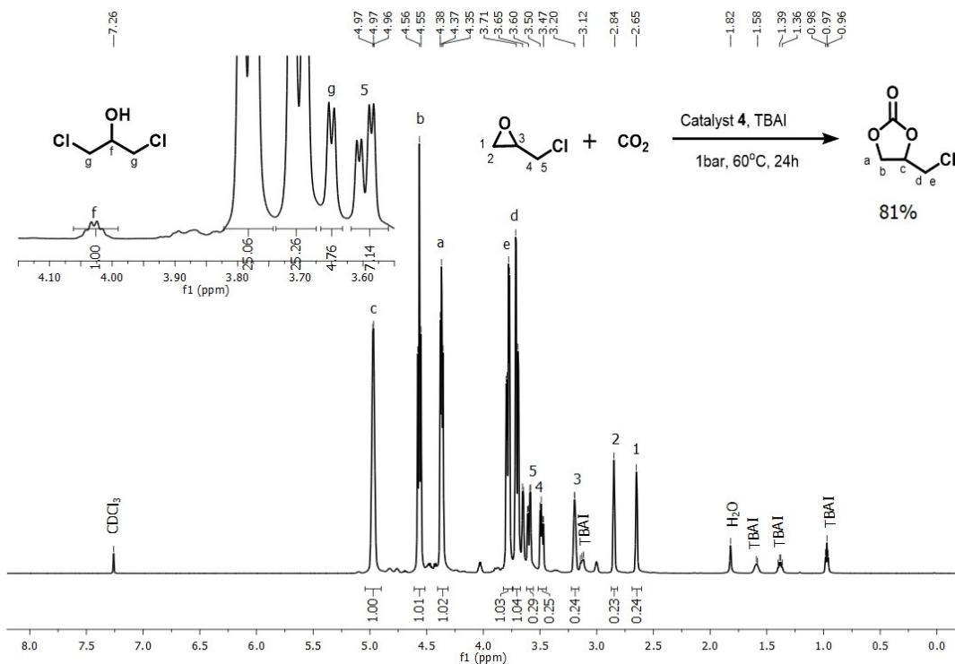
**Figure S31.** Crude <sup>1</sup>H-NMR spectra of cycloaddition of CO<sub>2</sub> to Epichlorohydrin by using catalyst **4** with TBAI (Table 3, Entry 11).
