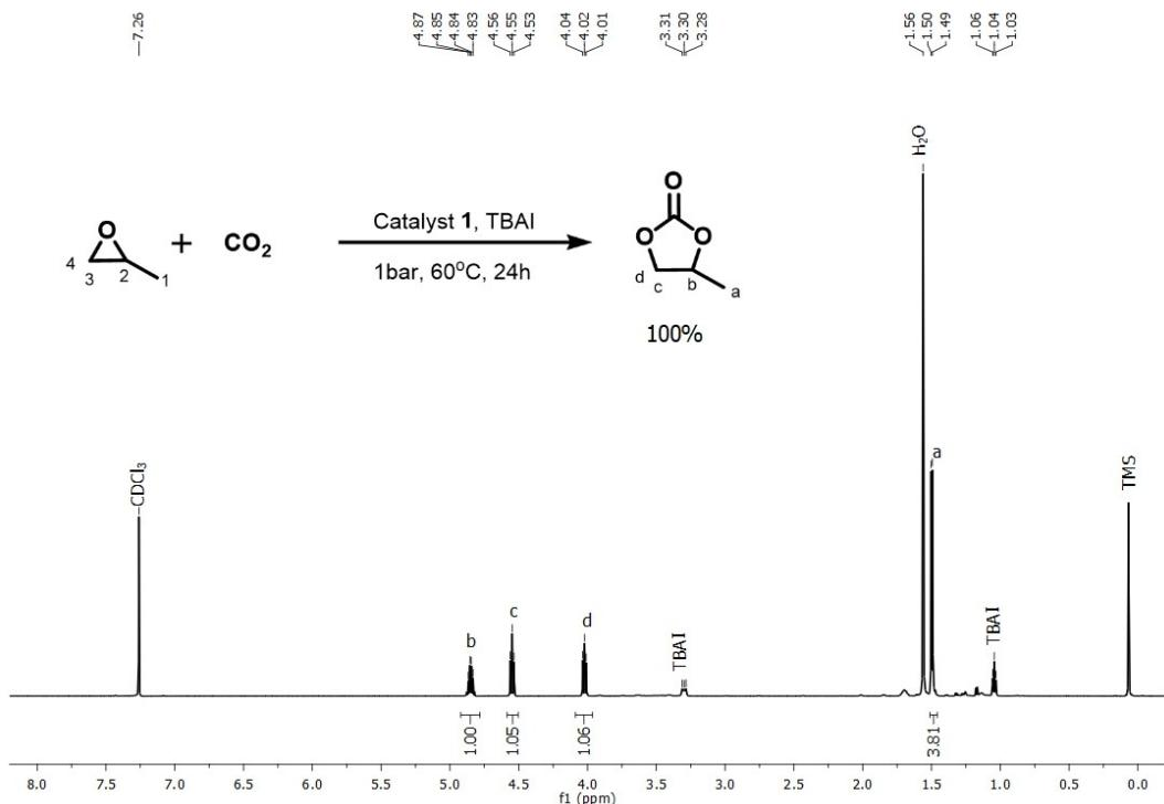
**Figure S18.** Crude  $^1\text{H}$ -NMR spectra of cycloaddition of  $\text{CO}_2$  to Propylene oxide by using catalyst **1** with TBAI. The  $\text{CDCl}_3$  solvent used for this spectrum contains water and TMS as standards (Table 3, Entry 4).
