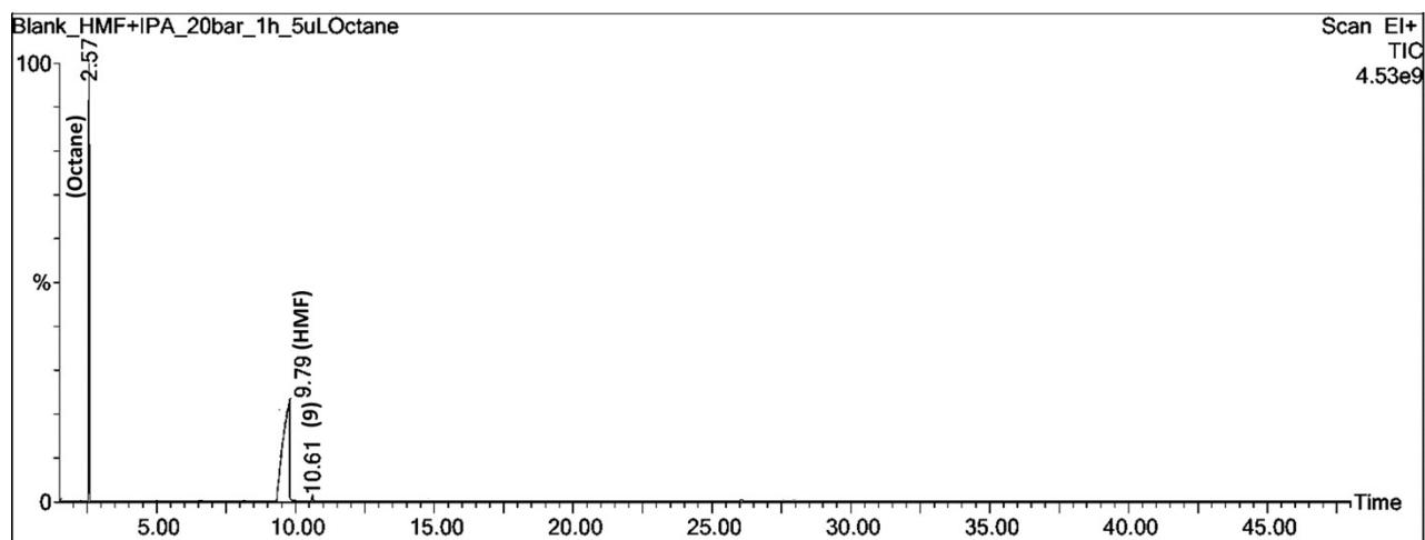
**Figure S41.** Chromatogram of reductive etherification of HMF without catalyst (blank reaction) at 150 °C, 20 bar N<sub>2</sub> for 1 h (Table S5, Entry 1).
