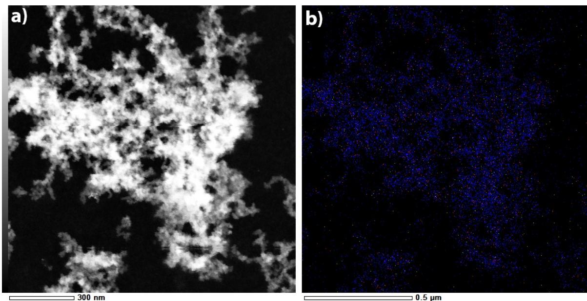
**Figure S14.** a) ADF-TEM image and b) EDS mapping (Si (blue), Y (red) and Cl (green)) of material **2** after three catalytic cycles.
