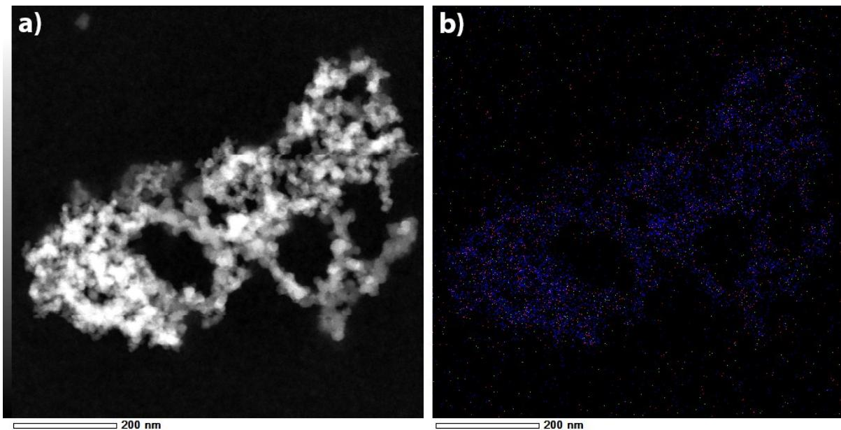
**Figure S13.** a) ADF-TEM image and b) EDS mapping (Si (blue), Y (red) and Cl (green)) of material **2**.
