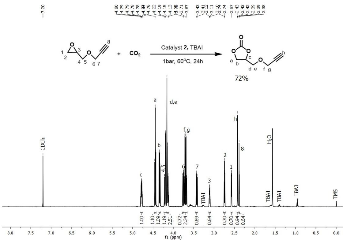
**Figure S33.** Crude <sup>1</sup>H-NMR spectra of cycloaddition of CO<sub>2</sub> to glycidyl propargyl ether (**5g**) by using catalyst **2** with TBAI at 60°C for 24 h (Table 3, Entry 13).
