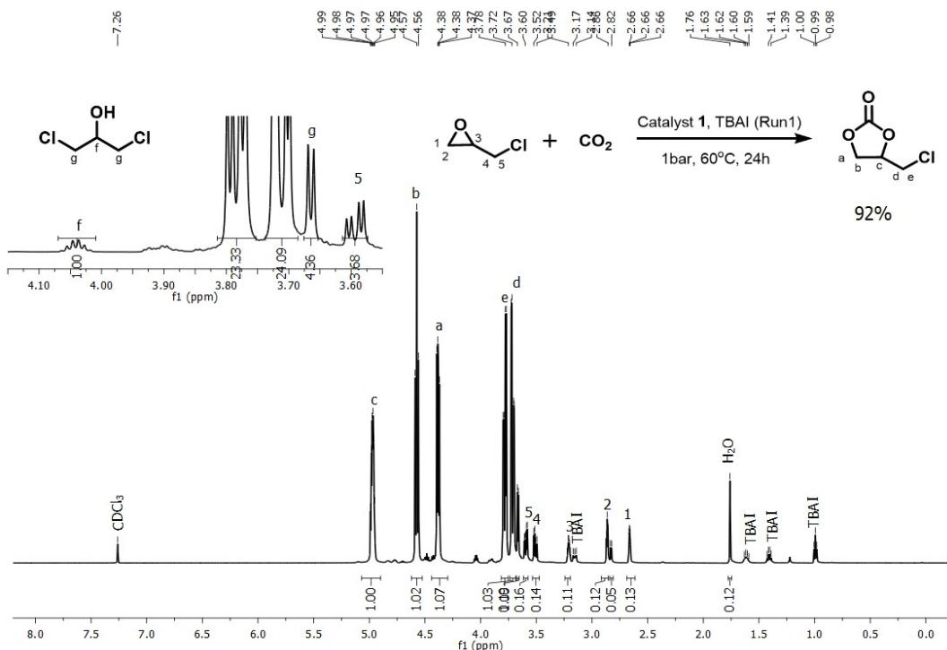
**Figure S19.** Crude <sup>1</sup>H-NMR spectra of cycloaddition of CO<sub>2</sub> to Epichlorohydrin by using catalyst **1** with TBAI (Run 1, Table 3, Entry 5).
