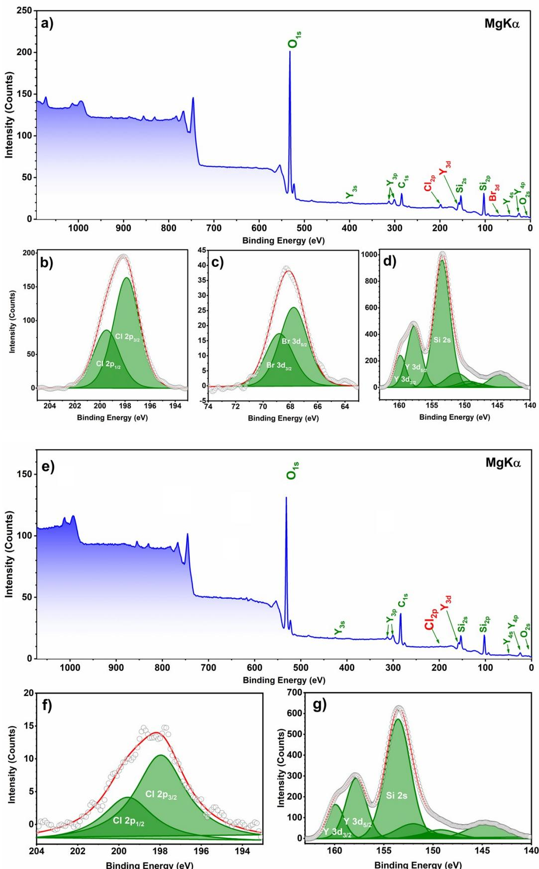
**Figure S7.** Surveys (a, e) and excerpts (b, c, d, f, g) of the high-resolution XPS spectra of pristine **2** (a-d) and recovered **2** (e-g) after three catalytic cycles.
