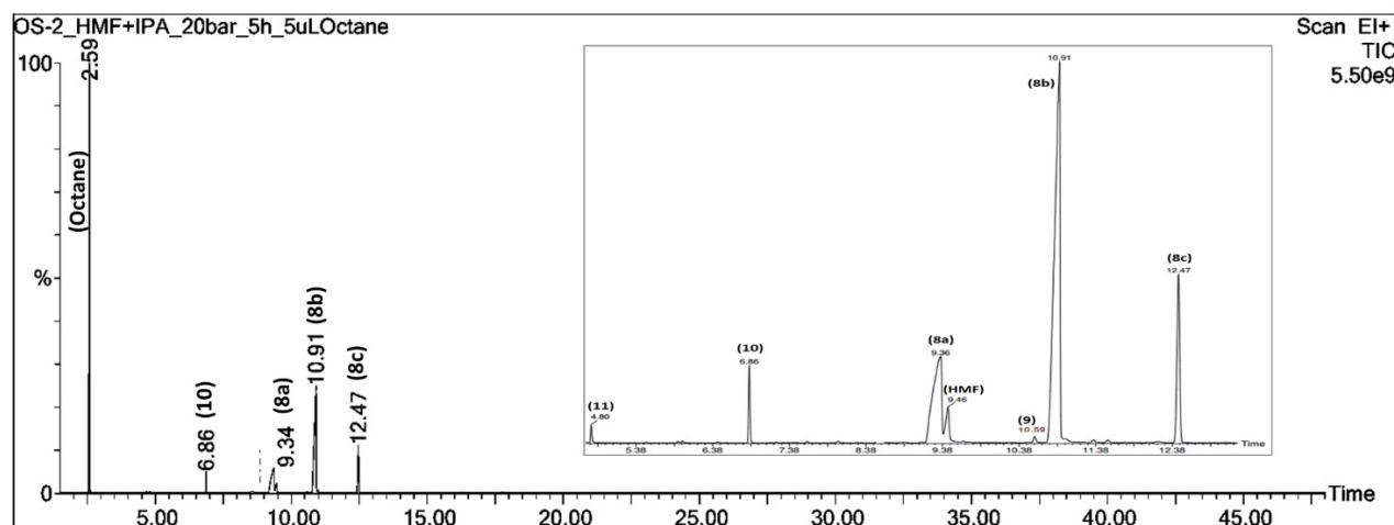
**Figure S44.** Chromatogram of reductive etherification of HMF catalyzed by **2** at 150 °C, 20 bar N<sub>2</sub> for 5 h (Table S5, Entry 5).
