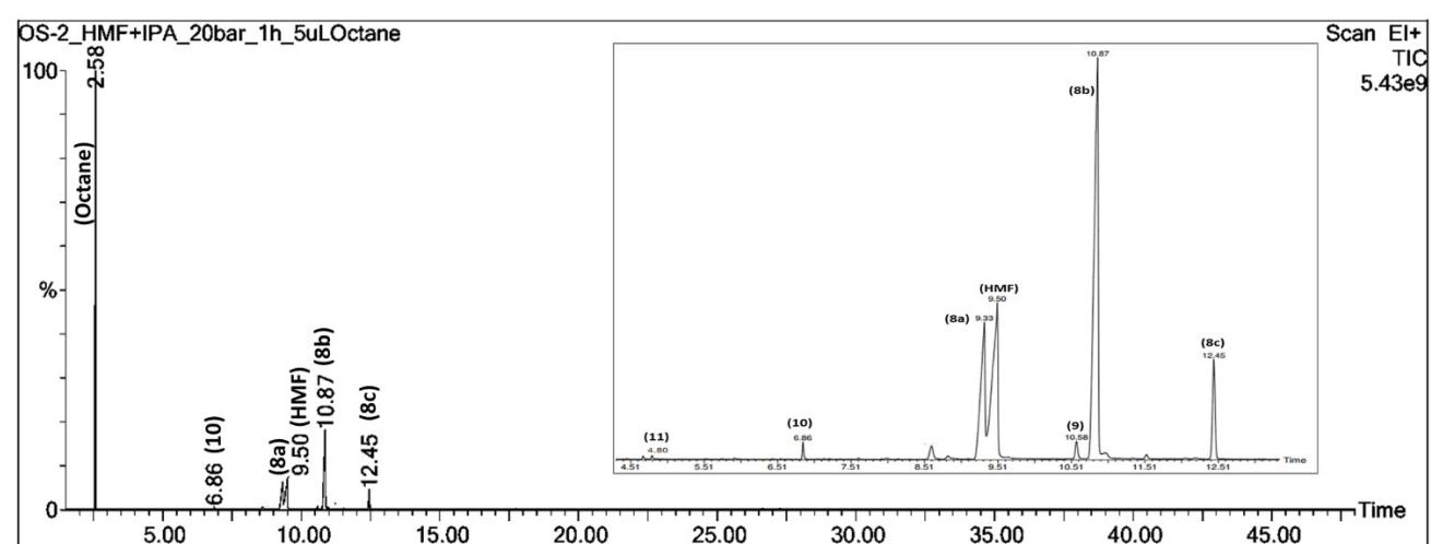
**Figure S43.** Chromatogram of reductive etherification of HMF catalyzed by **2** at 150 °C, 20 bar N<sub>2</sub> for 1 h (Table S5, Entry 4).
