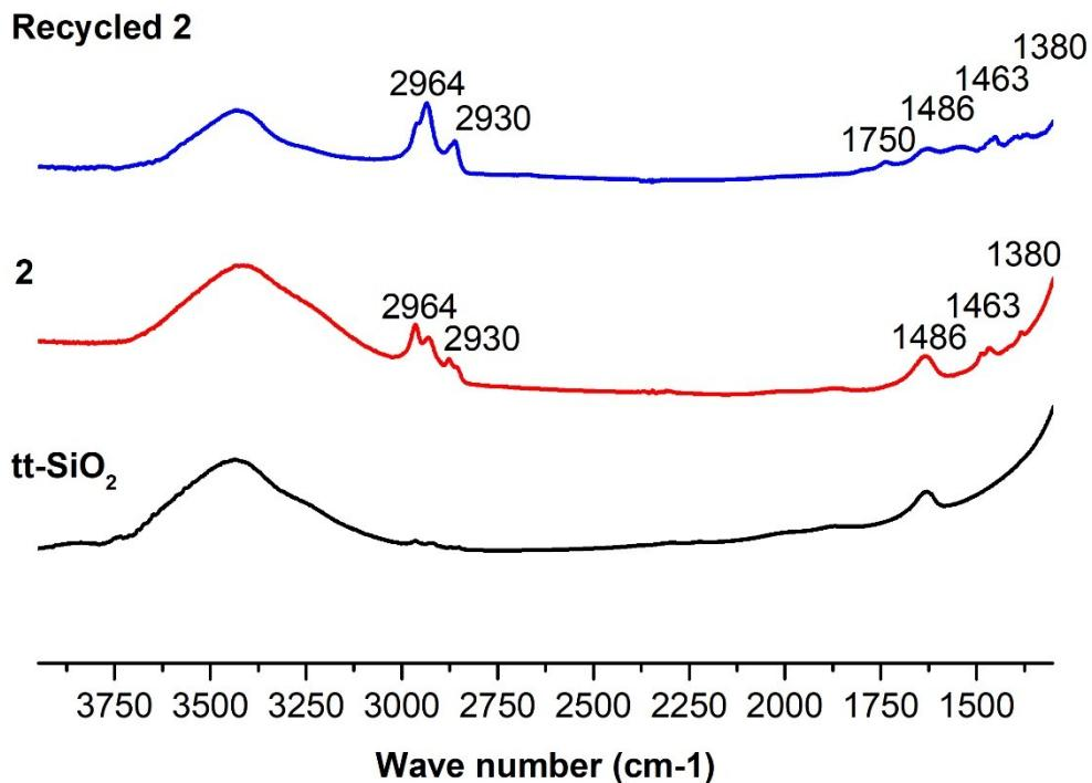
**Figure S4.** FT-IR spectra of tt-SiO<sub>2</sub> (black trace, bottom), material **2** (red trace, middle) and material **2** after three catalytic cycles (top).
