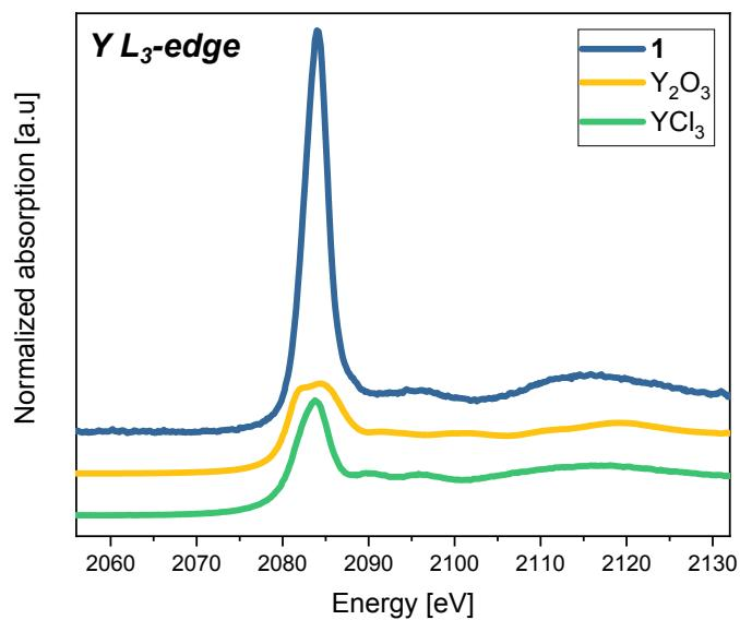
**Figure S10:** XANES spectra measured at the Y  $L_3$ -edge for compound **1** with  $\text{Y}_2\text{O}_3$  and  $\text{YCl}_3$  references. The spectra have been normalized and shifted for the sake of clarity.
