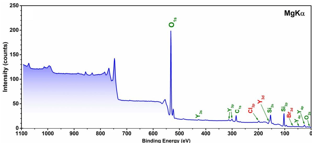
**Figure S6.** Survey XPS spectrum of **1**. For high-resolution spectra see Figure 3 of the manuscript.
