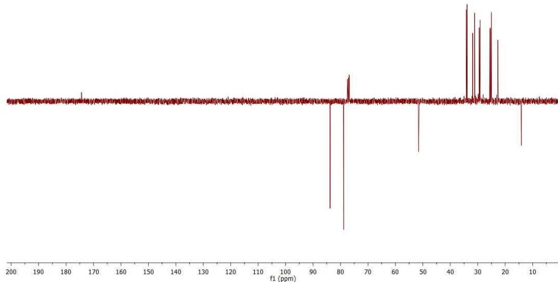
**$^{13}\text{C-NMR (APT)}$**  ( $\text{CDCl}_3$ ,  $\delta$  ppm, 100 MHz): 174.3, 83.8, 83.7, 78.86, 78.85, 51.5, 34.1, 33.89, 33.88, 31.84, 31.14, 29.8, 29.4, 29.2, 29.1, 28.0, 25.5, 25.3, 25.0, 23.1, 22.6, 14.1.
