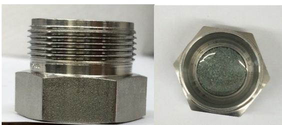
**Figure S1.** Experimental set up and photo of the mixed state of catalyst and feed (cap diameter: 3/4 inch, 0.2 g catalyst, 0.4 g guaiacol)
