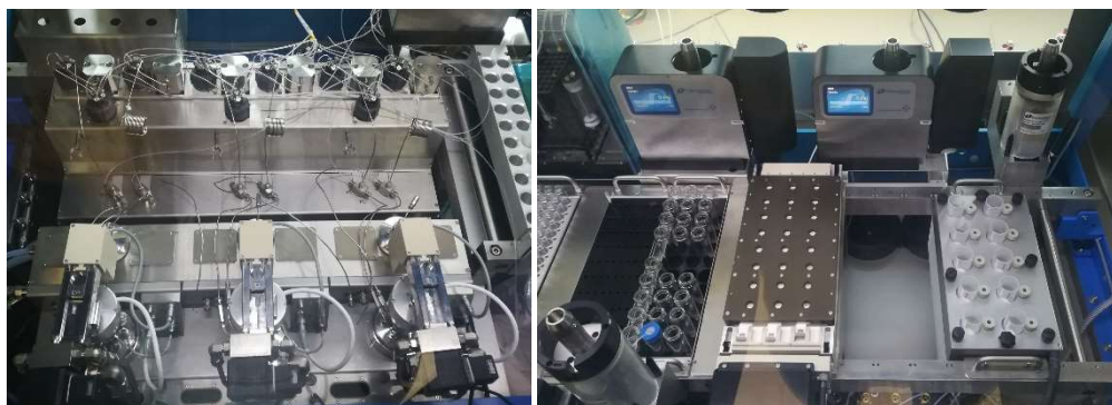
Figure S4. Automated Chemspeed platform equipped with three semi-batch reactors (left) and ISYNTH ® module (right)
