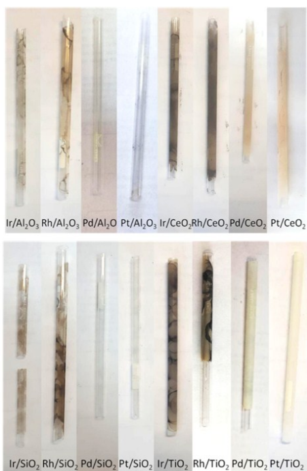
Figure S1. Photographs of reactors with catalytic coatings (16 compositions) after heterogeneous catalytic hydrogenations of 1,3-butadiene.
