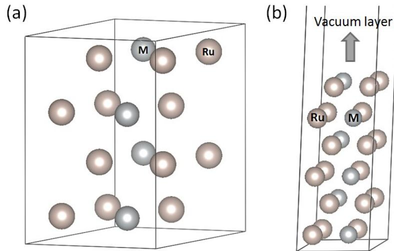
**Figure S1.** (a) Extended HCP-Ru<sub>3</sub>-M<sub>1</sub> bulk model and (b) Ru<sub>3</sub>-M<sub>1</sub> (0001) surface model, where Ru and M atoms are indicated.
