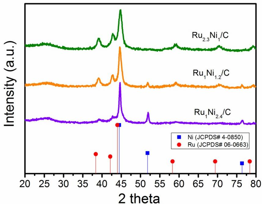
**Figure S9.** XRD patterns of Ru<sub>2.3</sub>Ni<sub>1</sub>/C, Ru<sub>1</sub>Ni<sub>1.2</sub>/C and Ru<sub>1</sub>Ni<sub>2.4</sub>/C nanocatalysts.
