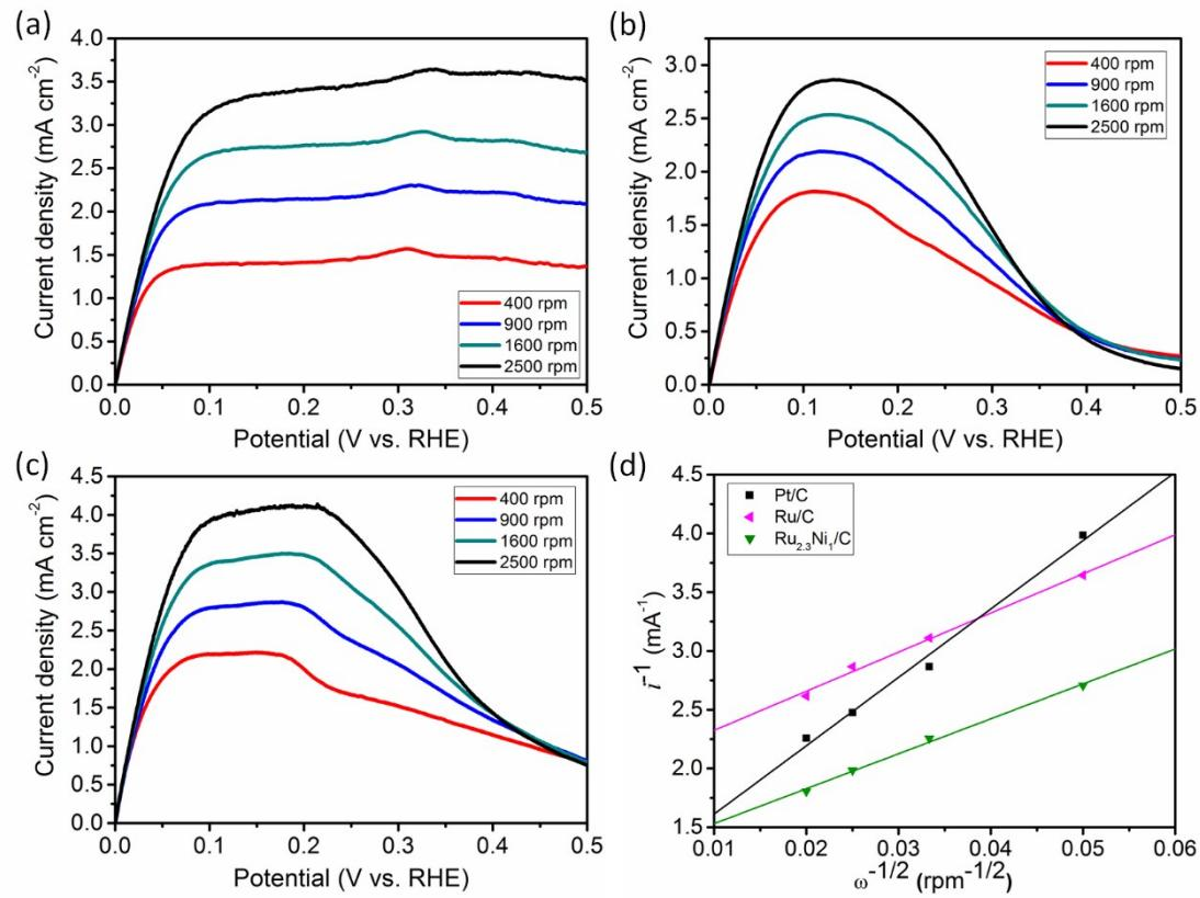
**Figure S7.** Rotating-disk voltammograms of: (a) Pt/C, (b) Ru/C and (c) Ru<sub>2.3</sub>Ni<sub>1</sub>/C in H<sub>2</sub>-saturated 0.1 M KOH at 10 mV s<sup>-1</sup>. (d) Koutechy-Levich plots of the different catalysts.
