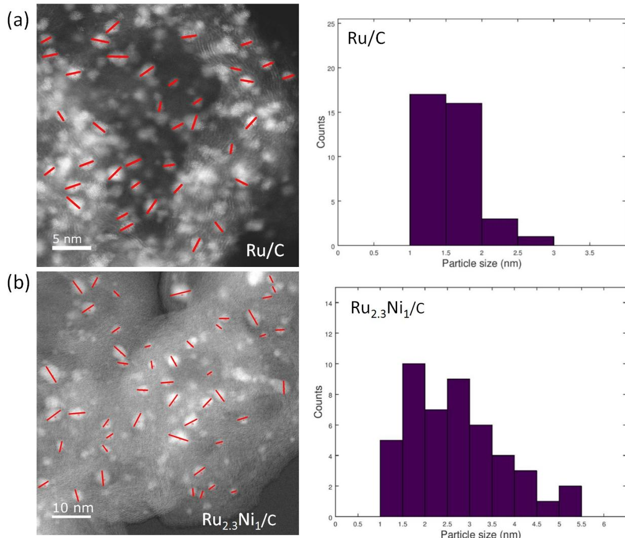
**Figure S2.** STEM images of: (a) Ru/C and (b)  $\text{Ru}_{2.3}\text{Ni}_1/\text{C}$  and the corresponding particle size distribution.
