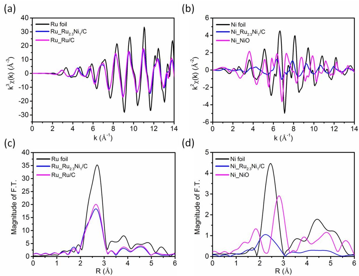
**Figure S10.**  $k$ -space and  $r$ -space of (a, c) Ru K-edge and (b, d) Ni K-edge for the Ru<sub>2.3</sub>Ni<sub>1</sub>/C catalyst.
