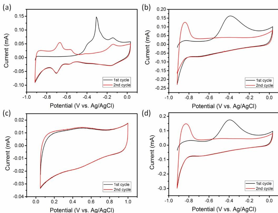
**Figure S8.** CO stripping voltammograms of: (a) Pt/C, (b) Ru/C, (c) Ni/C and (d) Ru<sub>2.3</sub>Ni<sub>1</sub>/C in CO-saturated 0.1 M KOH at 10 mV s<sup>-1</sup>.
