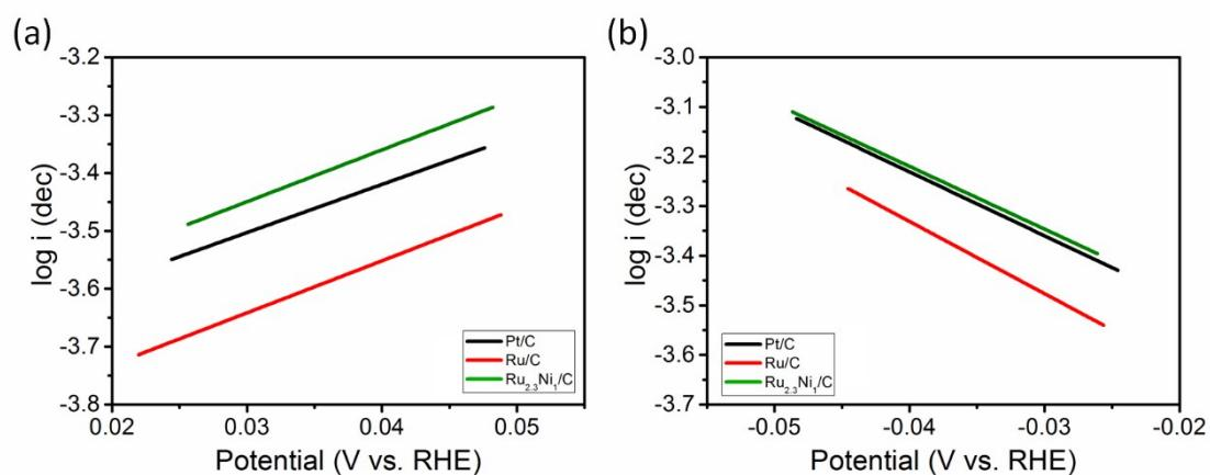
**Figure S6.** Tafel plots of Pt/C, Ru/C and  $\text{Ru}_{2.3}\text{Ni}_1/\text{C}$  in alkaline (a) HOR and (b) HER.
