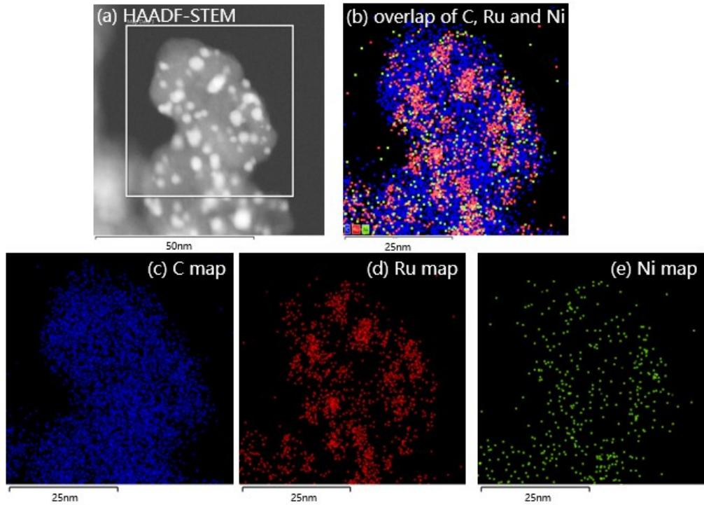
**Figure S3.** STEM-EDS elemental maps of the  $\text{Ru}_{2.3}\text{Ni}_1/\text{C}$  catalyst. (a) HAADF-STEM image, (b) overlap of C, Ru and Ni elemental map signals, (c) C elemental map signals, (d) Ru elemental map signals, and (e) Ni elemental map signals.
