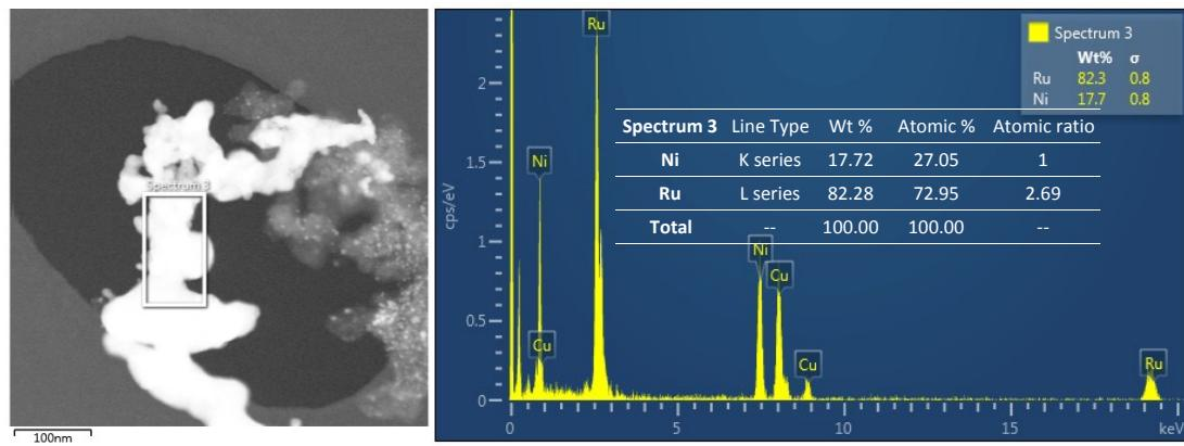
**Figure S4** (a) STEM image and (b) EDS analysis of synthesized RuNi NPs.
