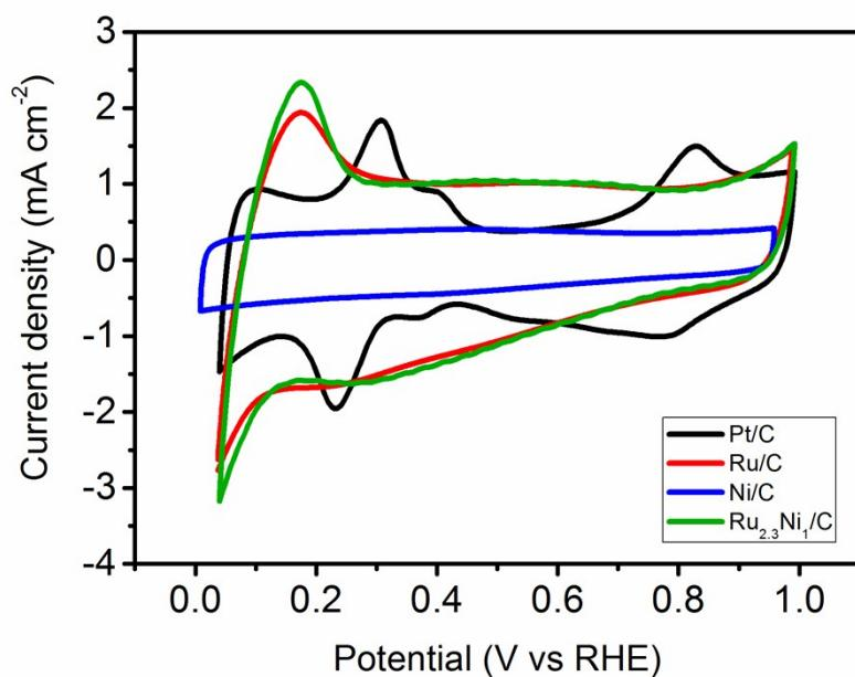
**Figure S5** Cyclic voltammetric curve of Pt/C, Ru/C, Ni/C and  $\text{Ru}_{2.3}\text{Ni}_1/\text{C}$  in Ar-saturated 0.1 M KOH at  $50 \text{ mV s}^{-1}$ .
