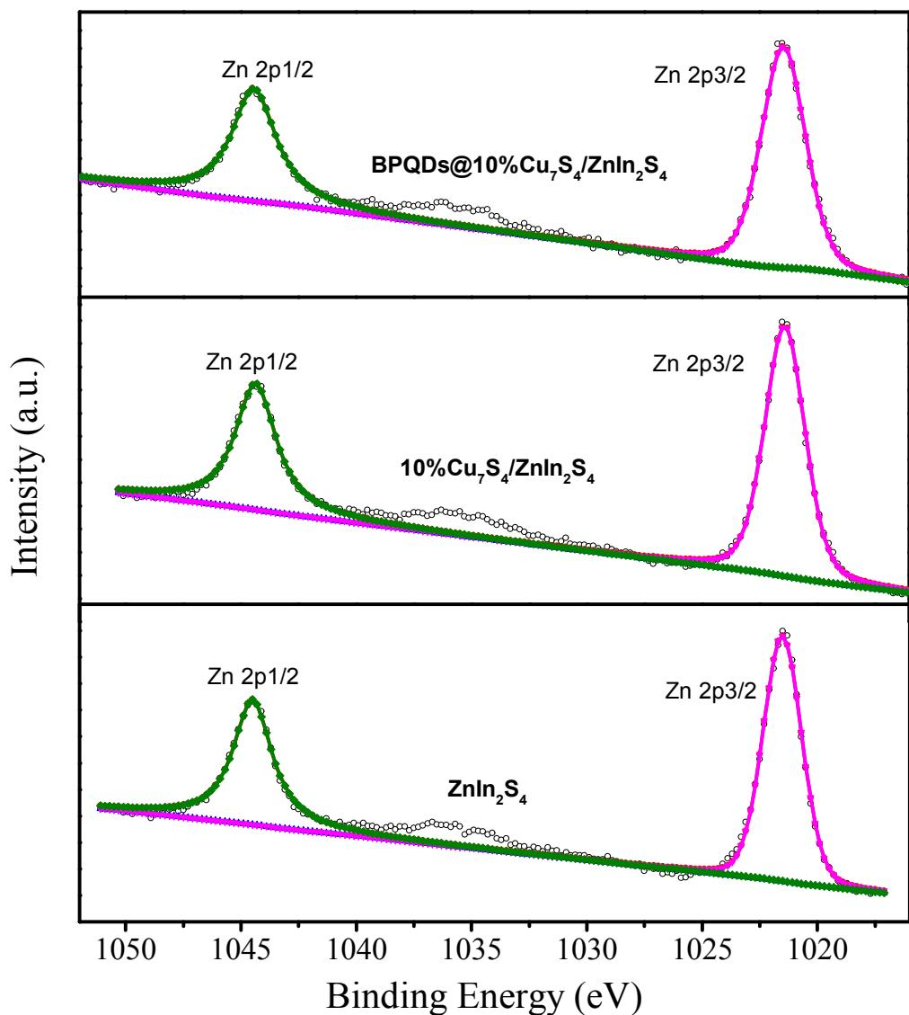
**Fig. S12.** Zn high-resolution XPS spectra of  $\text{ZnIn}_2\text{S}_4$ , 10% $\text{Cu}_7\text{S}_4/\text{ZnIn}_2\text{S}_4$  and BPQDs@10% $\text{Cu}_7\text{S}_4/\text{ZnIn}_2\text{S}_4$  samples.
