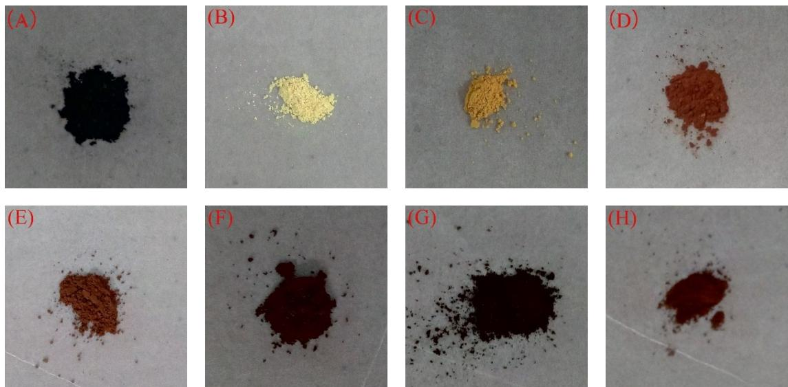
**Fig. S8.** Appearance color contrast of (A)  $\text{Cu}_7\text{S}_4$ , (B)  $\text{ZnIn}_2\text{S}_4$ , (C) 1% $\text{Cu}_7\text{S}_4/\text{ZnIn}_2\text{S}_4$ , (D) 5% $\text{Cu}_7\text{S}_4/\text{ZnIn}_2\text{S}_4$ , (E) 10% $\text{Cu}_7\text{S}_4/\text{ZnIn}_2\text{S}_4$ , (F) 20% $\text{Cu}_7\text{S}_4/\text{ZnIn}_2\text{S}_4$ , (G) 30% $\text{Cu}_7\text{S}_4/\text{ZnIn}_2\text{S}_4$  and (H) BPQDs@10% $\text{Cu}_7\text{S}_4/\text{ZnIn}_2\text{S}_4$  composites.
