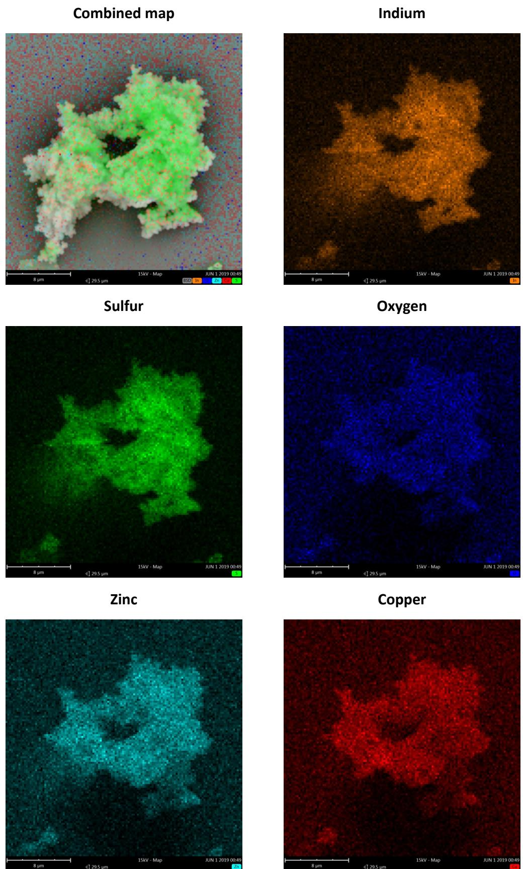
**Fig. S3.** EDS mapping profiles of 30% $\text{Cu}_7\text{S}_4/\text{ZnIn}_2\text{S}_4$  samples.
