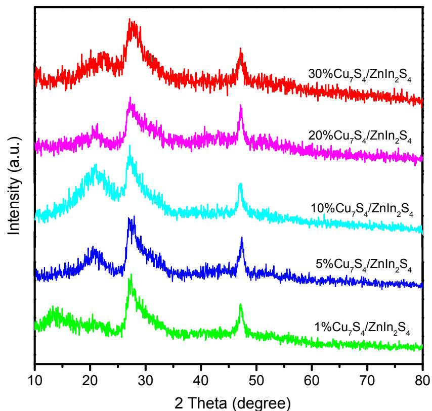
**Fig. S7.** XRD patterns of different contents of  $\text{Cu}_7\text{S}_4/\text{ZnIn}_2\text{S}_4$  samples.
