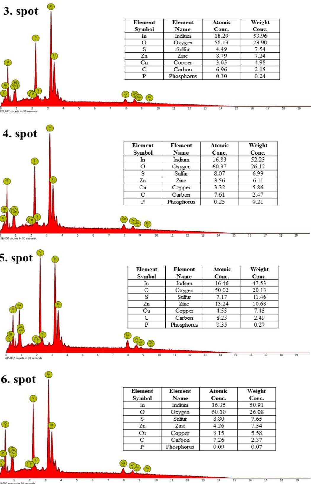
**Fig. S5.** Quantitative results of BPQDs@Cu<sub>7</sub>S<sub>4</sub>/ZnIn<sub>2</sub>S<sub>4</sub> through random selection of 6 points by tabletting method.
