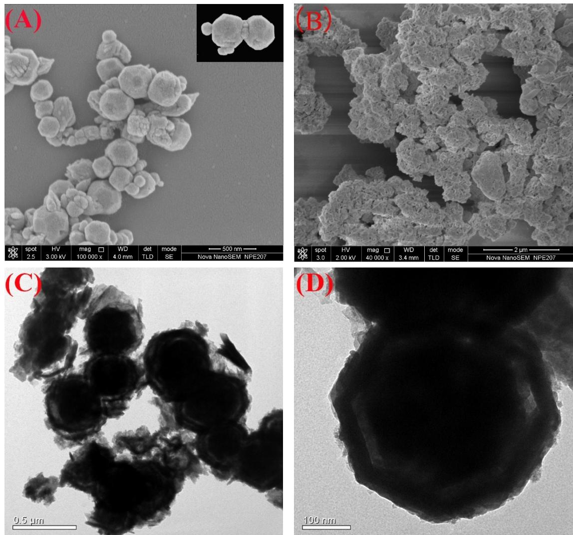
**Fig. S1.** FESEM images of (A)  $\text{Cu}_2\text{O}$ , (B)  $\text{ZnIn}_2\text{S}_4$  and TEM images of (C)  $\text{Cu}_7\text{S}_4$ , (D) enlarged  $\text{Cu}_7\text{S}_4$  samples.
