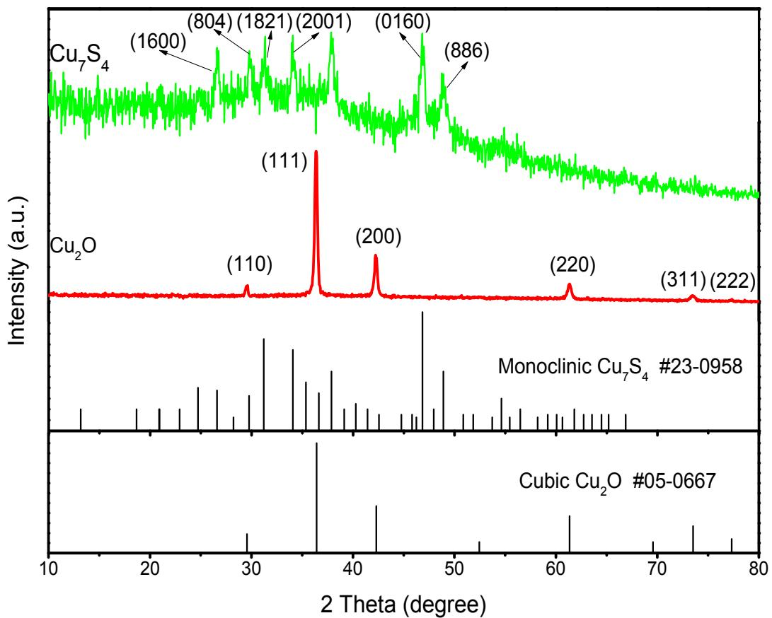
**Fig. S6.** XRD patterns of  $\text{Cu}_2\text{O}$ ,  $\text{Cu}_7\text{S}_4$  samples.
