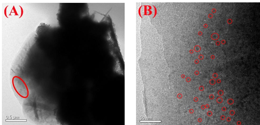
**Fig. S4.** TEM images of the deposition of BPQDs on the surface of  $\text{ZnIn}_2\text{S}_4$ .
