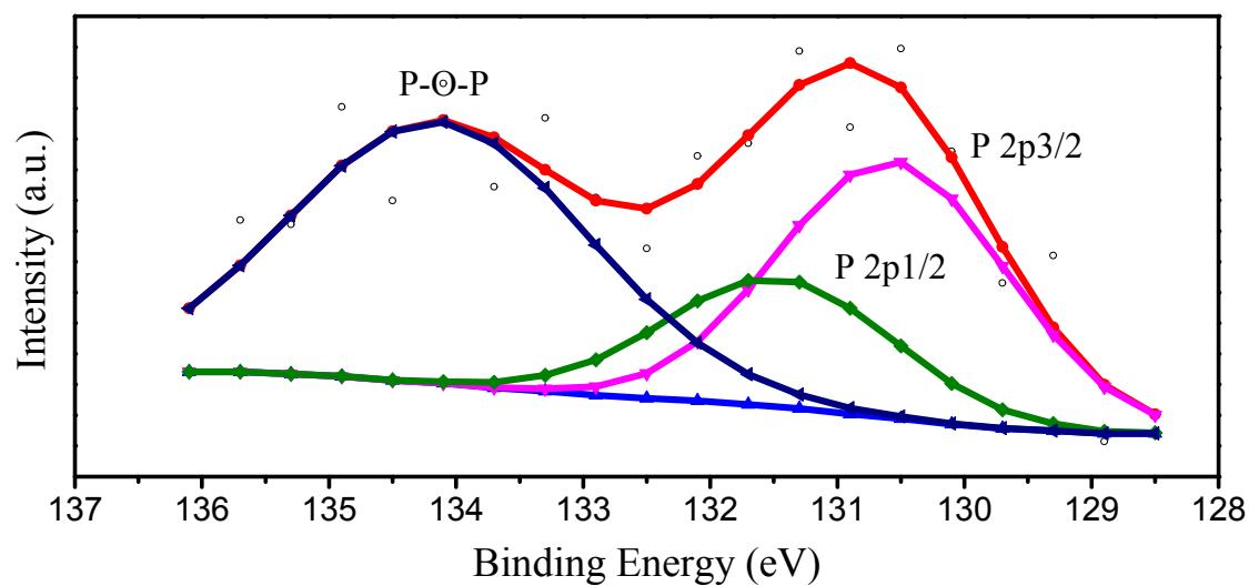
**Fig. S13.** P 2p high-resolution XPS spectra of BPQDs@10%Cu<sub>7</sub>S<sub>4</sub>/ZnIn<sub>2</sub>S<sub>4</sub> samples.
