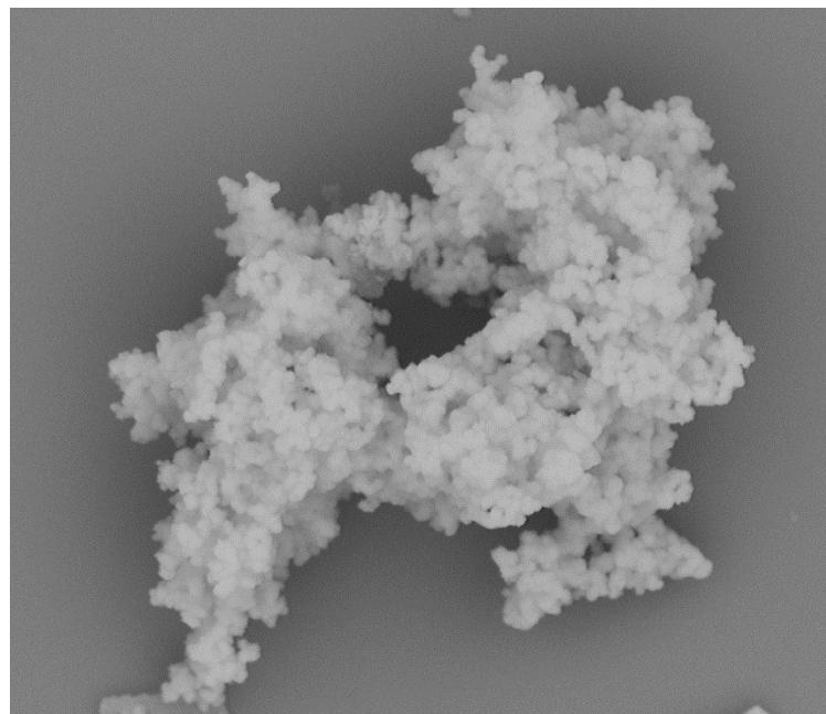
**Fig. S14.** Agglomerated phenomenon of 30% Cu<sub>7</sub>S<sub>4</sub>/ZnIn<sub>2</sub>S<sub>4</sub> samples.
