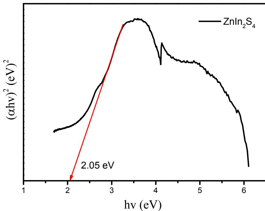
**Fig. S15.** Optical band gaps of pristine  $\text{ZnIn}_2\text{S}_4$  determined by Kubelka-Munk plot.
