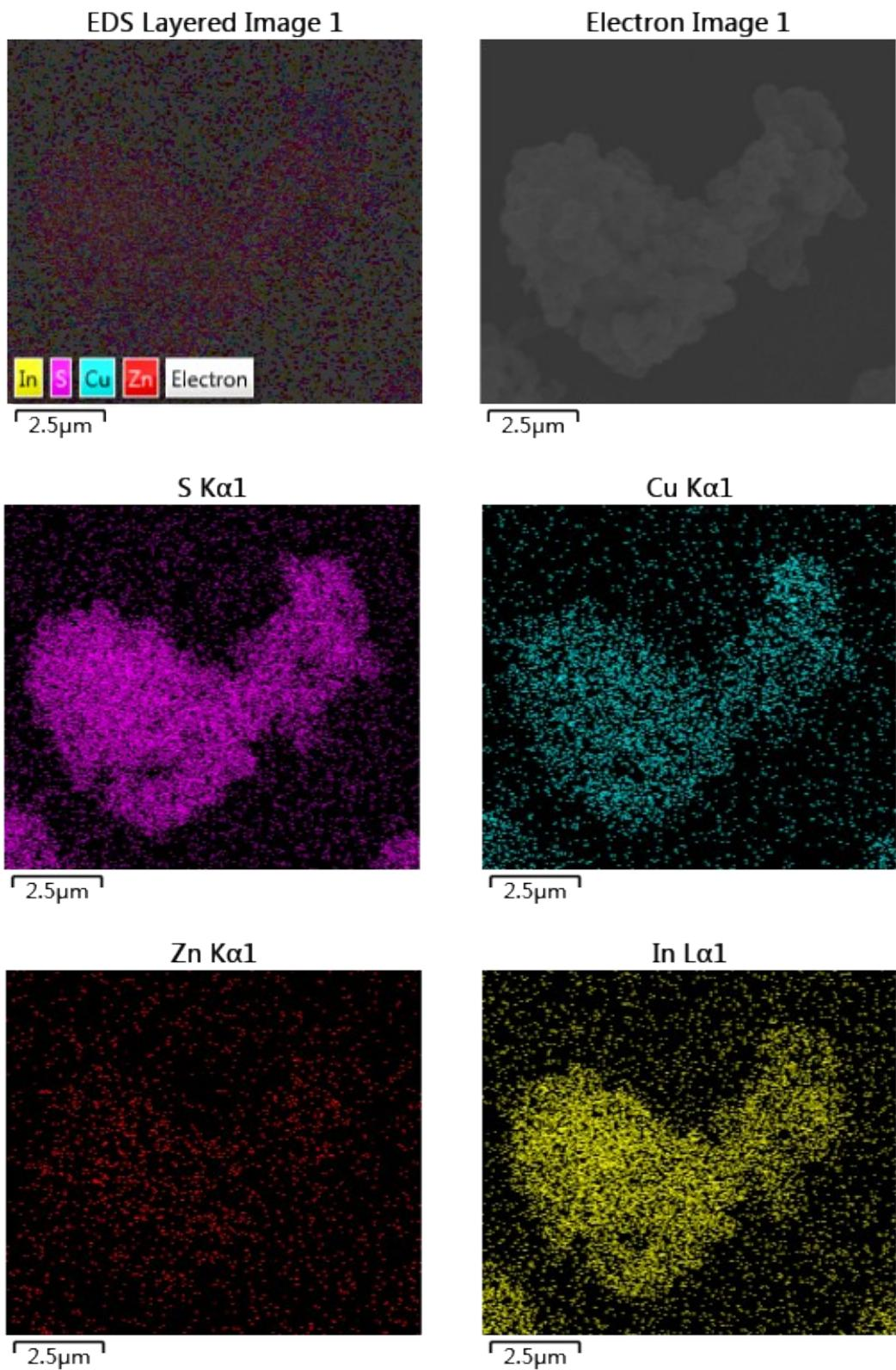
**Fig. S2.** EDS mapping profiles of 20%Cu<sub>7</sub>S<sub>4</sub>/ZnIn<sub>2</sub>S<sub>4</sub> samples.
