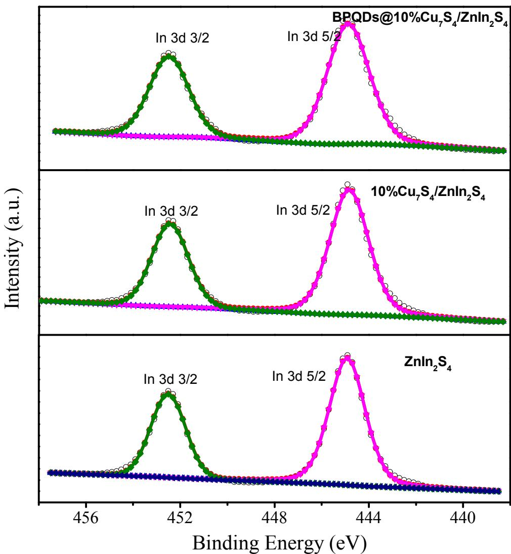
**Fig. S11.** In high-resolution XPS spectra of ZnIn<sub>2</sub>S<sub>4</sub>, 10%Cu<sub>7</sub>S<sub>4</sub>/ZnIn<sub>2</sub>S<sub>4</sub> and BPQDs@10%Cu<sub>7</sub>S<sub>4</sub>/ZnIn<sub>2</sub>S<sub>4</sub> samples.
