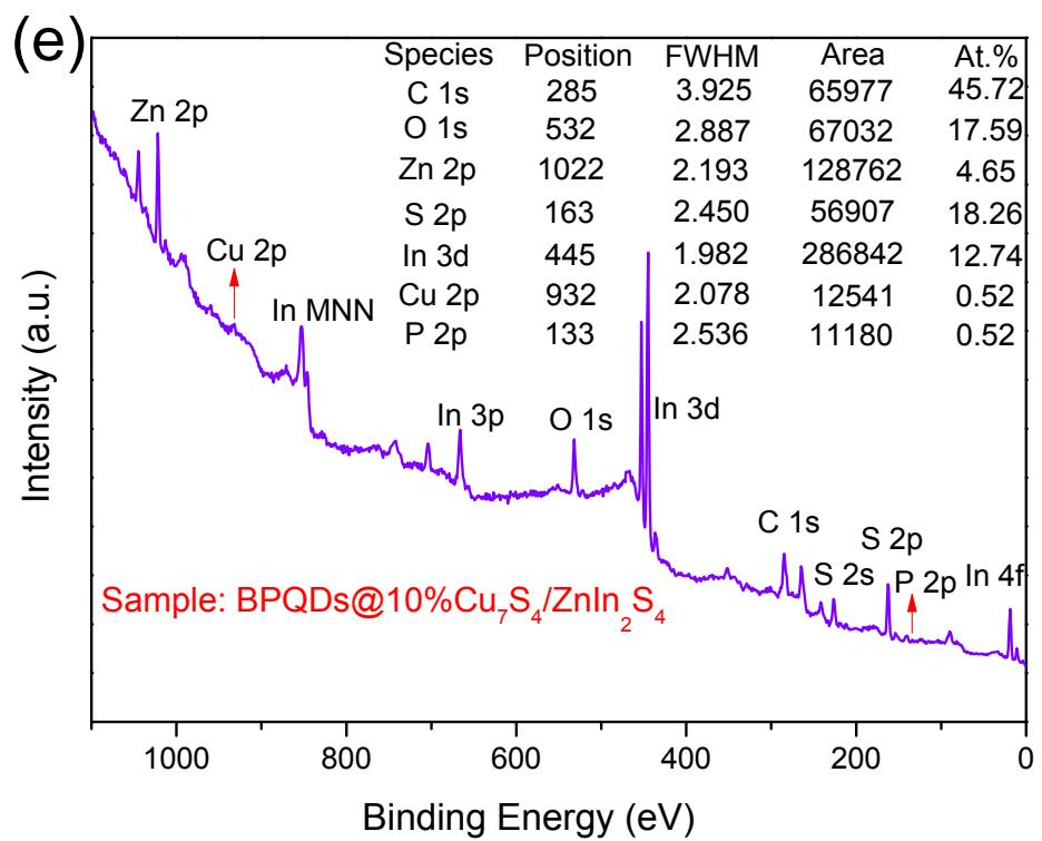
**Fig. S10.** Full-spectrum XPS scan of  $\text{Cu}_2\text{O}$ ,  $\text{Cu}_7\text{S}_4$ ,  $\text{ZnIn}_2\text{S}_4$ , 10% $\text{Cu}_7\text{S}_4/\text{ZnIn}_2\text{S}_4$  and BPQDs@10% $\text{Cu}_7\text{S}_4/\text{ZnIn}_2\text{S}_4$  samples.
