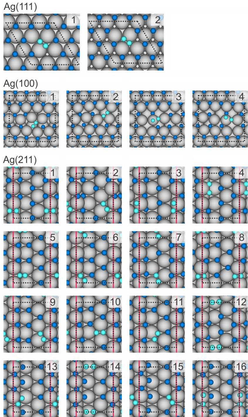
**Figure S6** Top views of all identified high-coverage transition state structures for H<sub>2</sub>/D<sub>2</sub> dissociative adsorption (initial state 7/9 ML; final state 1 ML) on the (111), (100), and (211) surfaces of Ag. Structures are labelled by their entry numbers in Table S4. Red lines mark the step edges. The unit cell is marked by dashed lines. Color code: grey – Ag, blue – spectator H, cyan – dissociating H<sub>2</sub> molecule.
