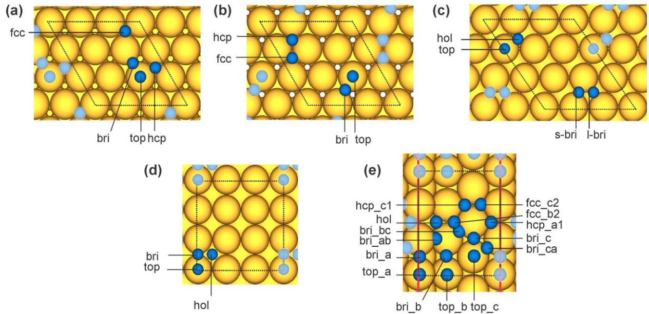
**Figure S3** Top view of high-symmetry sites for adsorption of atomic H on (a) fcc (111) surfaces, (b) hcp (0001) surfaces, (c) bcc (110) surfaces, (d) fcc (100) surfaces, and (e) fcc (211) surfaces, where red lines mark the step edges. “hol” and “bri” are abbreviations for “hollow” and “bridge” respectively. Dashed lines mark the unit cell. Color code: yellow – metal, blue – H in unit cell, light blue – H out of unit cell.
