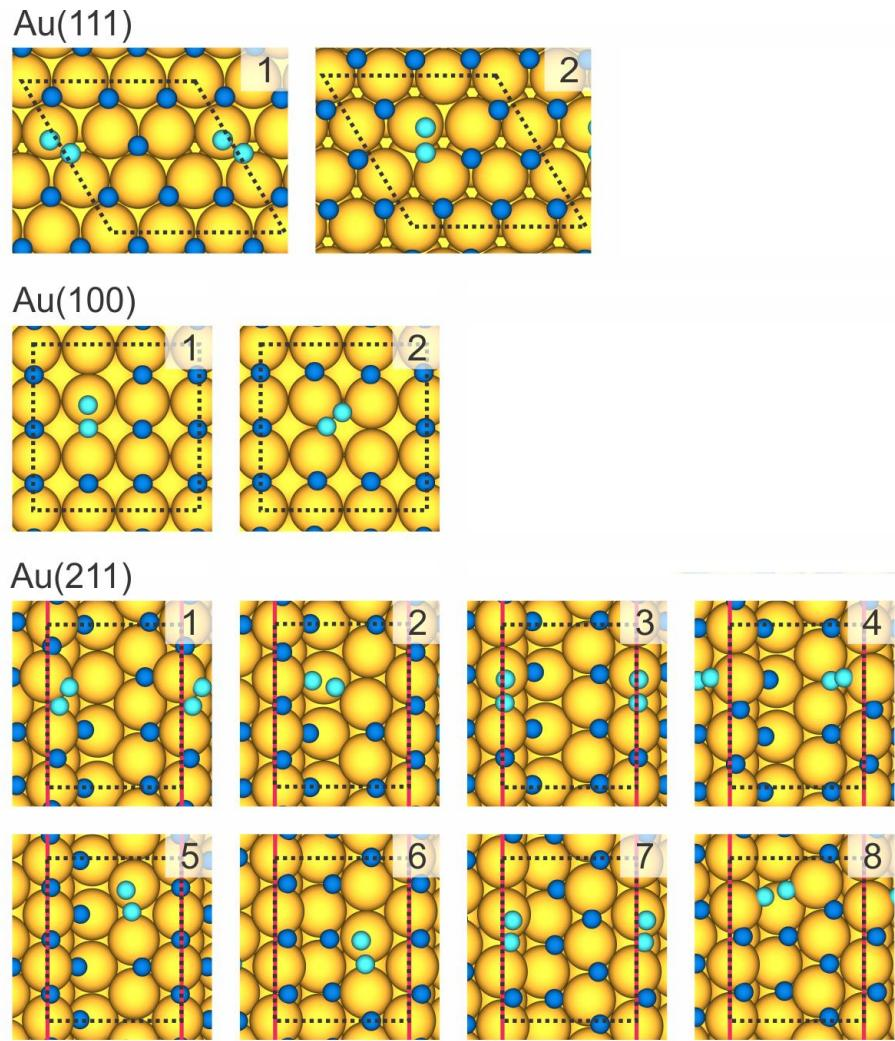
**Figure S7** Top views of all identified high-coverage transition state structures for  $\text{H}_2/\text{D}_2$  dissociative adsorption (initial state 7/9 ML; final state 1 ML) on the (111), (100), and (211) surfaces of Au. Structures are labelled by their entry numbers in Table S4. Red lines mark the step edges. The unit cell is marked by dashed lines. Color code: yellow – Au, blue – spectator H, cyan – dissociating  $\text{H}_2$  molecule.
