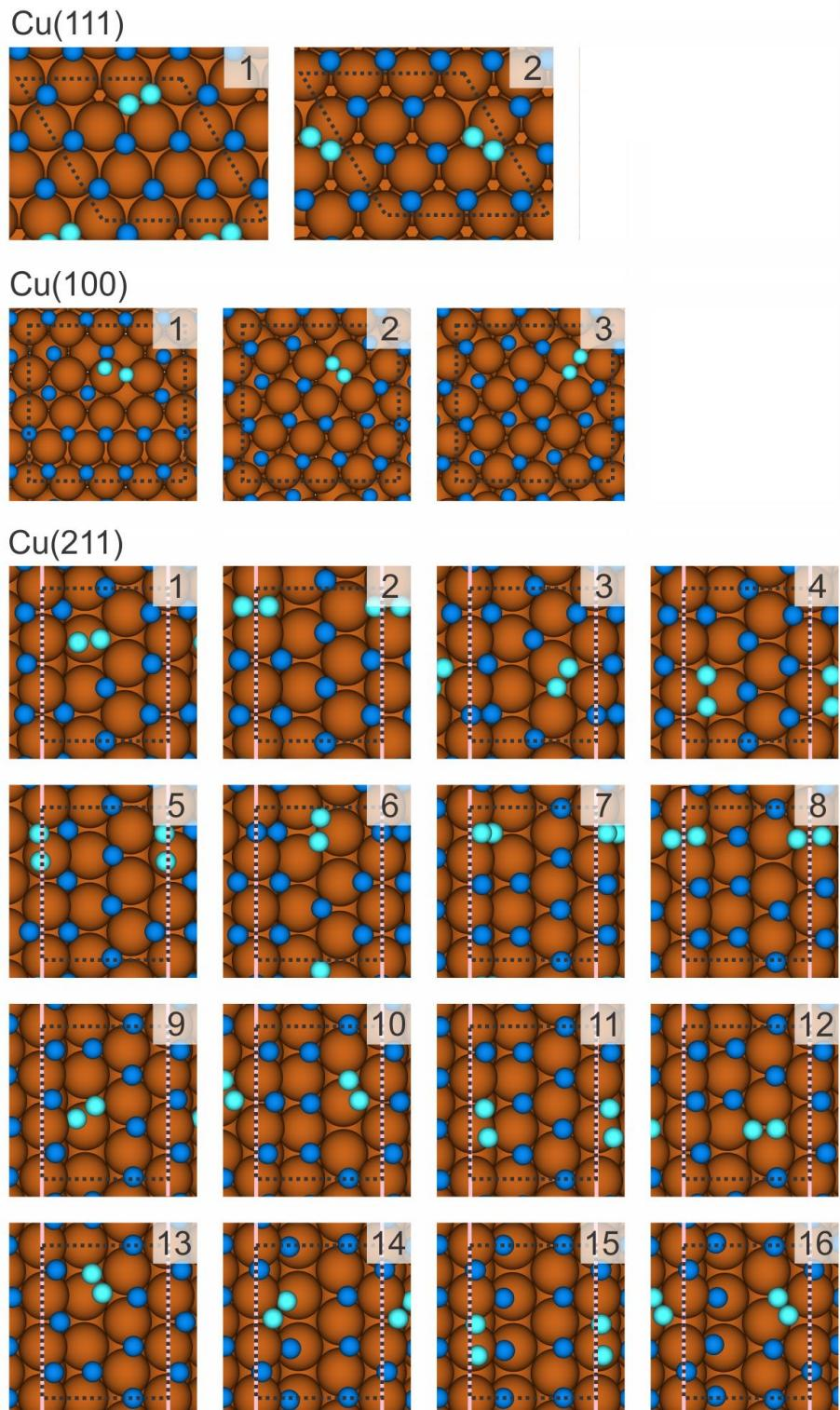
**Figure S8** Top views of all identified high-coverage transition state structures for  $\text{H}_2/\text{D}_2$  dissociative adsorption (initial state 7/9 ML; final state 1 ML) on the (111), (100), and (211) surfaces of Cu. Structures are labelled by their entry numbers in Table S4. Pink lines mark the step edges. The unit cell is marked by dashed lines. Color code: brown – Cu, blue – spectator H, cyan – dissociating  $\text{H}_2$  molecule.
