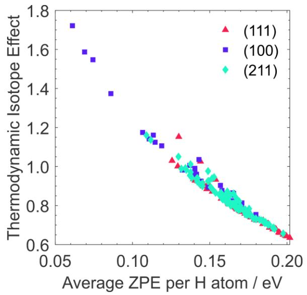
**Figure S5** Calculated average zero-point energies (ZPEs) per H atom versus calculated thermodynamic isotope effects (TIEs) for all structures listed in Tables 1–3 of the main text. The TIE's are evaluated at 623 K and 0.1 atm H<sub>2</sub>/D<sub>2</sub> pressure.
