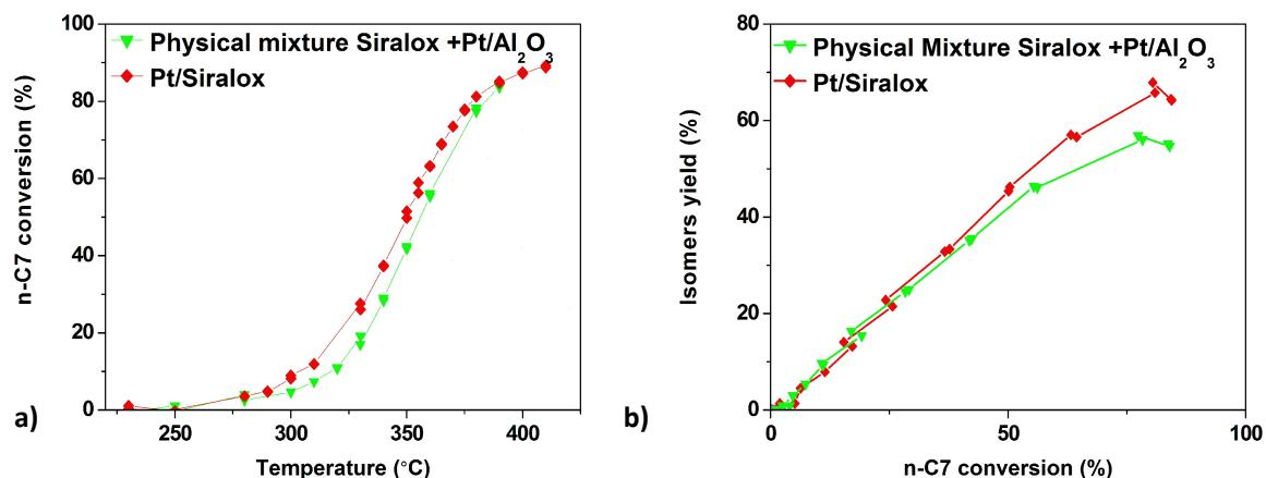
Fig SI.11.a. Conversion profile of n-heptane against temperature for Pt-Siralox40hpv ( $[\text{Pt}(\text{NH}_3)_4](\text{NO}_3)_2$ ) (red diamonds);  $\text{Pt}-\gamma\text{-Al}_2\text{O}_3 + \text{Siralox40hpv}$  (green squares), physical mixture of 75-212  $\mu\text{m}$  grains b. Yields of C7 isomers Catalysis performed at 10 bar ;  $\text{H}_2/\text{n-C}_7 = 10/1$  mol/mol; WHSV = 1.15 g<sub>n-C7</sub>.g<sub>solid acid</sub>.h<sup>-1</sup>
