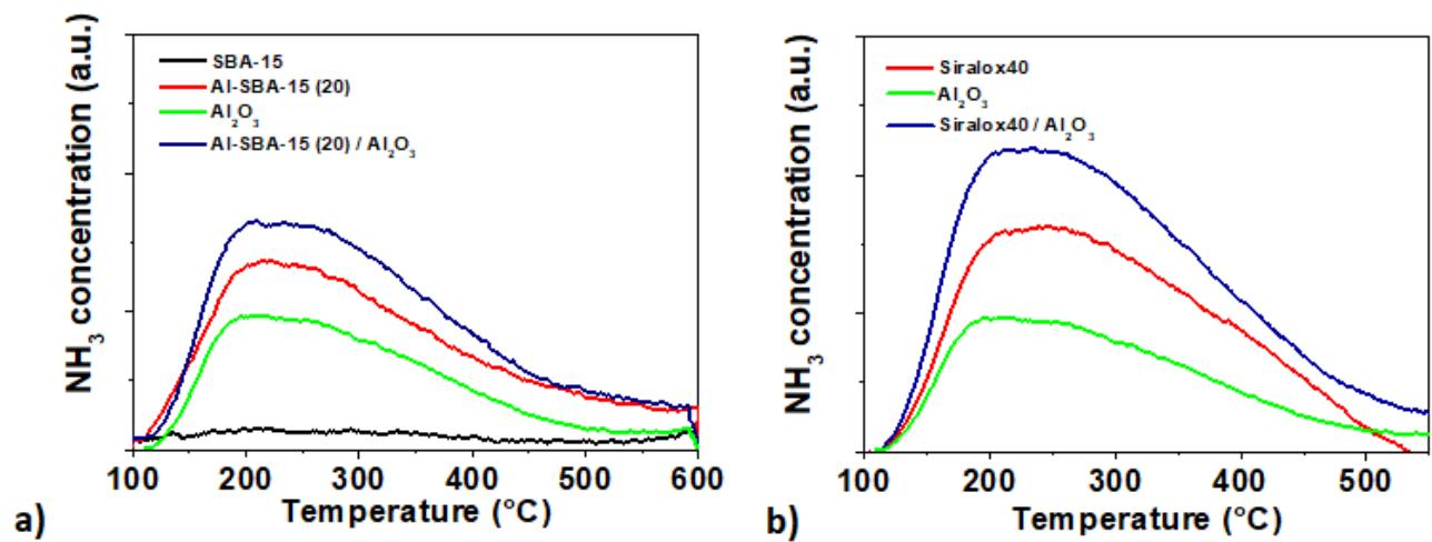
Fig. SI.7 NH<sub>3</sub>-TPD measurements of a) SBA-15; black line, Al-SBA-15(20), red line;  $\gamma$ -Al<sub>2</sub>O<sub>3</sub>, green line; composite Al-SBA-15(20)/  $\gamma$ -Al<sub>2</sub>O<sub>3</sub>, blue line b) Siralox40, red line;  $\gamma$ -Al<sub>2</sub>O<sub>3</sub>, green line; composite Siralox40/ $\gamma$ -Al<sub>2</sub>O<sub>3</sub>, blue line
