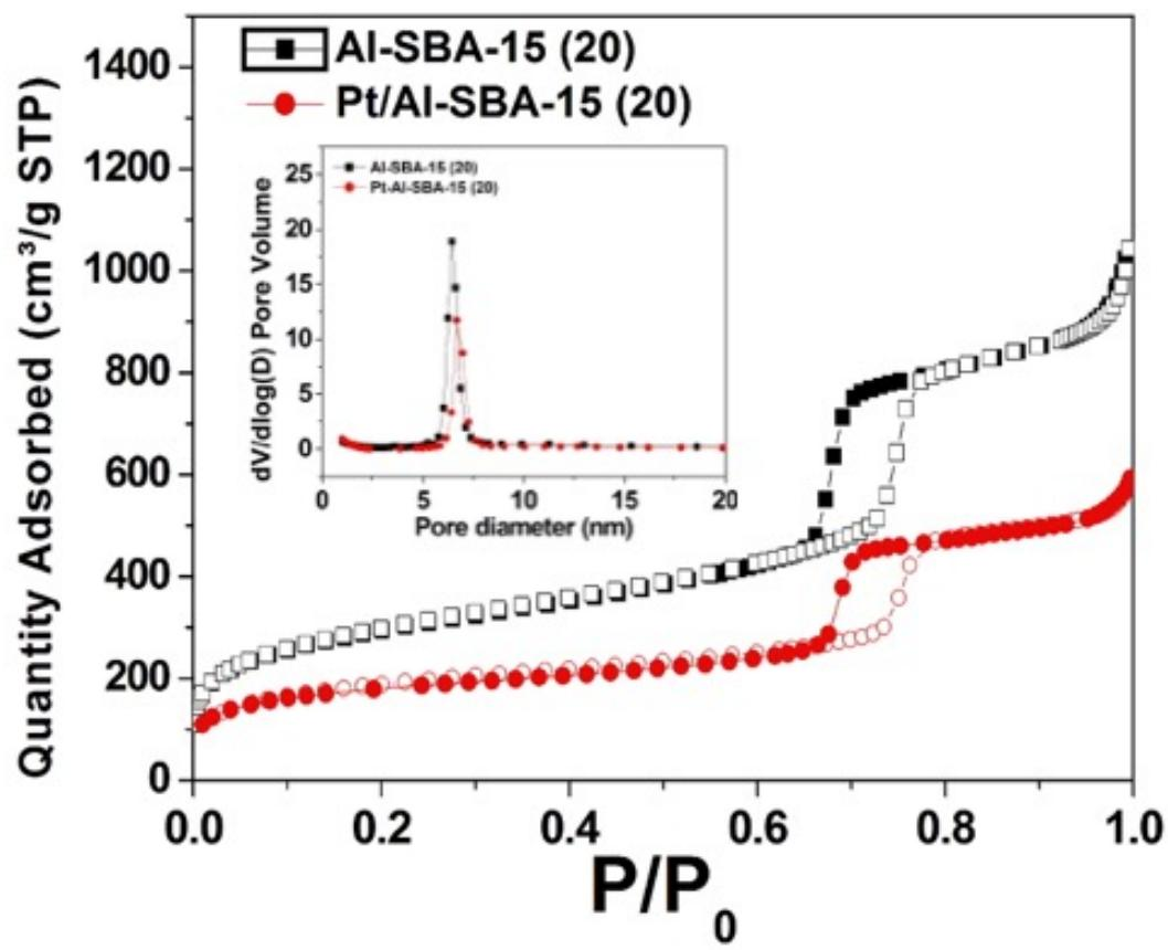
Fig. SI.14 N<sub>2</sub> physisorption analysis of Al-SBA-15(20), black line, and Pt-Al-SBA-15(20) red line. Both contain mesopores with an average pore size around 6 nm.
