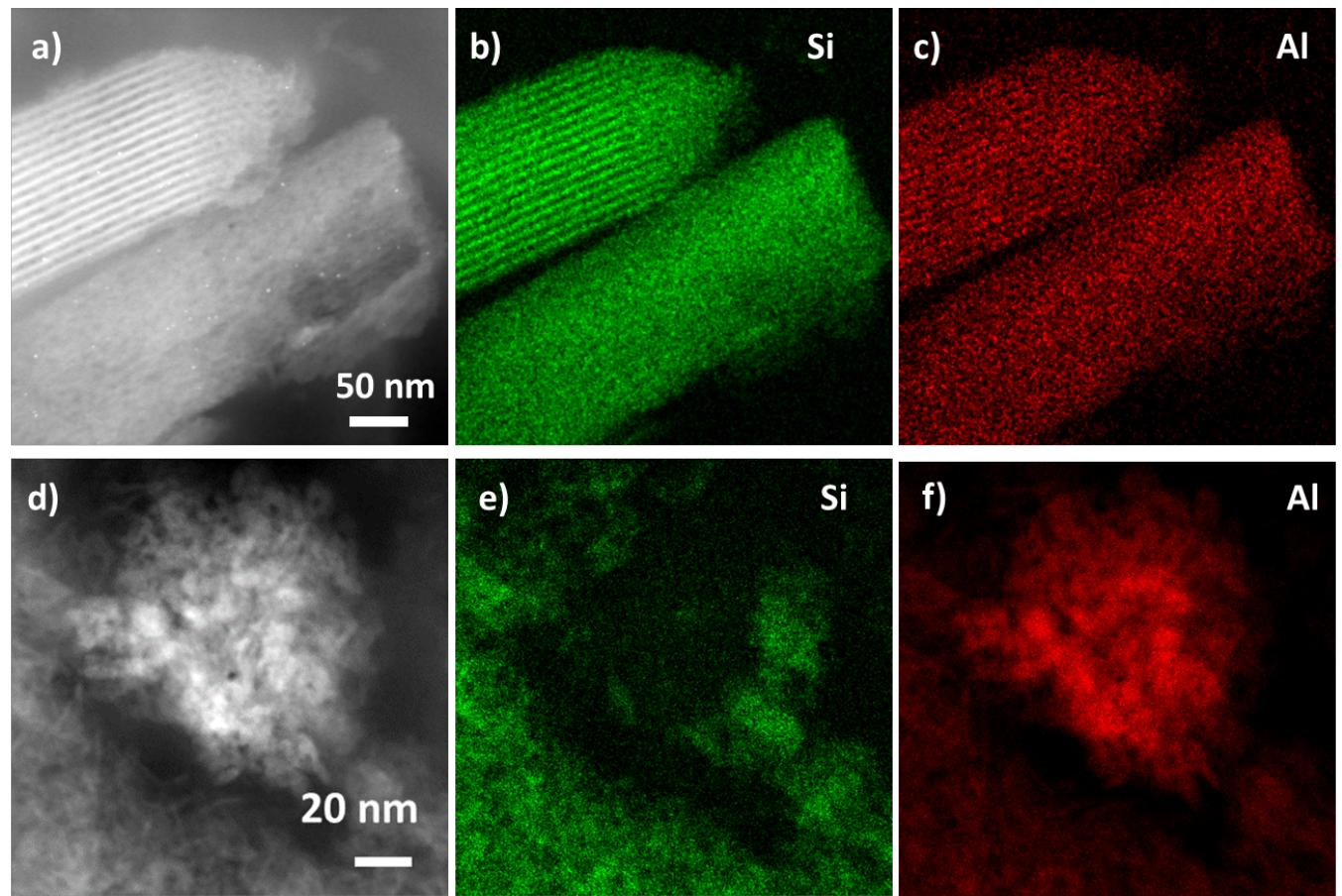
Fig SI.2 a. HAADF-STEM image of Al-SBA-15(20). b. and c. EDX mapping of Si and Al. Al elemental mapping suggest a uniform Al dispersion along the walls of SBA-15
