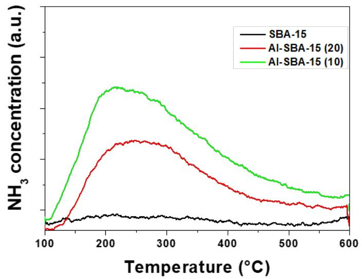
Fig. SI.3 NH<sub>3</sub>-TPD measurements of SBA-15; black line, Al-SBA-15(20), red line; Al-SBA-15(10), green line;
