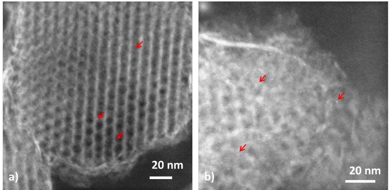
Fig SI.8. TEM images of the Pt-Al-SBA-15/ $\gamma$ -Al<sub>2</sub>O<sub>3</sub> catalyst. Pt particles are observed on the Al-SBA-15 (a) but also on the binder (b), pointing to an non-selective Pt deposition.
