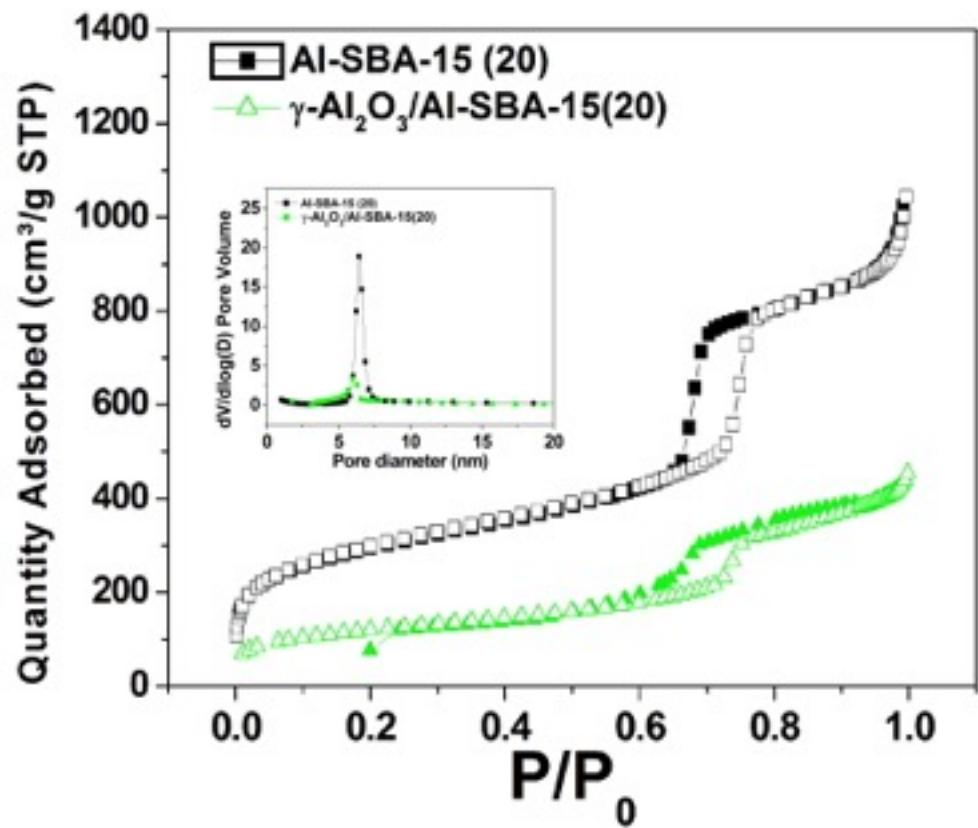
Fig. SI.6 N<sub>2</sub> physisorption analysis of Al-SBA-15(20), black line which and composite Al-SBA-15(20)/γ-Al<sub>2</sub>O<sub>3</sub> green line. Both contain mesopores with an average pore size around 6 nm.
