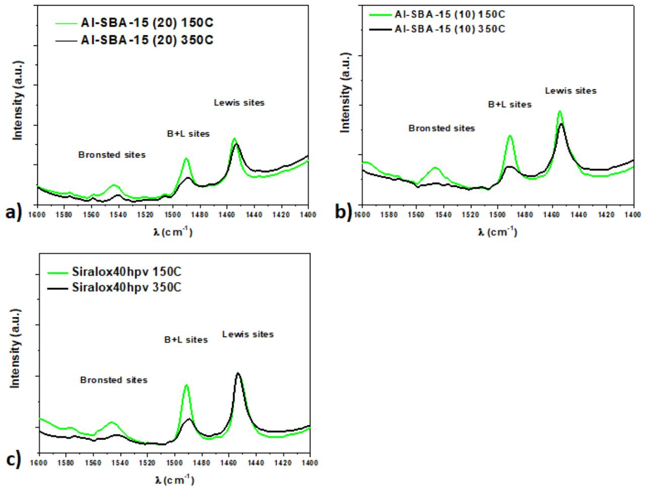
Fig SI.4 Pyridine desorption - Infrared spectrum of a) Al-SBA-15(20) b) Al-SBA-15(10) c) Siralox40hpv (Desorption at 150°C (green line); and 350°C (black line) at  $1.10^{-5}$  bar)
