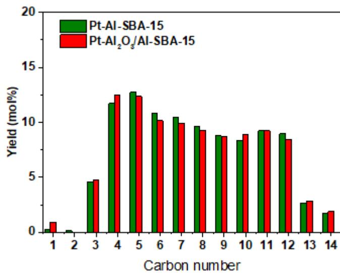
Fig SI.12. Cracking products distribution (mol%) per function of their carbon number for Pt-Al-SBA-15 and Pt-Al<sub>2</sub>O<sub>3</sub>/Al-SBA-15 at *n*-C16 conversion = 80%, T = 290 °C.
