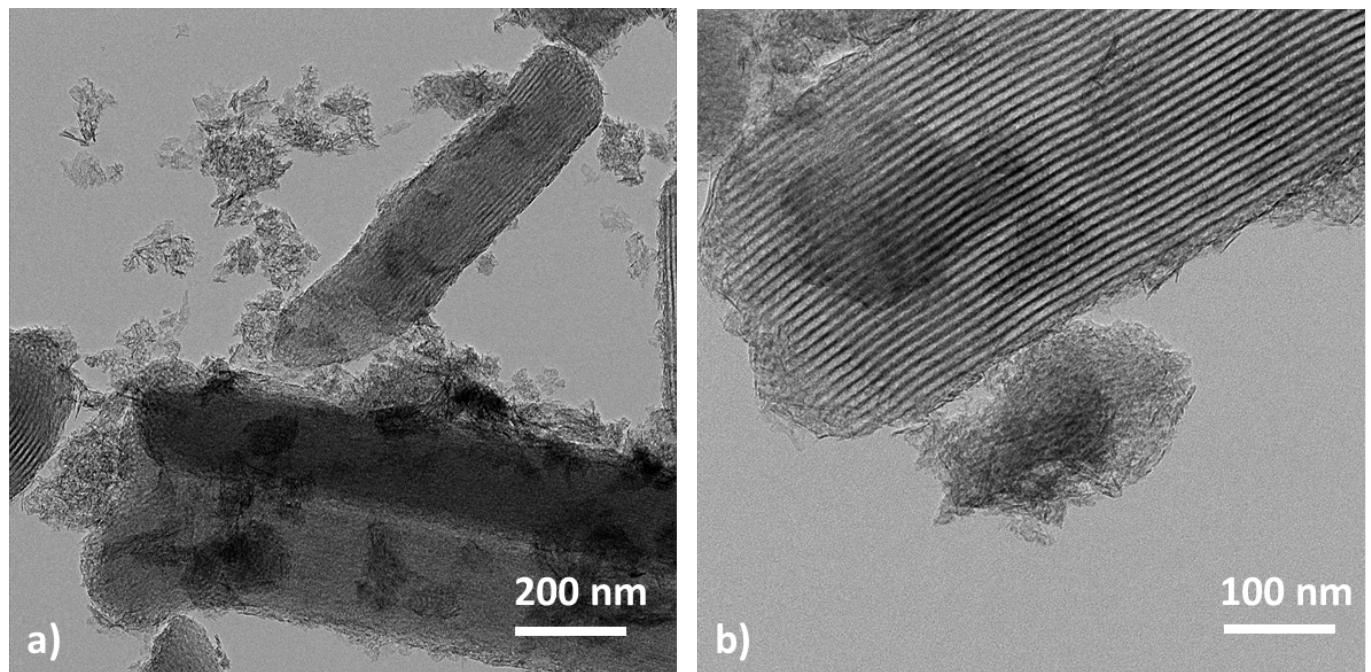
Fig SI.5 TEM images of the  $\gamma$ - $\text{Al}_2\text{O}_3$ /Al-SBA-15 composite. The coverage of Al-SBA-15 by the alumina is apparent from Fig. SI.5-b.
