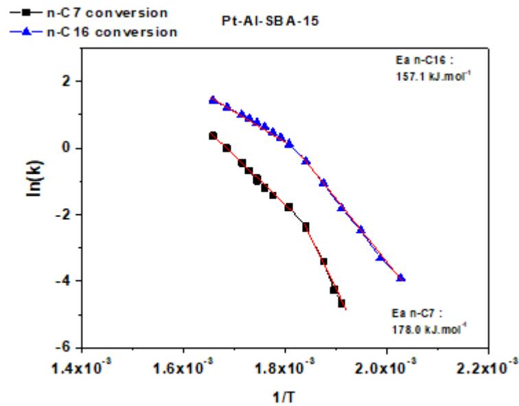
Fig SI.13. Arrhenius plots for  $n\text{-C}_7$  and  $n\text{-C}_{16}$  conversion for Pt-Al-SBA-15(20).
