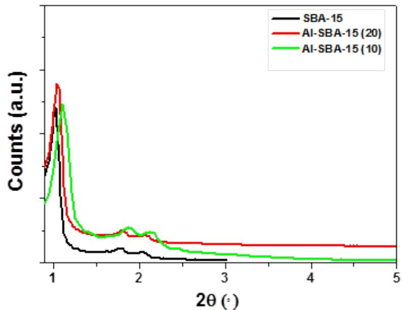
Fig. SI.1 Small angle XRD measurements of SBA-15; black line, Al-SBA-15(20), red line; Al-SBA-15(10), green line.
