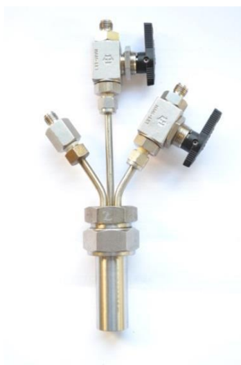
Figure 1: 25 mL stainless steel autoclave for screening experiments (left) and glass autoclave for recycling experiments (right)
