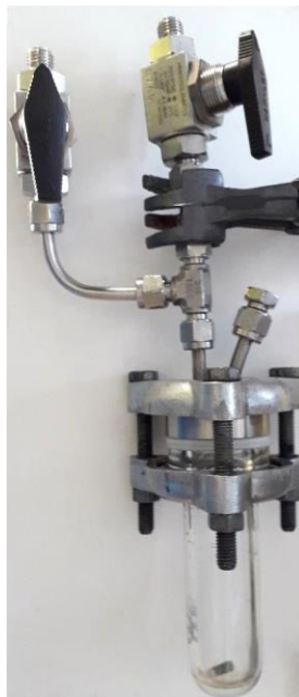
Figure 1: 25 mL stainless steel autoclave for screening experiments (left) and glass autoclave for recycling experiments (right)
