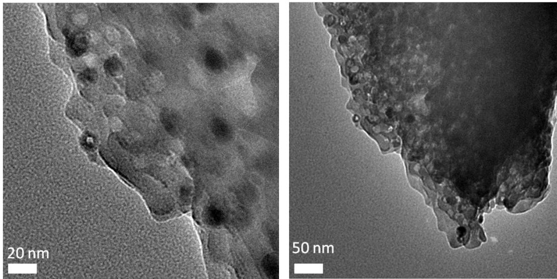
**Fig. S5.** TEM images of Cu(5)@LP-S16C-40 at different resolutions.
