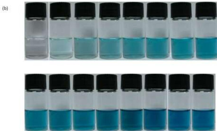
Fig. S1 Absorption spectra (a) and photographs (b) of UCNS-oxTMB nanosystem with addition of 0, 1.85, 3.69, 5.52, 7.35, 9.17, 11.0, 14.6, 18.2, 21.7, 25.3, 28.8, 35.7, 44.2, 69.0 and 84.7  $\mu\text{M}$  of  $\text{MnO}_4^-$  ions..
