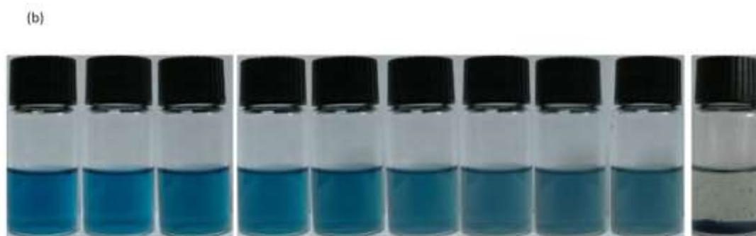
Fig. S6 Absorption spectra (a) and photographs (b) of UCNS-oxTMB nanosystem with addition of 0, 18.3, 36.6, 72.9, 109, 145, 180, 215 and 250  $\mu\text{M}$  of  $\text{Cr}_2\text{O}_7^{2-}$  ions, and last photograph was taken after standing for 1h.
