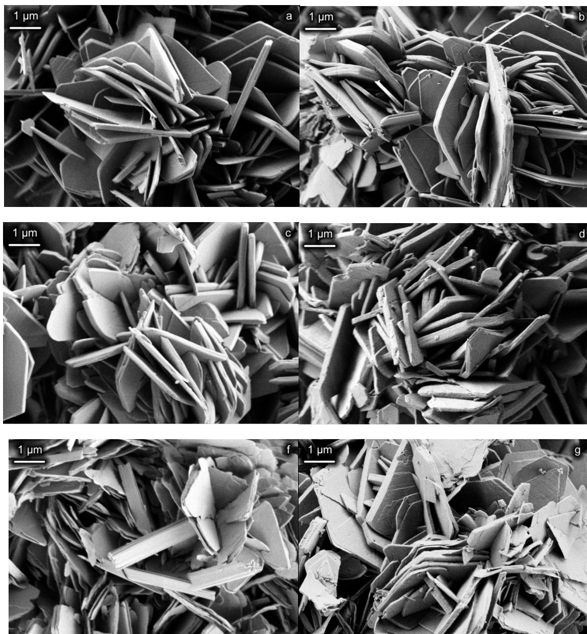
Fig. S2. SEM images of (Y_{0.95}Eu_{0.05})_2(OH)_5NO_3 \cdot 1.7H_2O obtained by refluxing a HMTA, NaNO_3 , Y(NO_3)_3 \cdot nH_2O и Eu(NO_3)_3 \cdot nH_2O solution mixture and the products of its ion exchange reactions with aqueous solutions of (a) phthalic, (b) isophthalic, (c) terephthalic, (d) 2-sulphobenzoic, (e) 3-sulphobenzoic and (f) 4-sulphobenzoic acid salts under HTMW treatment (200 °C, 30 min).
