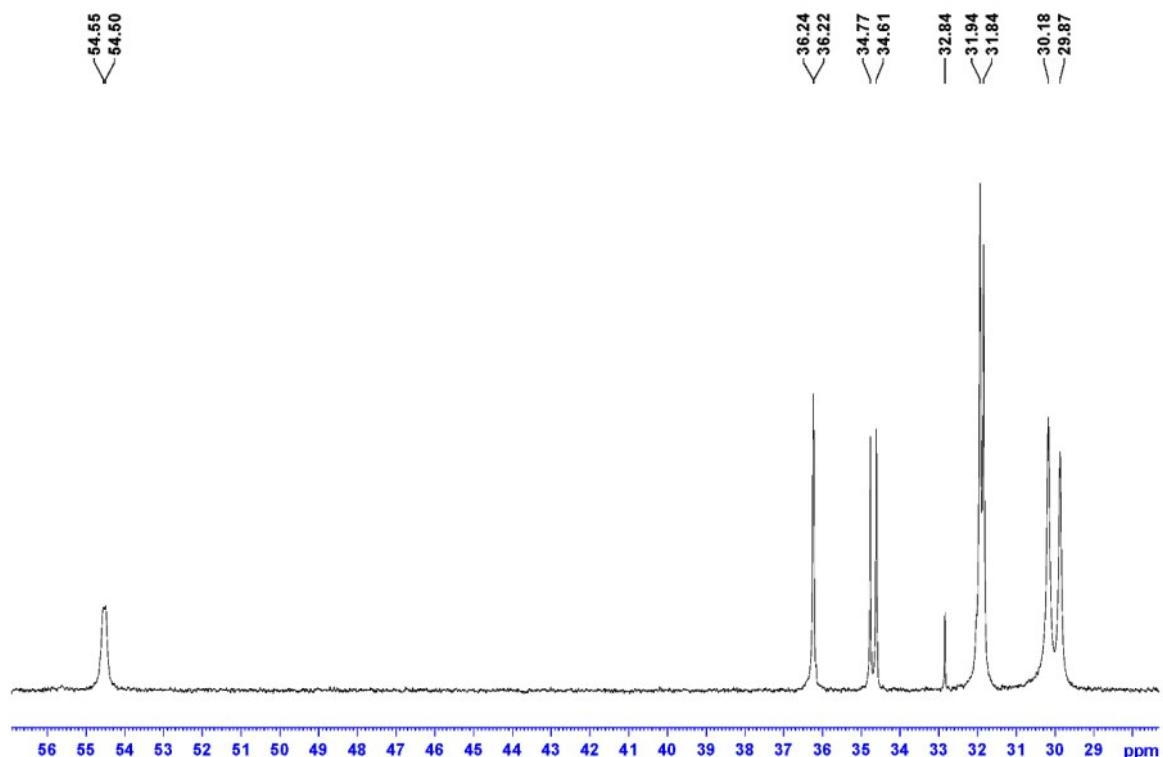
$^{31}\text{P}$  NMR spectrum of **2a** in THF- $d_8$  at 223 K:
