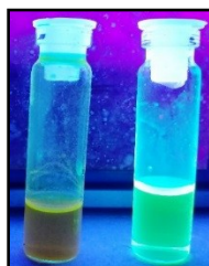
Figure S5. Color of the solution changes from yellow to fluorescent green upon addition of Zn^{2+} .
