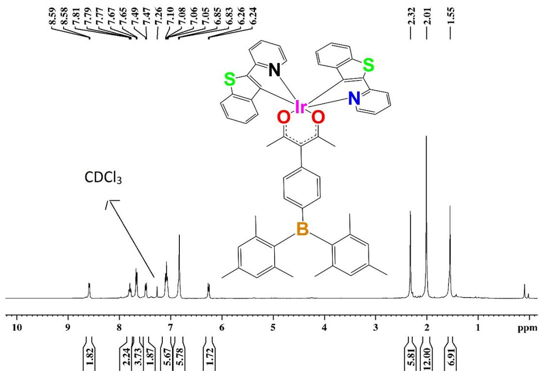
Figure S9: <sup>1</sup>H NMR spectrum of complex 5
