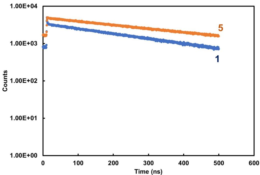
**Figure S25:** Luminescence decay profile of complex **1 and 5** with 375 excitation.
