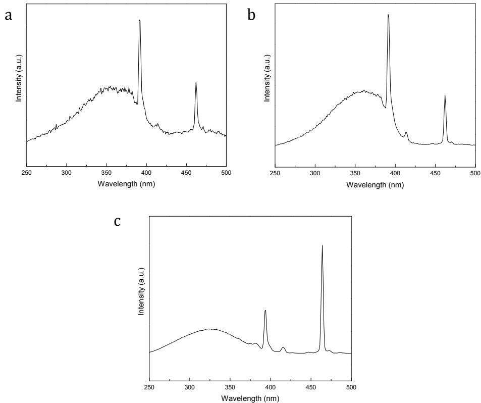
Figure S3 Excitation spectra of a) 1%Eu: LuPOM, b) 2.5%Eu: LuPOM, and c) 5%Eu: LuPOM (observed at the  ${}^5D_0 \rightarrow {}^7F_2$  transition peak)
