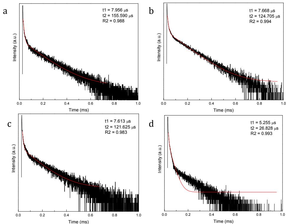
Figure S4 Decay profiles of a) 7.5%Eu: LuPOM, b) 5%Eu: LuPOM, c) 2.5%Eu: LuPOM, d) 1%Eu: LuPOM (excited into the maximum of the LMCT band and observed at the maximum of the  $^5D_0 \rightarrow ^7F_2$  transition peak)
