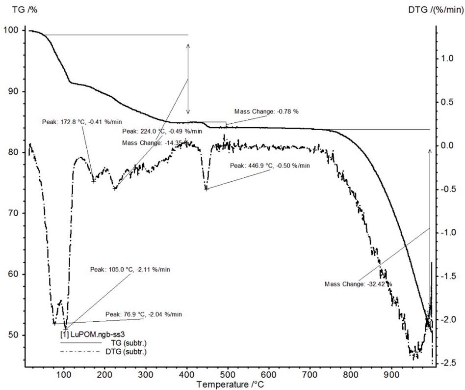
Figure S5 TGA and DTG of LuPOM compound.
