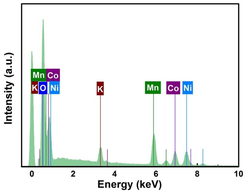
**Fig. S3** EDX spectrum of the  $\text{NiCo}_2\text{O}_4@\text{MnO}_2/\text{NF}/\text{MnO}_2$  sandwiches.
