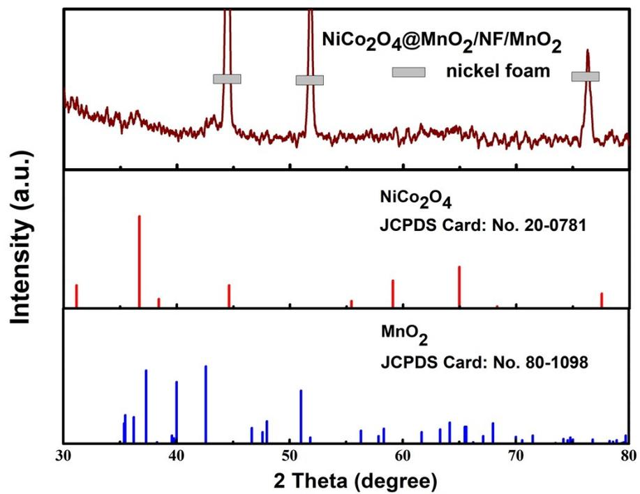
**Fig. S4** XRD patterns of the  $\text{NiCo}_2\text{O}_4@MnO_2/NF/MnO_2$  sandwiches.
