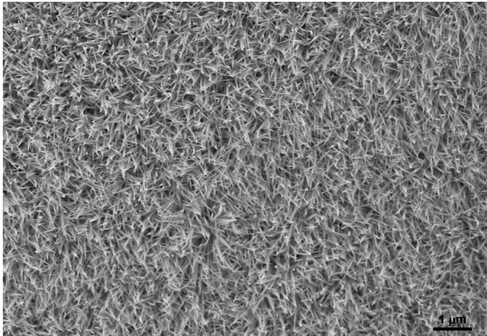
**Fig. S1** FESEM images of the as-synthesized cobalt-nickel hydroxide precursor nanowire arrays grown on NF.
