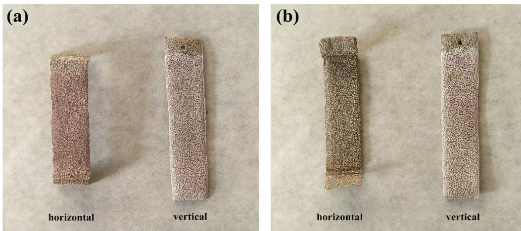
**Fig. S2** (a, b) The different distributions of cobalt-nickel hydroxide precursors on NF.
