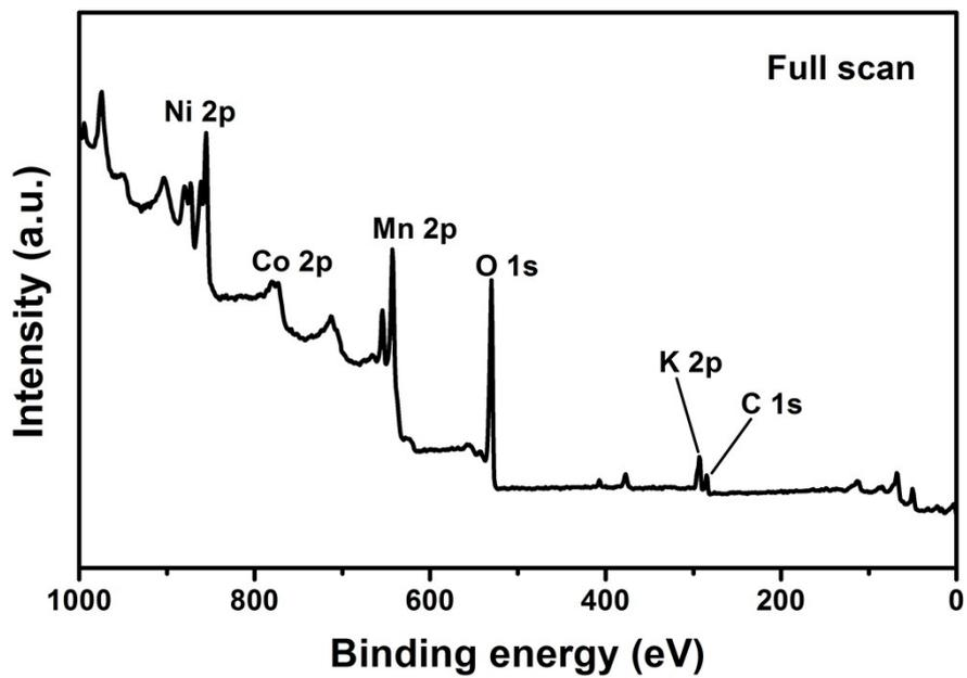
**Fig. S6** XPS spectrum of survey for the as-fabricated NiCo<sub>2</sub>O<sub>4</sub>@MnO<sub>2</sub>/NF/MnO<sub>2</sub> sandwiches.
