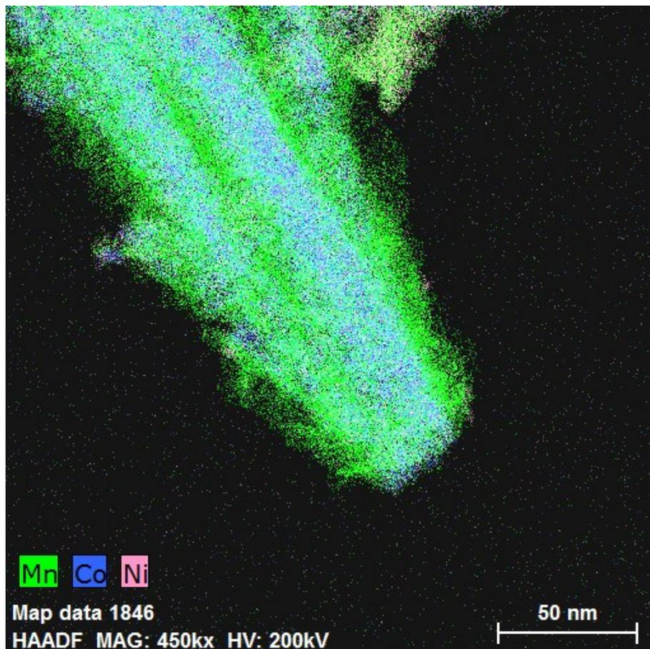
**Fig. S5** The corresponding EDX mapping image showing the distribution of Mn, Co, and Ni for NiCo<sub>2</sub>O<sub>4</sub>@MnO<sub>2</sub> core-shell structures.
