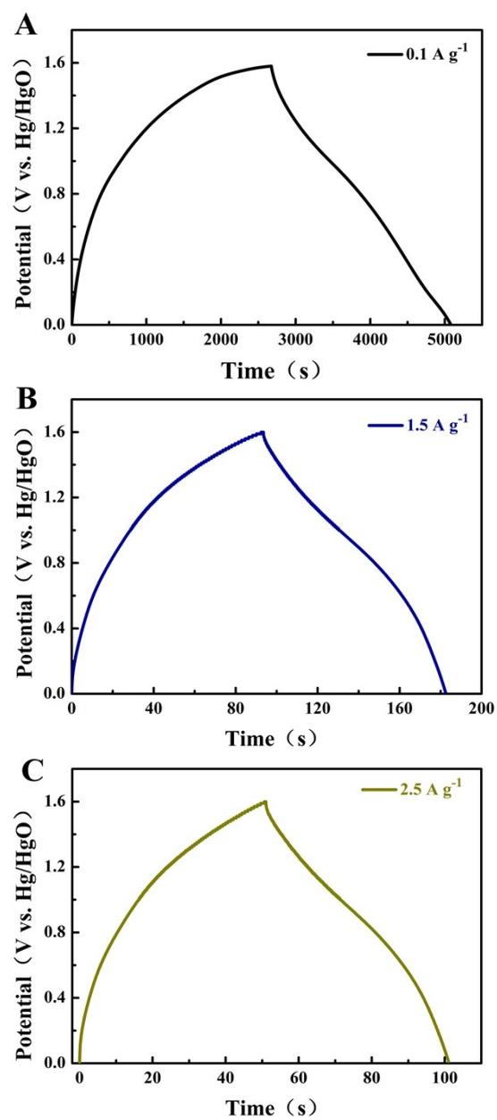
**Fig. S8** the GCD curves of HSC at  $0.1 \text{ A g}^{-1}$  (A),  $1.5 \text{ A g}^{-1}$  (B) and  $2.5 \text{ A g}^{-1}$  (C).
