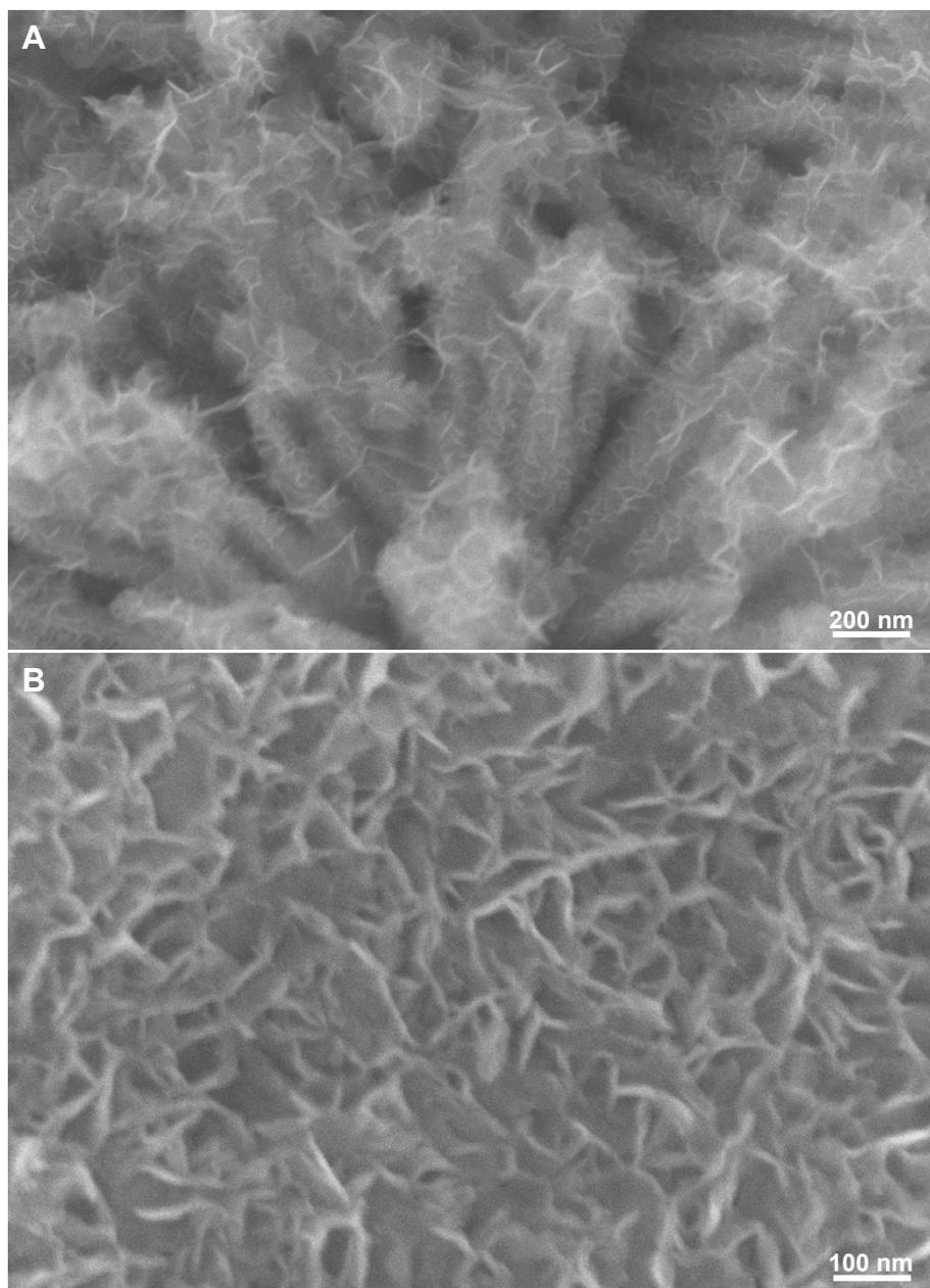
**Fig. S7** FESEM images of the side A (A) and side B (B) of  $\text{NiCo}_2\text{O}_4@\text{MnO}_2/\text{NF}/\text{MnO}_2$  sandwiches after 30,000 cycles.
