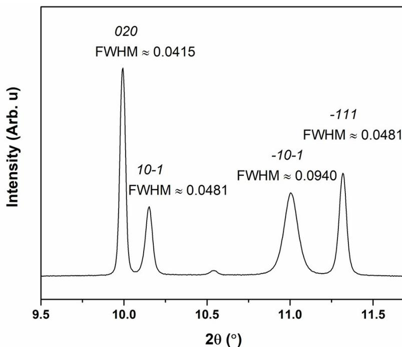
**Figure S4.** SR PXD data measured at  $-52 \text{ }^\circ\text{C}$ ,  $\lambda = 0.70848 \text{ \AA}$ , for  $\alpha\text{-KB}_3\text{H}_8$ , shown in the  $2\theta$  range 9.5 to 11.7°. The full width half maximum values are provided for four selected  $hkl$  reflections.
