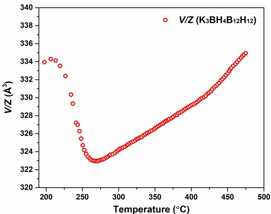
**Figure S5:** Volume per formula unit ( $V/Z$ ) extracted from sequential Rietveld refinement of  $K_3BH_4B_{12}H_{12}$  from SR PXD data of the as synthesized  $KB_3H_8$  sample measured at Diamond ( $\lambda = 0.824598 \text{ \AA}$ ) in the temperature range 198 to 475 °C.
