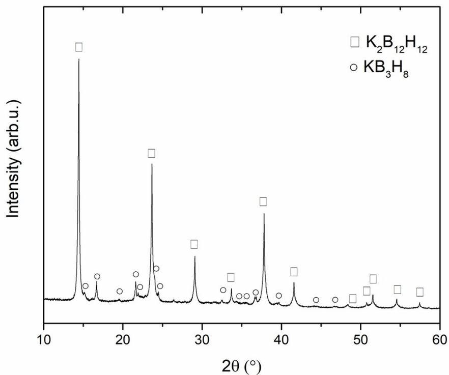
**Figure S7.** PXD pattern of sample **s5** measured at *RT*,  $\lambda = 1.54056 \text{ \AA}$ . Two crystalline compounds,  $\text{K}_2\text{B}_{12}\text{H}_{12}$  and  $\text{KB}_3\text{H}_8$ , are observed.
