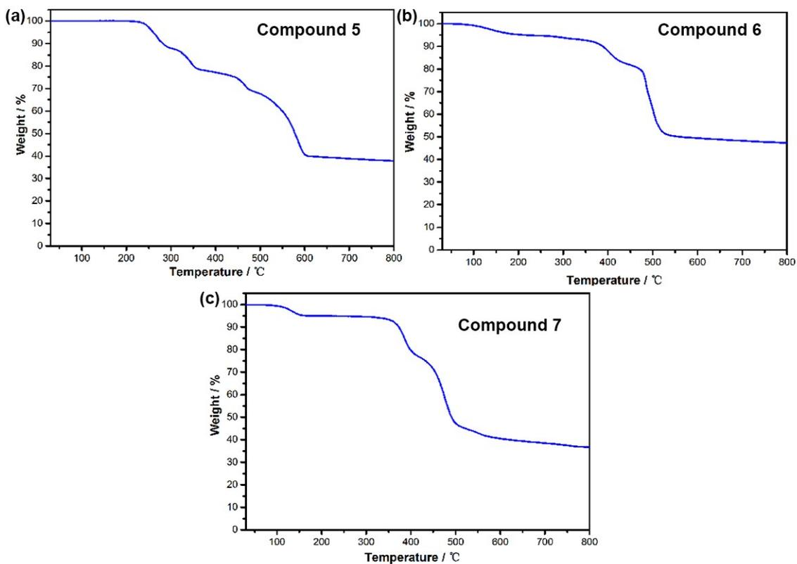
**Figure S4.** Thermogravimetric analysis curves of compounds 5-7.
