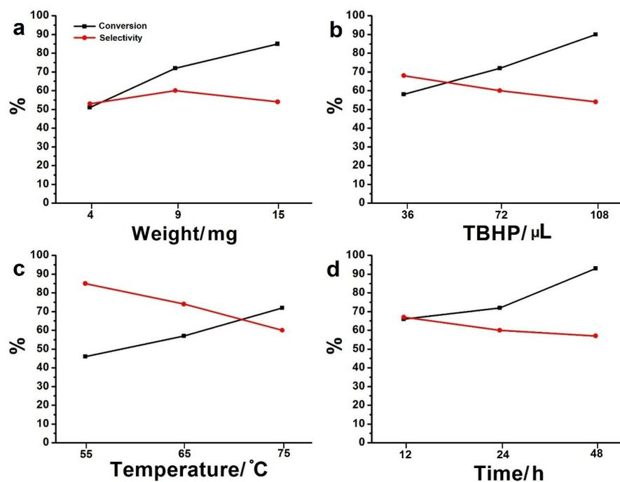
**Figure S6.** Linear relationship diagrams for the oxidation of styrene with compound 7 as catalyst: (a) Weight of catalyst vs Conversion/Selectivity; (b) amount of TBHP vs Conversion/Selectivity; (c) Temperature vs Conversion/Selectivity; (d) Time vs Conversion/Selectivity.
