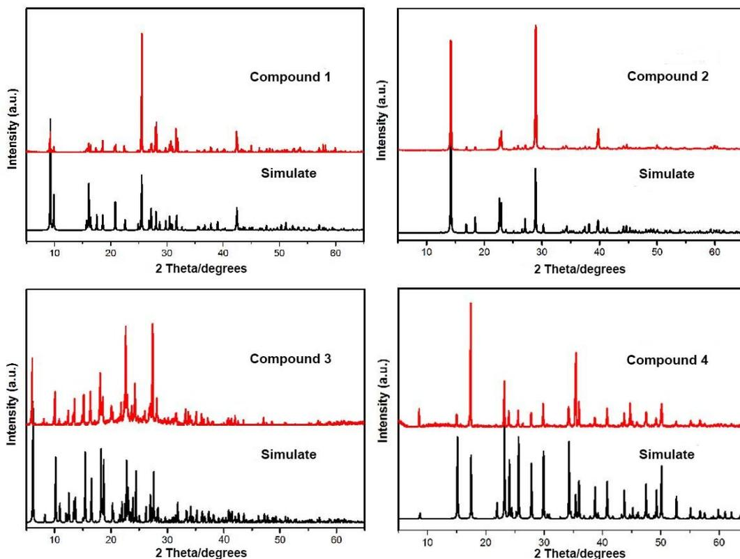
**Figure S1.** The experimental (red) and simulated (black) PXRD patterns of compounds **1-4**.
