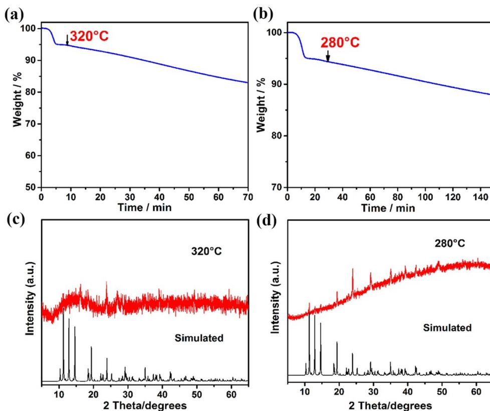
**Figure S8.** TGA curves of compound 7 heated at 320°C (a) and 280°C (b); comparison between simulated (black) PXRD pattern and experimental (red) PXRD pattern of samples heated at 320°C (c) and 280°C (d).
