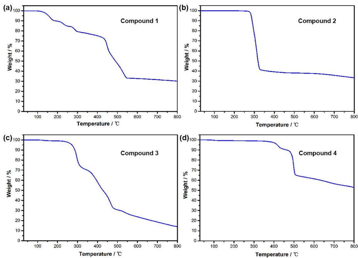
**Figure S3.** Thermogravimetric analysis curves of compounds 1-4.
