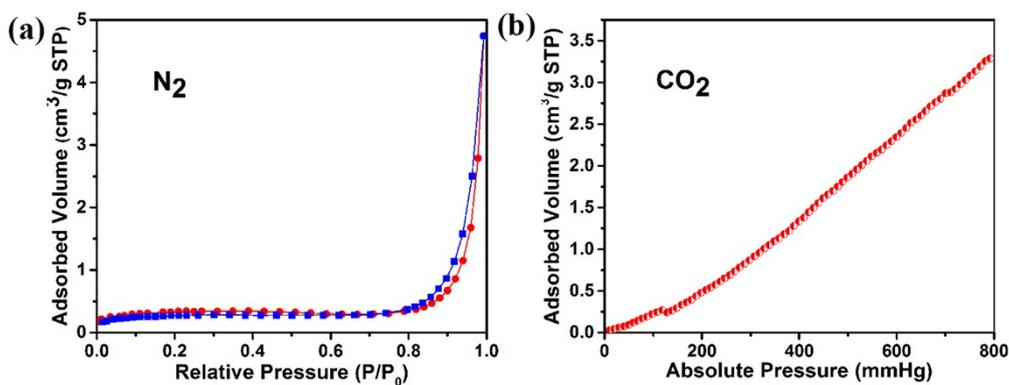
**Figure S7.** (a) N<sub>2</sub> adsorption-desorption isotherms and (b) CO<sub>2</sub> adsorption isotherms.
