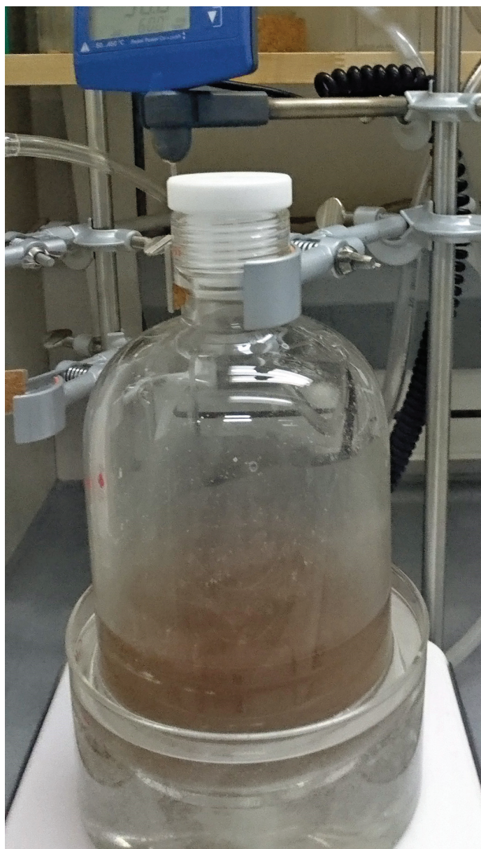
Photo 2. Heating of the reaction mixture at 60 °C after addition of \text{CF}_3\text{SiMe}_3 in a tightly closed reaction vessel immersed in an oil bath preheated at 60 °C.
