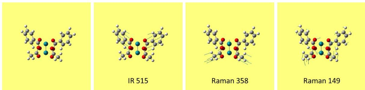
Figure S 20: Most prominent calculated vibrational modes of cis- $[Rh_2(OBz)_2(OAc)_2]$ .
