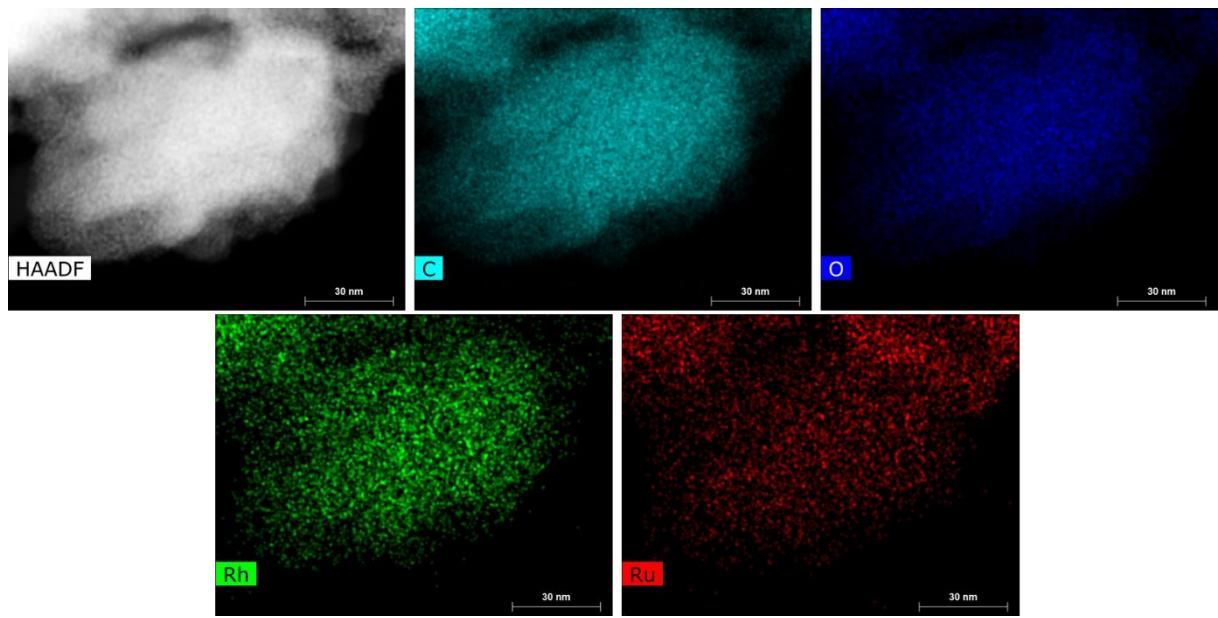
*Figure S 5:* HR-STEM images of representative particle of 75% Rh sample: From left to right: HAADF image and elemental mapping for C, O, Ru and Rh (map2).
