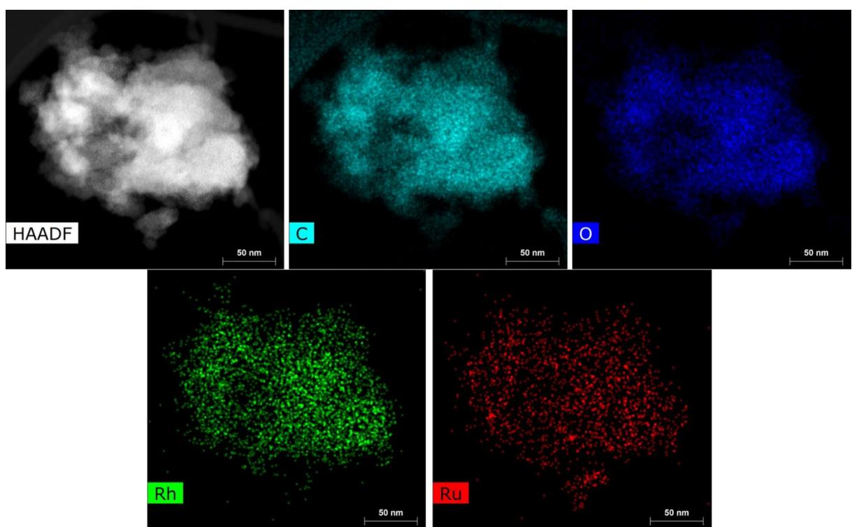
Figure S 4: HR-STEM images of representative particle of 75% Rh sample: From left to right: HAADF image and elemental mapping for C, O, Ru and Rh (map1).
