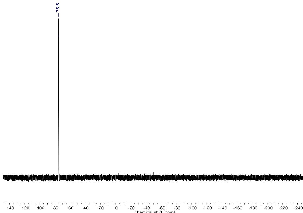
Figure S 32 <sup>31</sup>P {<sup>1</sup>H} NMR (243 MHz, C<sub>6</sub>D<sub>6</sub>, rt) of Et<sub>3</sub>PO·B(C<sub>6</sub>F<sub>5</sub>)<sub>3</sub> without MgN<sup>F</sup><sub>2</sub>.
