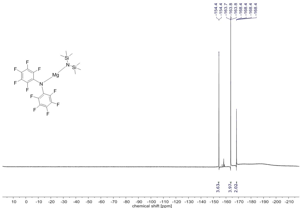
Figure S 17  $^{19}F\{^1H\}$  NMR (565 MHz,  $C_6D_6$ , rt) of  $(N^F Mg N'')_2$ .
