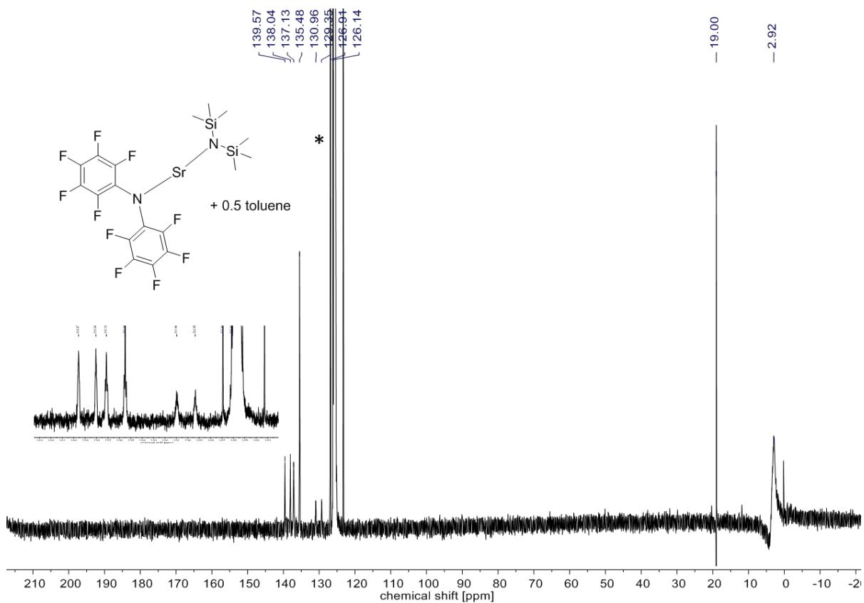
Figure S24  $^{13}\text{C}\{\text{H}\}$  NMR (151 MHz,  $\text{C}_6\text{D}_6$ , rt) of  $(\text{N}^{\text{F}}\text{SrN}^{\prime})_2$ , with co-crystallized toluene.
