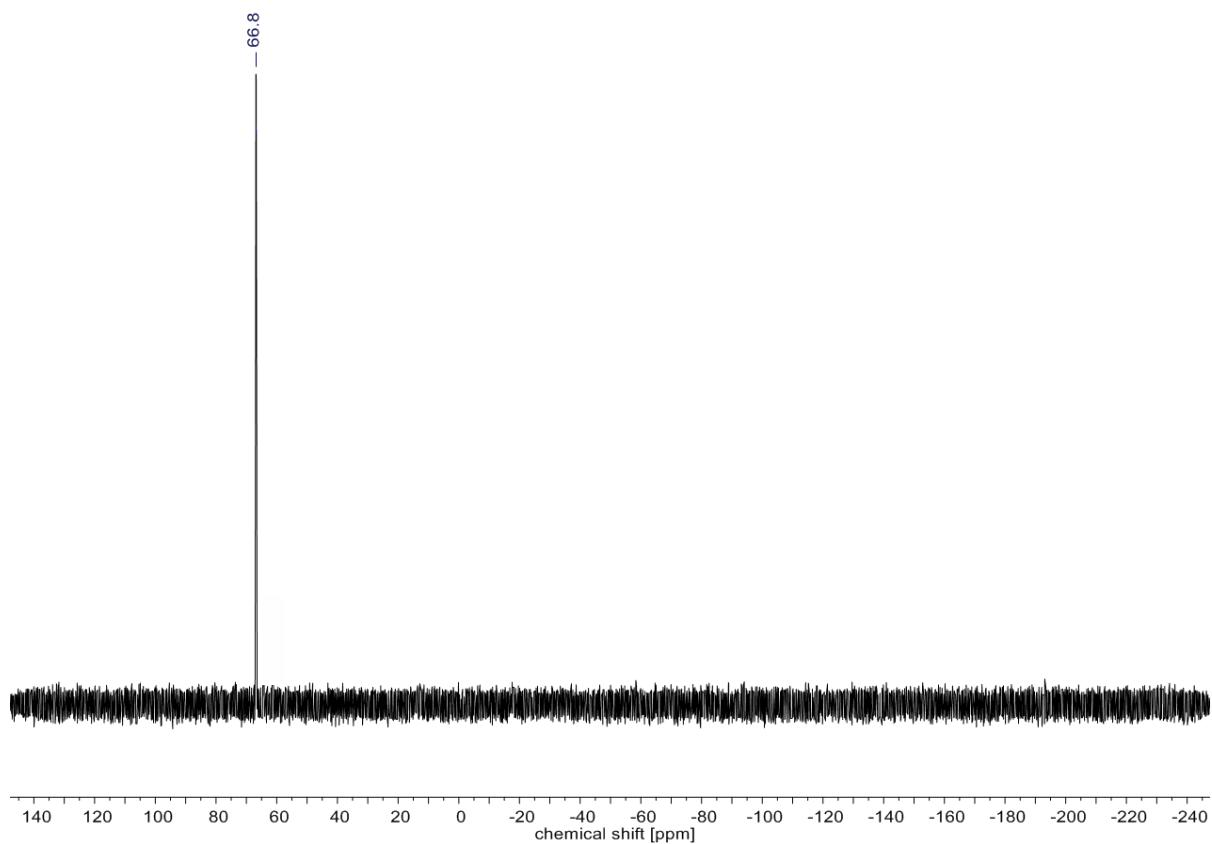
Figure S28  $^{31}\text{P}\{\text{H}\}$  NMR (243 MHz,  $\text{C}_6\text{D}_6$ , rt) of  $\text{OPEt}_3$  with  $\text{MgNF}_2$
