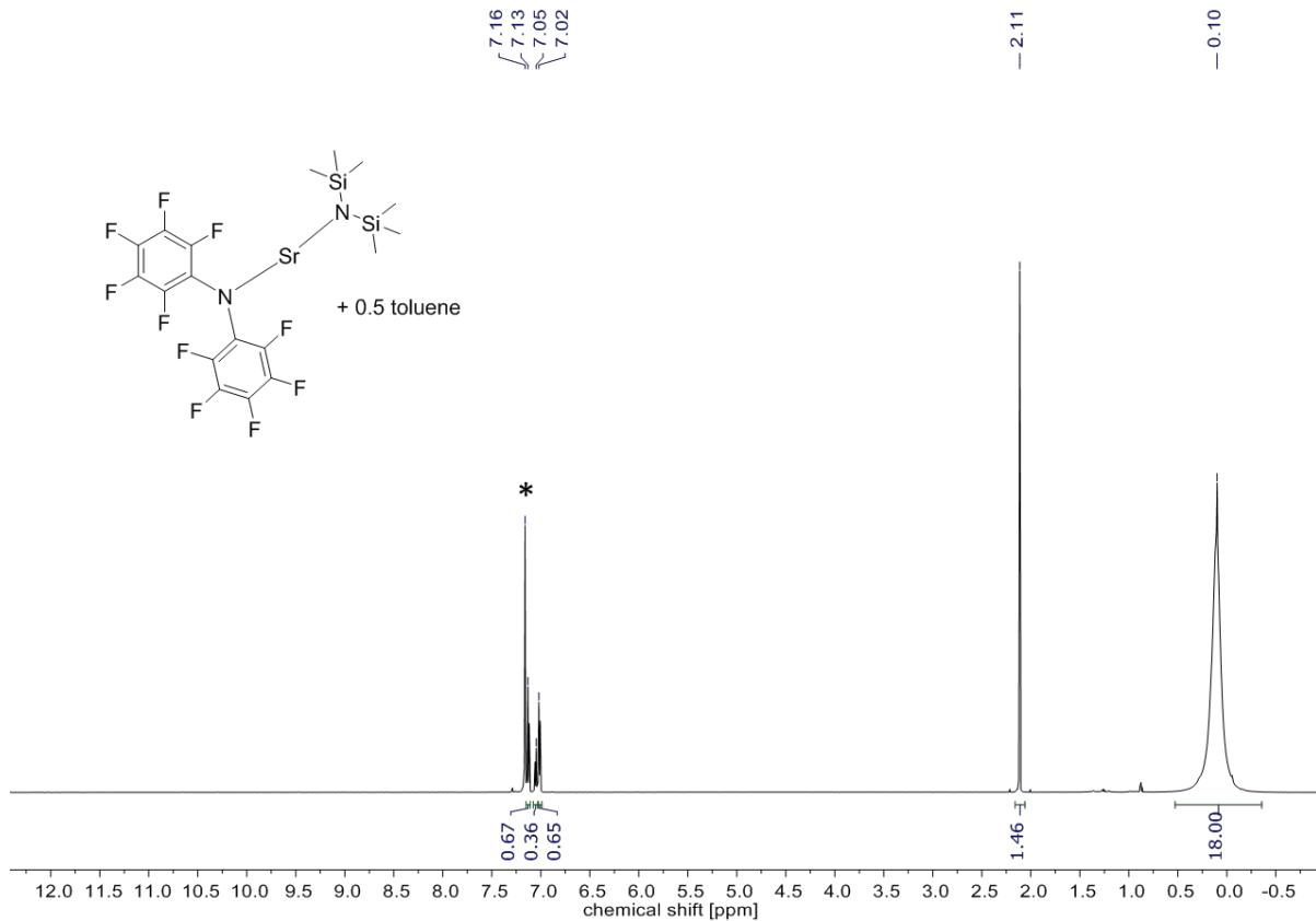
Figure S 22  $^1\text{H}$  NMR (600 MHz,  $\text{C}_6\text{D}_6$ ,  $rt$ ) of  $(\text{N}^{\text{F}}\text{SrN}')_2$ , with co-crystallized toluene.
