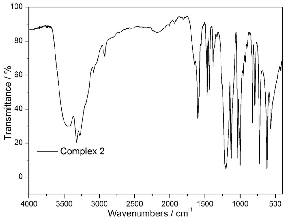
**Figure S10.** Infrared spectra of complex **2<sub>BPDS</sub>** at room temperature
