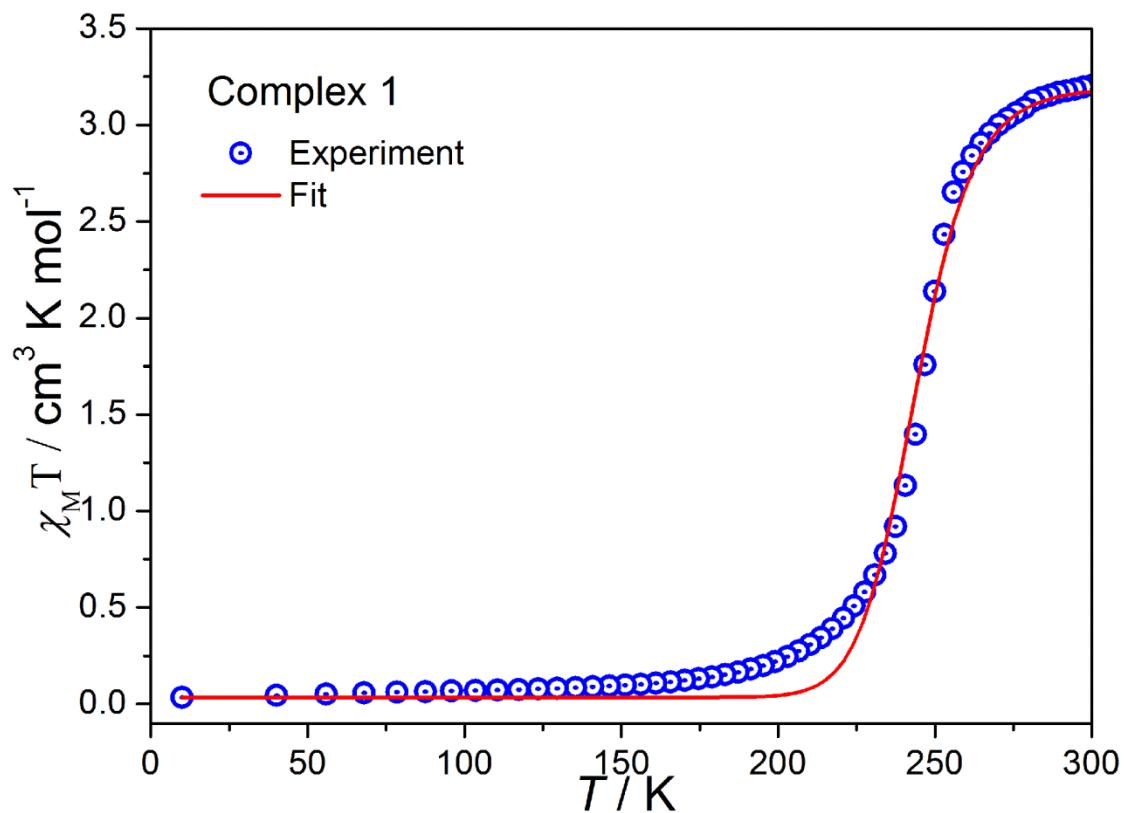
**Figure S15.** Temperature Plot of  $\chi_M T$  vs.  $T$  for  $\mathbf{1}_{\text{NDS}}$  under an applied external magnetic field of 1 kOe. The red solid line corresponds to the domain model
