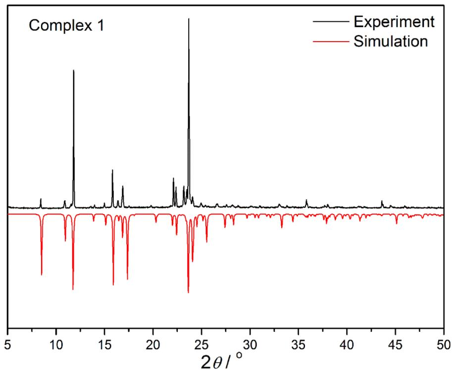
**Figure S1.** Experimental and simulated powder X-ray diffraction patterns for **1<sub>NDS</sub>**.
