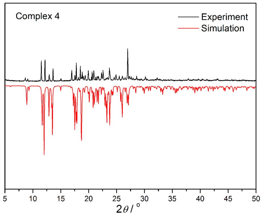
**Figure S4.** Experimental and simulated powder X-ray diffraction patterns for **4<sub>DNDS</sub>**.
