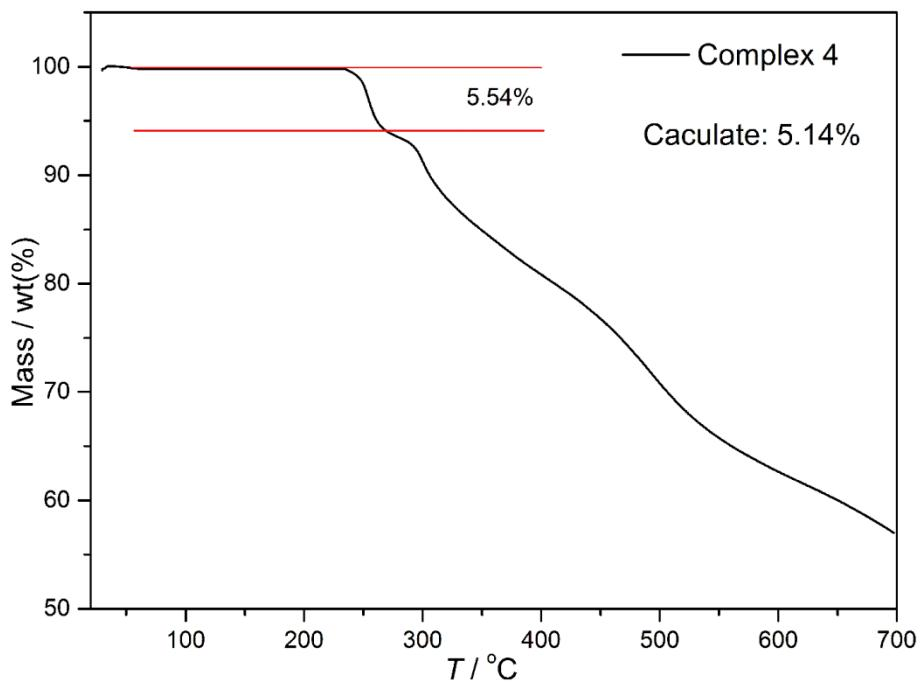
**Figure S8.** TG curve of compound **4<sub>DNDS</sub>** at a rate of  $10 \text{ K}\cdot\text{min}^{-1}$  under at  $\text{N}_2$  atmosphere.
