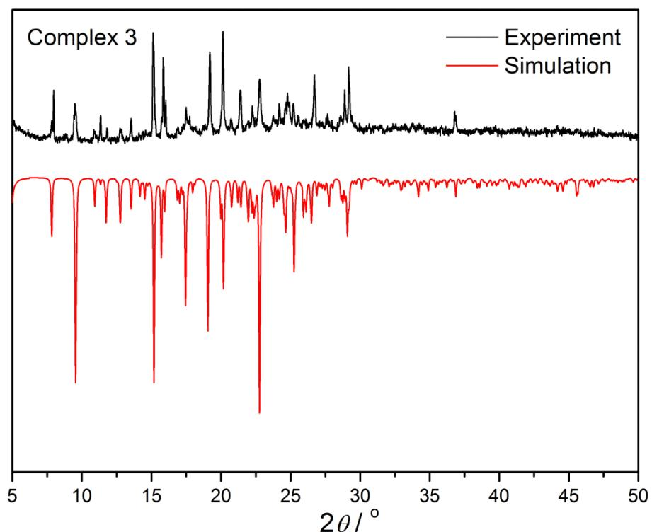
**Figure S3.** Experimental and simulated powder X-ray diffraction patterns for **3<sub>ABDS</sub>**.
