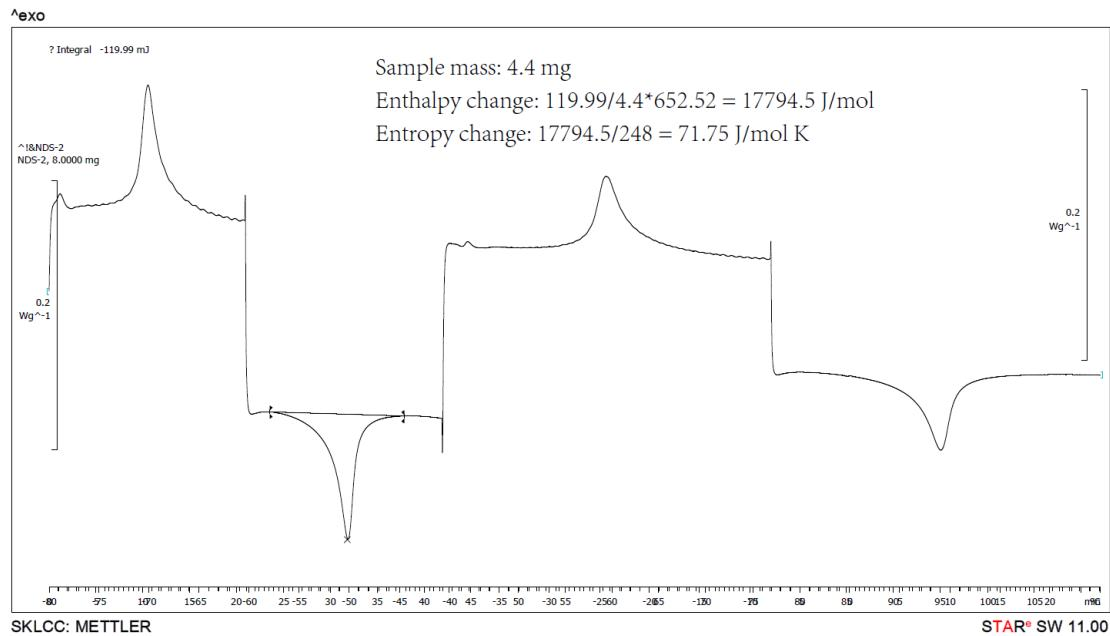
**Figure S14.** DSC data processing of complex **1<sub>NDS</sub>** (the first warming process)
