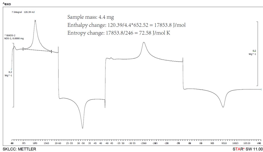
**Figure S13.** DSC data processing of complex **1<sub>NDS</sub>** (the first cooling process)
