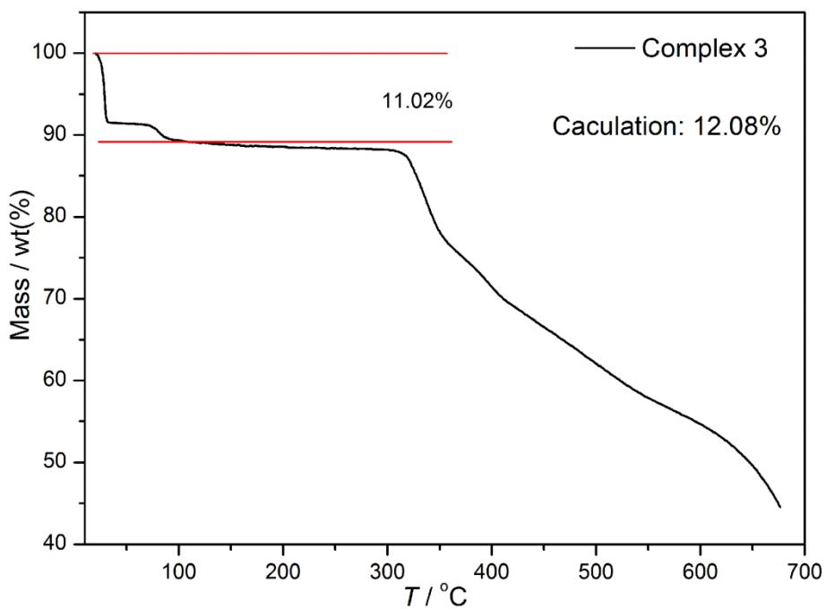
**Figure S7.** TG curve of compound **3<sub>ABDS</sub>** at a rate of  $10 \text{ K}\cdot\text{min}^{-1}$  under at  $\text{N}_2$  atmosphere.
