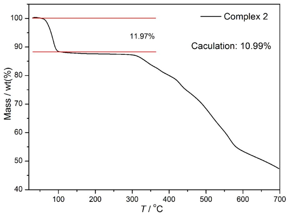
**Figure S6.** TG curve of compound **2<sub>BPDS</sub>** at a rate of  $10 \text{ K}\cdot\text{min}^{-1}$  under at  $\text{N}_2$  atmosphere.
