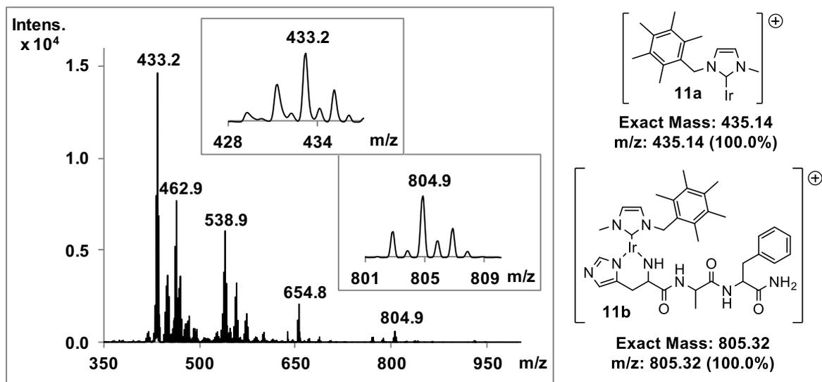
**Supplementary Figure S9:** ESI MS spectrum of the adduct between peptide **6b** and complex **7b** with the respective fragments **11a** and **11b** belonging to the suggested Iridium adduct. In contrast to the adducts of **6c** and **7b**, several other fragments with undefined structures can be seen.
