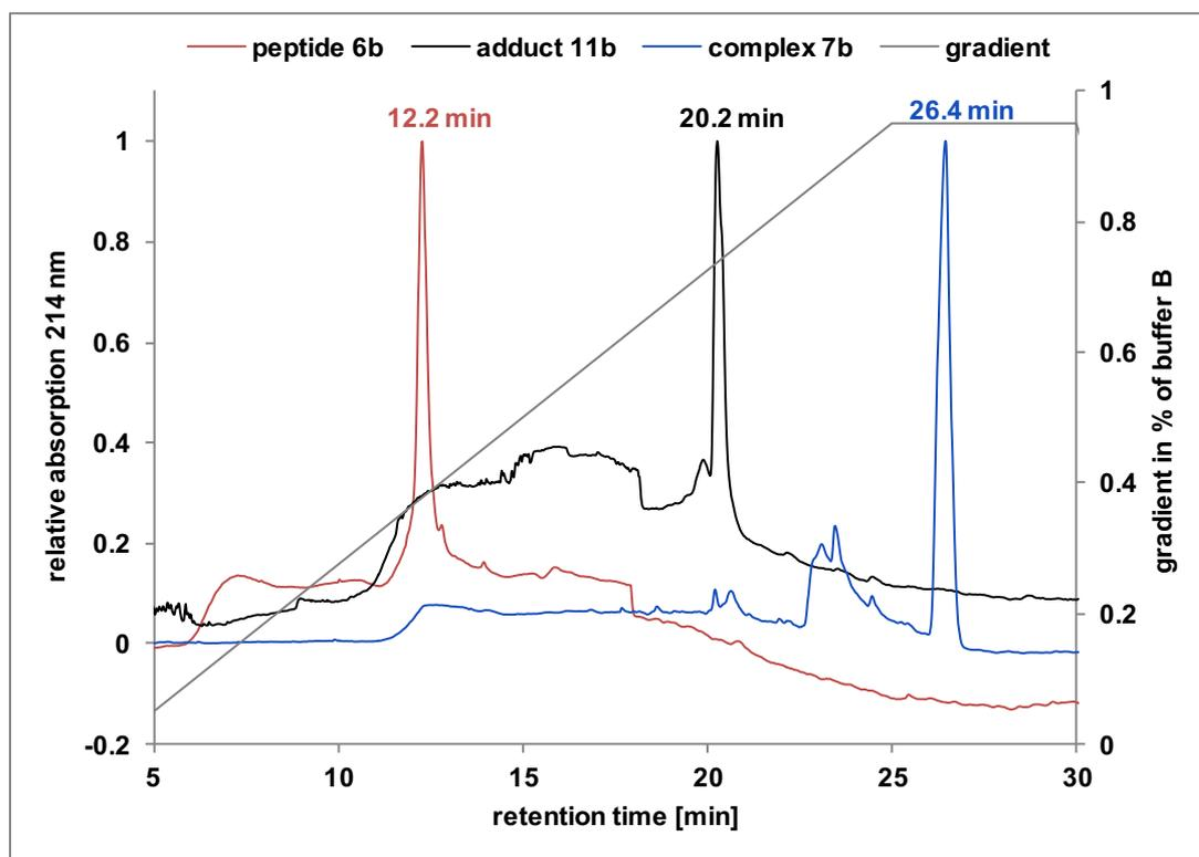
**Supplementary Figure S10:** Analytical HPLC trace of adduct **11b** in comparison to peptide **6b** and complex **7b** (Buffer A: H<sub>2</sub>O with 0.1% TFA, Buffer B: ACN with 0.1% of TFA, Column: Dr. Maisch Reprisil pur C8 250 x 4.6 mm)
