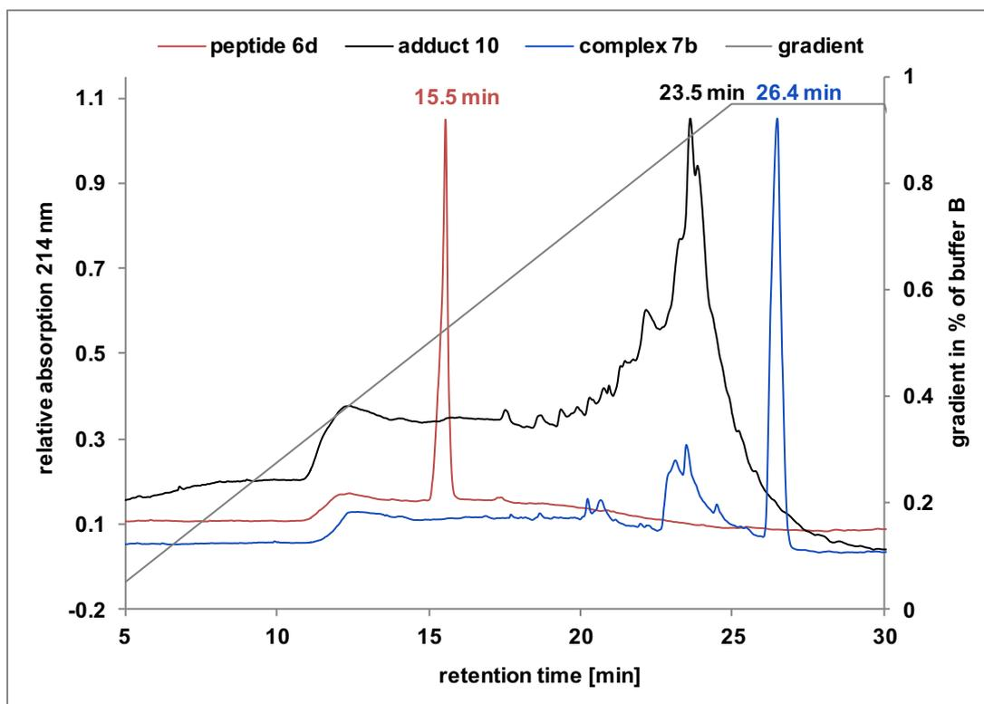
**Supplementary Figure S14:** Analytical HPLC trace of adduct **10a, b, c** or **d** in comparison to peptide **6d** and complex **7b** (Buffer A: H<sub>2</sub>O with 0.1% TFA, Buffer B: ACN with 0.1% of TFA, Column: Dr. Maisch Reprisil pur C8 250 x 4.6 mm)
