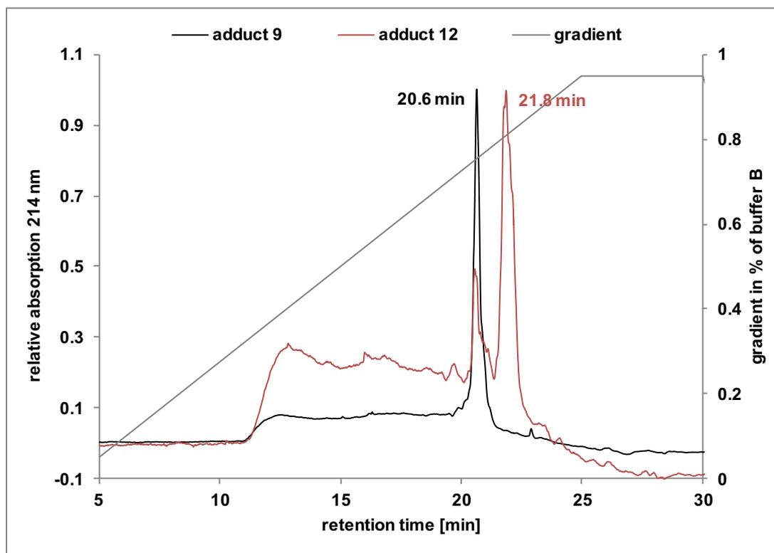
**Supplementary Figure S13:** Analytical HPLC trace of adduct **9a** or **b** in comparison to adduct **12** (Buffer A: H<sub>2</sub>O with 0.1% TFA, Buffer B: ACN with 0.1% of TFA, Column: Dr. Maisch Reprisil pur C8 250 x 4.6 mm)
