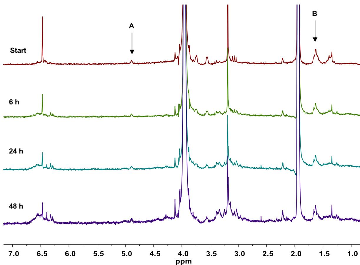
**Supplementary Figure S4:** Time dependent  $^1\text{H}$  NMR spectra of complex **7a** in deuterated PBS with addition of 10% of DMSO. The spectrum shows the signals expected for the compound and the additional signals A and B (marked with an arrow). Over time an overall decrease in peak intensity can be observed for the signals representing complex **7a** while the intensity of the additional signals shows only a minor decrease.
