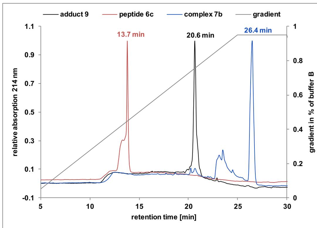
**Supplementary Figure S11:** Analytical HPLC trace of adduct **9a** or **b** in comparison to peptide **6c** and complex **7b** (Buffer A: H<sub>2</sub>O with 0.1% TFA, Buffer B: ACN with 0.1% of TFA, Column: Dr. Maisch Reprisil pur C8 250 x 4.6 mm)
