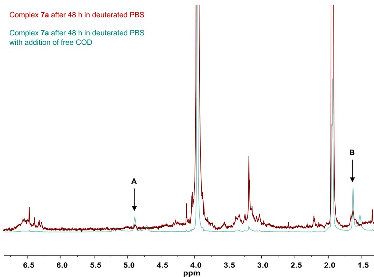
**Supplementary Figure S5:** Overlay of the <sup>1</sup>H NMR spectra of complex **7a** after 48 h in deuterated PBS with addition of 10% of DMSO (red trace) and of the same sample after addition of free COD (green trace). Upon addition of COD the green trace shows an increase in peak intensity of the signals A and B (marked with an arrow) thus clearly identifying them as the COD ligand of the initial complex getting detached in solution.
