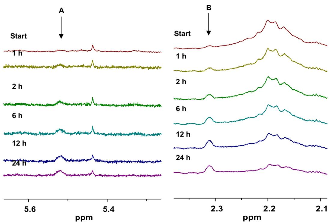
**Supplementary Figure S6:** Upper Part: Change in the overall  $^1\text{H}$  NMR of complex **7c** over time in deuterated ACN, which was used as an internal standard, after addition of water. The new signals A and
