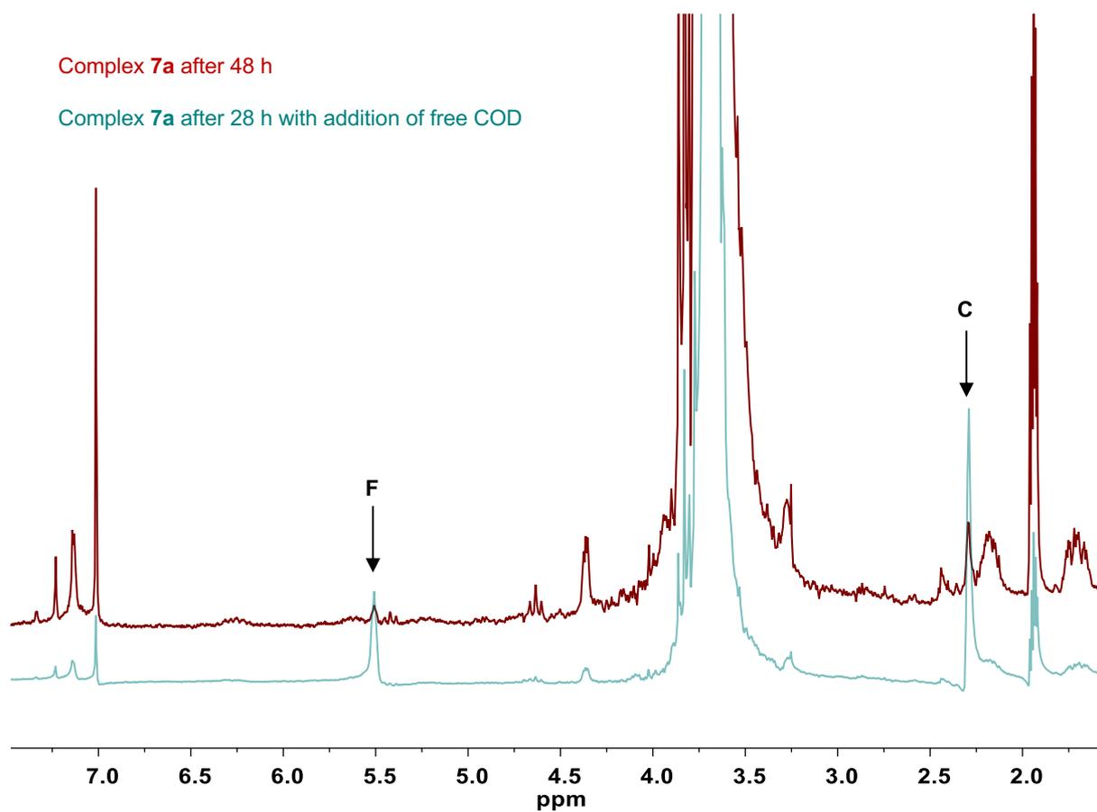
**Supplementary Figure S2:** Overlay of the <sup>1</sup>H NMR spectra of complex **7a** after 48 h (red trace) and of the same sample after addition of free COD (green trace). Upon addition of COD the green trace shows an increase in peak intensity of the signals F and C (marked with an arrow) thus clearly identifying them as the COD ligand of the initial complex getting detached in solution.
