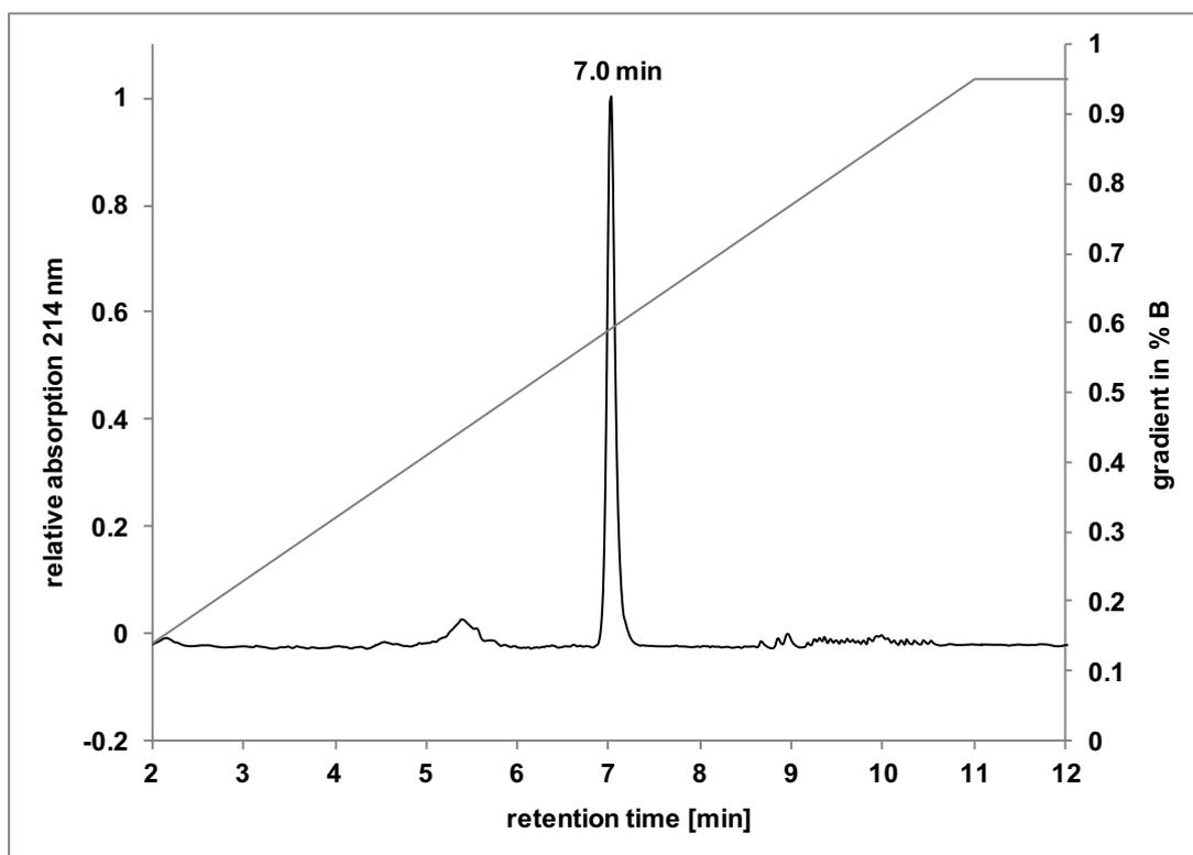
**Supplementary Figure S31:** Analytical HPLC trace of peptide 6a (Buffer A: H<sub>2</sub>O with 0.1% TFA, Buffer B: ACN with 0.1% of TFA, Column: EC 125/4 Nucleodur C18 Pyramid 5 $\mu$ m)
