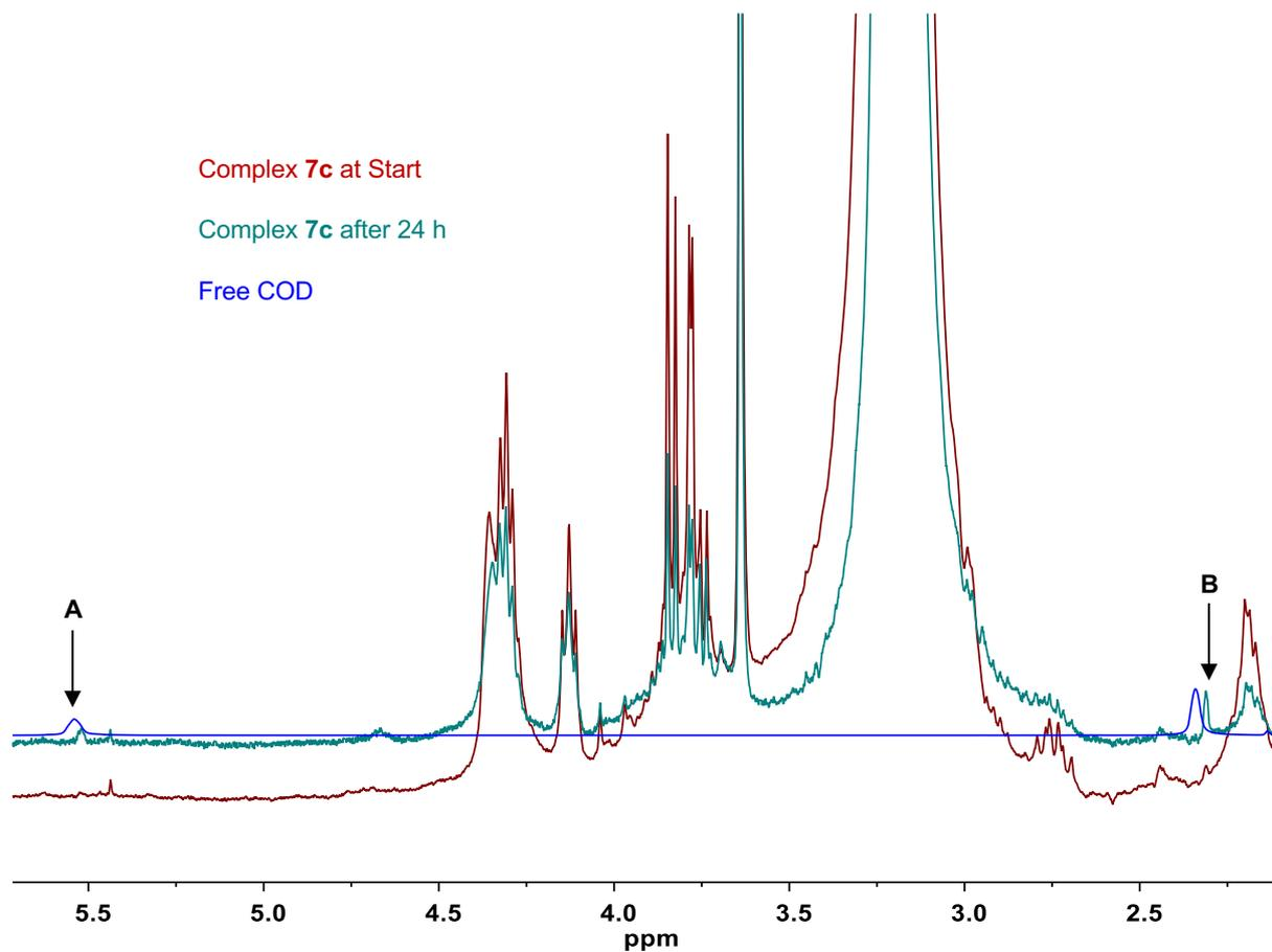
**Supplementary Figure S7:** Overlay of the <sup>1</sup>H NMR spectra of complex **7c** at the beginning of the experiment (red trace), after 24 h (green trace) and of free COD in deuterated acetonitrile (blue trace). The newly arising signals A and B (marked with an arrow) show a nearly perfect overlay with free COD, identifying them as the COD ligand of the initial complex getting detached in solution.
