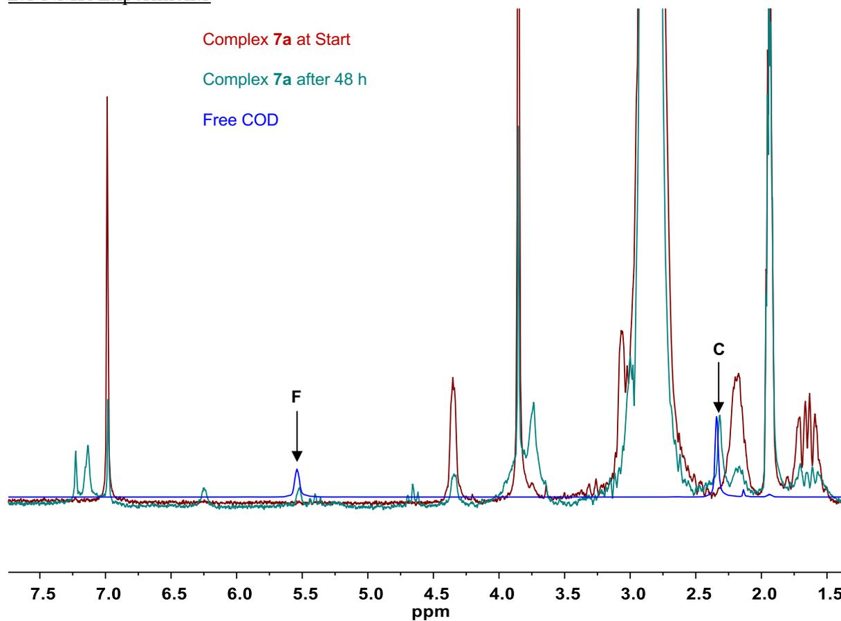
**Supplementary Figure S1:** Overlay of the <sup>1</sup>H NMR spectra of complex **7a** at the beginning of the experiment (red trace), after 48 h (green trace) and of free COD (blue trace) in deuterated acetonitrile. The red and green traces nicely illustrate the overall decrease in peak intensity of the initial complex over time. The newly arising signals F and C (marked with an arrow) are closest to the signals of free COD
